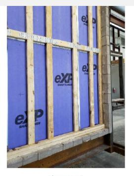
Photo No. 5 Unexposed side of Test Assembly
