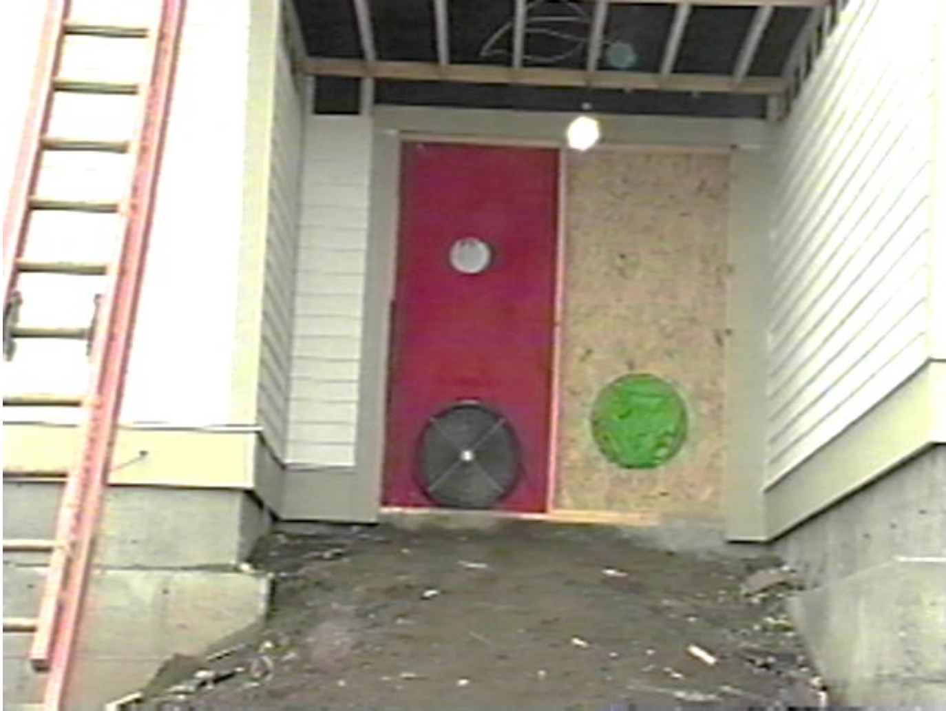
Blower door setup for pressurized theatrical fog (daylight) and depressurized infrared imaging (nighttime)
