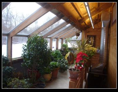
• A blower moves air carrying excess solar heat from the greenhouse to water storage in the Thermomass basement below
