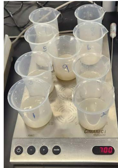
Crush and soak– How much chloride does it release?
