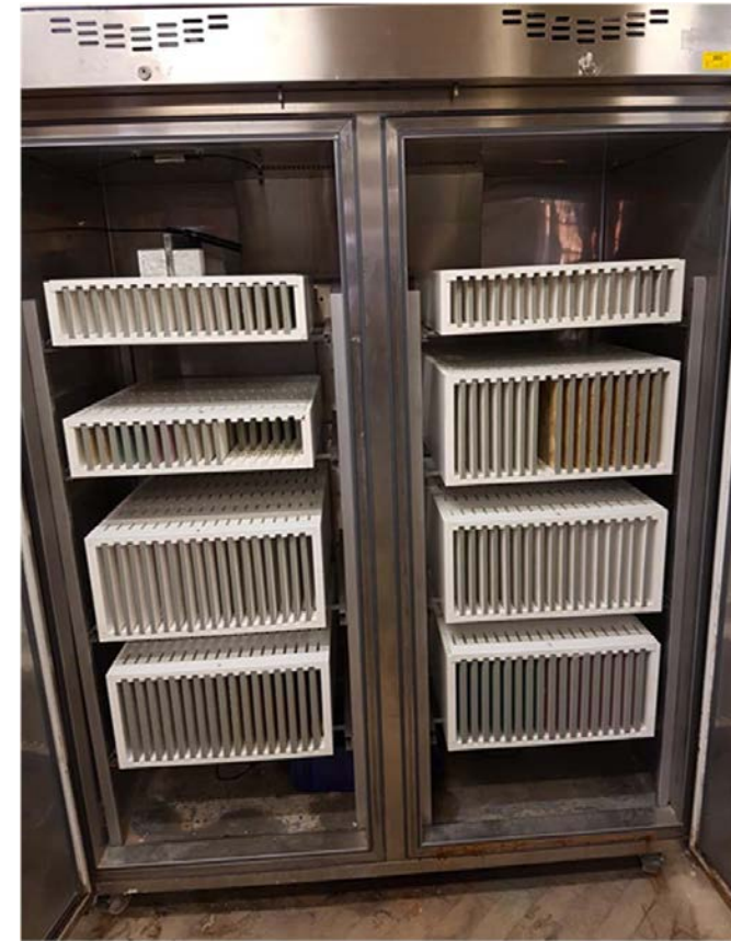
Australian research lab tests MgO samples for > 2 years at high RH
