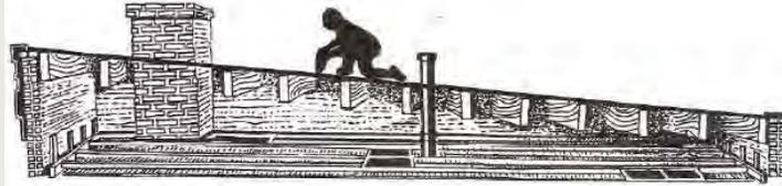
Inspect for roof leaks, and weak ceilings. Note bypass locations from below (duct chases, closets, ceiling height changes, etc.). Cut an access hole big enough for a person but small enough for a roof vent.
