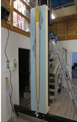
NESEA BE14-Cladding Movement over Exterior Insulation © buildingscience.com 22
