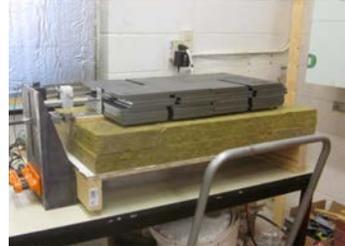
NESEA BE14-Cladding Movement over Exterior Insulation © buildingscience.com 18
