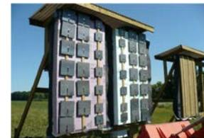
NESEA BE14-Cladding Movement over Exterior Insulation © buildingscience.com 8
