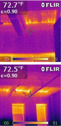
Can't rely on masonry alone to be an air barrier
