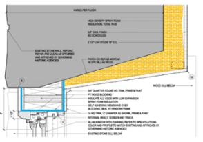
Minimum ~R-5 for thermal comfort (radiant surface temperatures)
