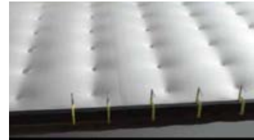
Photo 1. Wind uplift of a membrane with fasteners arranged in a grid pattern.
