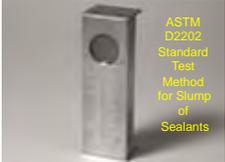
ASTM D2202 Standard Test Method for Slump of Sealants
