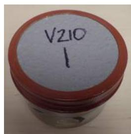
Improved lid with powder-coated corrosion proof finish & improved epoxy seal to keep water out of gap & consistent measurement
