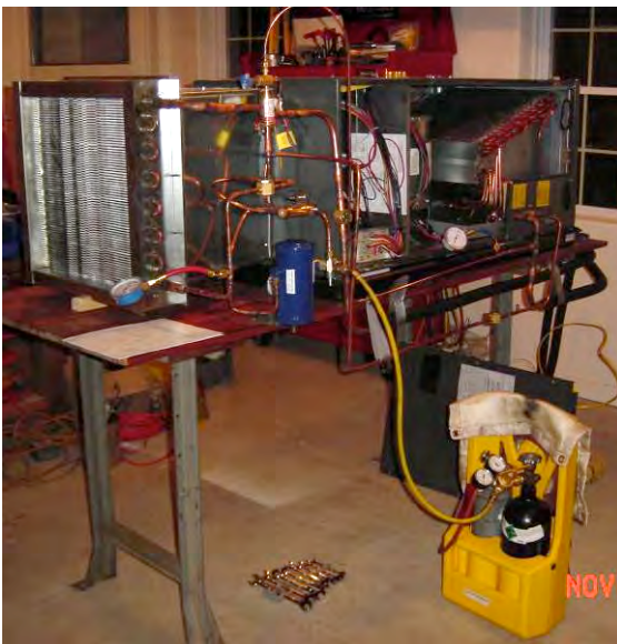
Figure 12: System pressure tested with dry nitrogen
