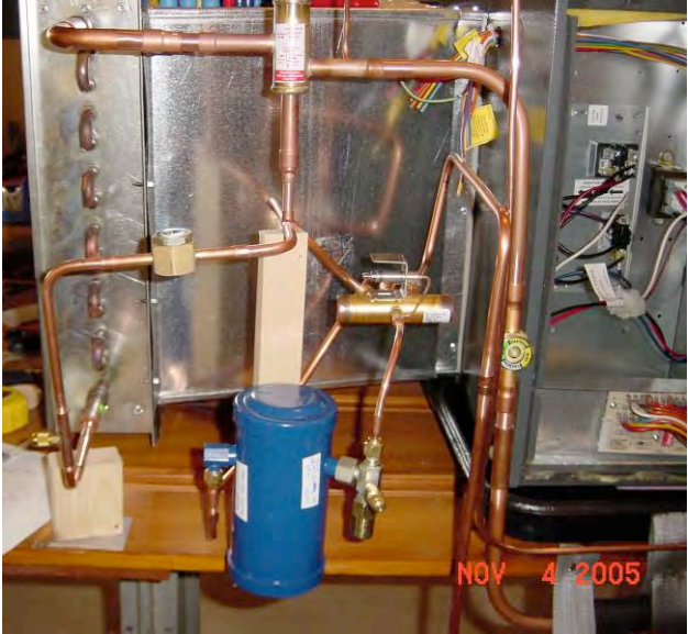
Figure 10: Add-on dehumidifier components fitted (from left to right: cased condenser/reheat coil, 3-way diverting valve with suction bleed, receiver, and reversing valve (required only for heat pump heating operation))
