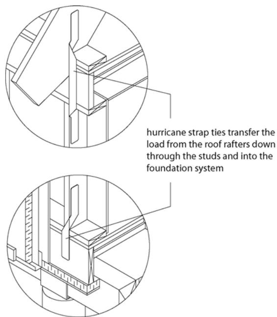
**Figure 3: Hurricane ties used to create a load path through the structure**
