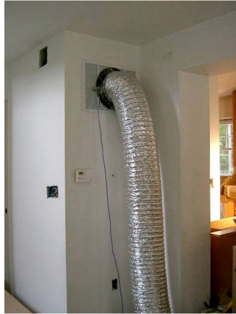
Figure 1.33: Duct Blaster® testing
