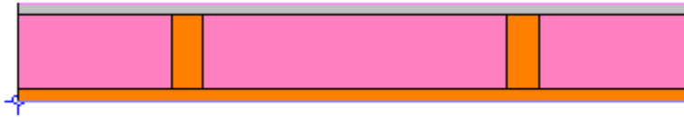
Figure 6 : Typical framing 16" o.c. - 9% framing factor
