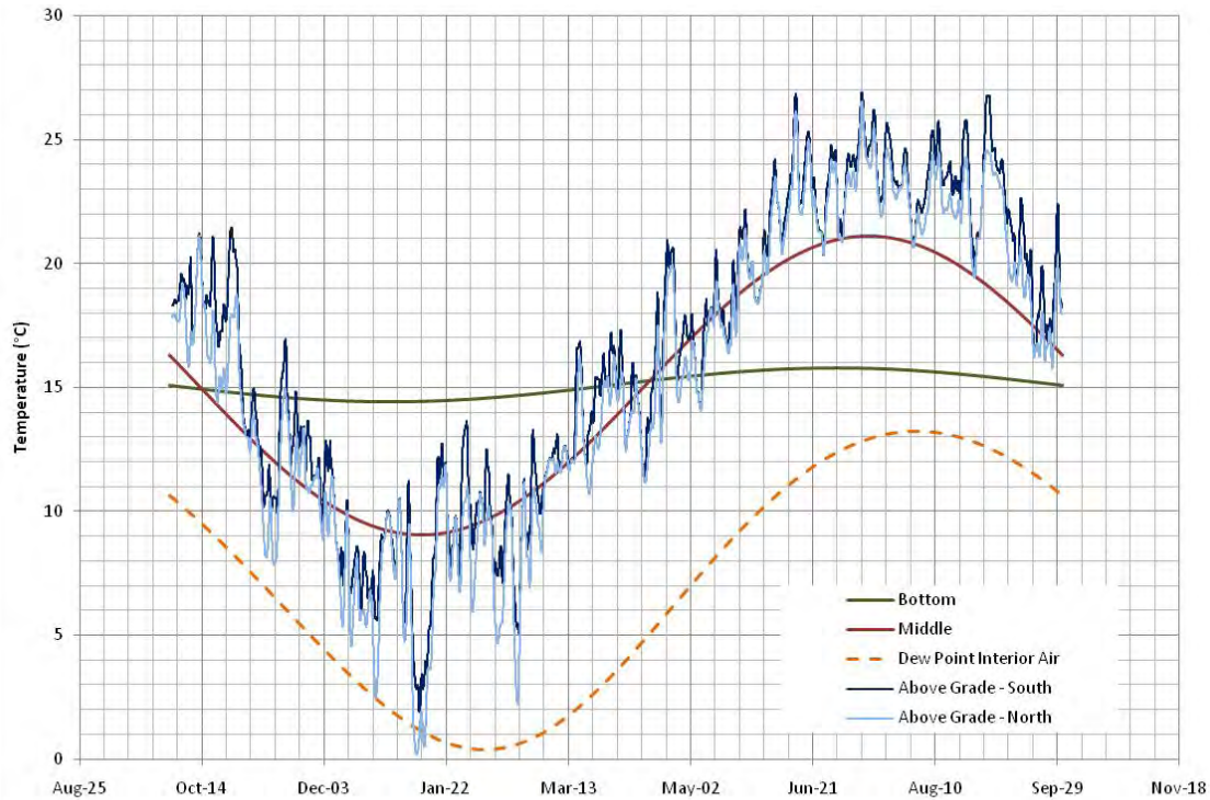
Figure 10 : Condensation Potential for Interior air on the Surface of the Concrete Foundation Wall
