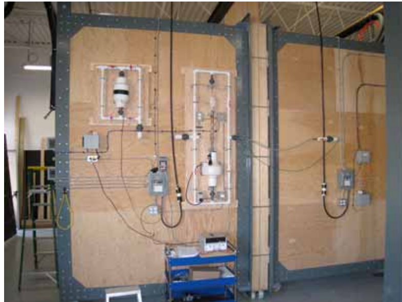
Figure 2: Precision Calibrated Hot Box
