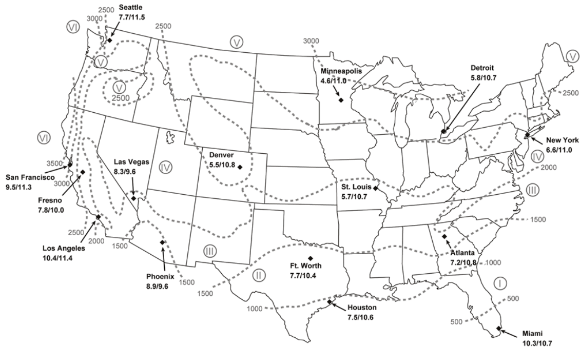
Figure 11: Effect of climate on HSPF and SEER (Fairey et al. 2004)
