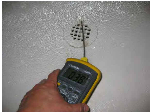
Figure 18: Handheld thermocouple reader, for hot water measurements (drain water T shown)
