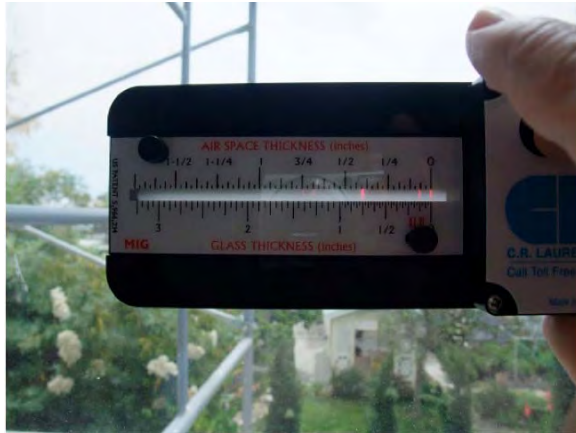
Figure 10.3.7: Laser glass thickness meter, indicating double glazing + suspended film
