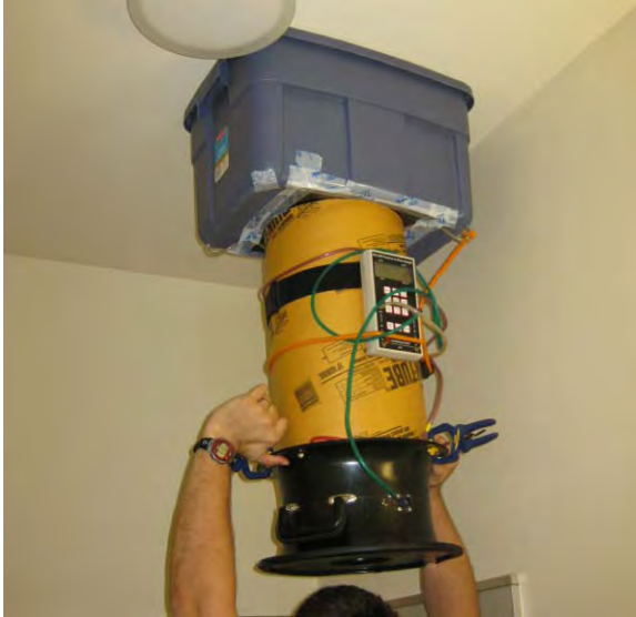
Figure 5: Duct blaster used as a powered capture hood
