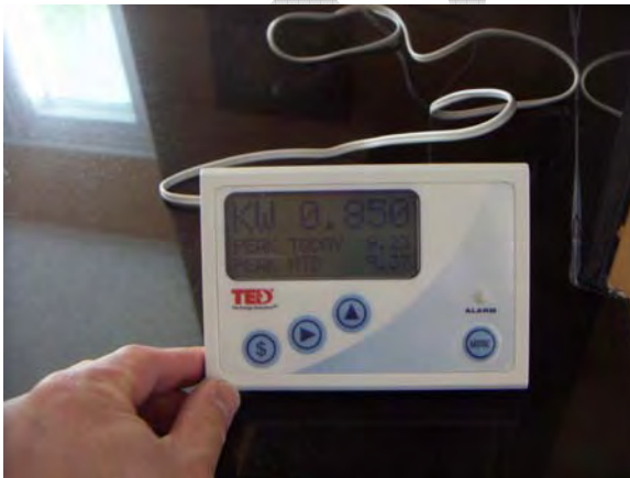
Figure 18: TED (The Energy Detective) electrical feedback monitor
