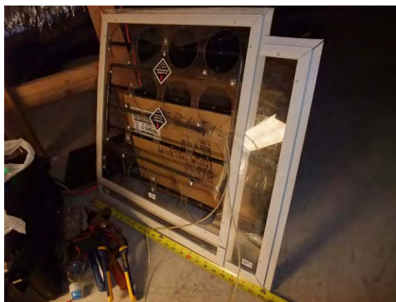
Figure 8: Energy Conservatory TrueFlow filter slot flow measurement plate
