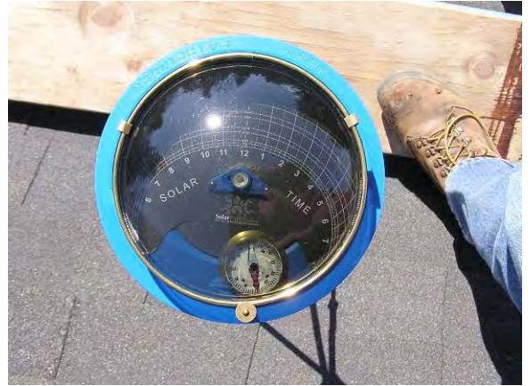
Figure 2.27: Solar Pathfinder™ representation of the relatively unobstructed exposure of the South-facing roof
