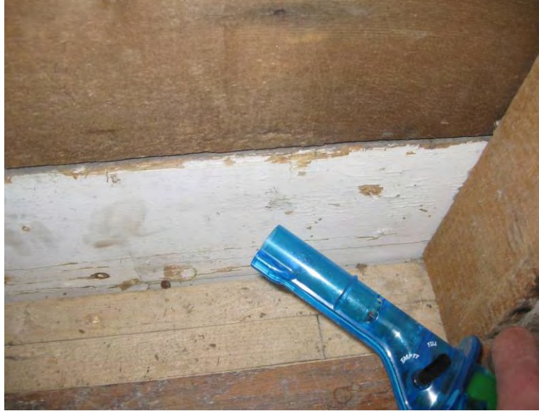
Figure 17 - air movement observed at sill
