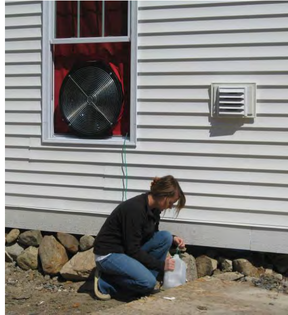
Figure 7 - blower door from exterior
