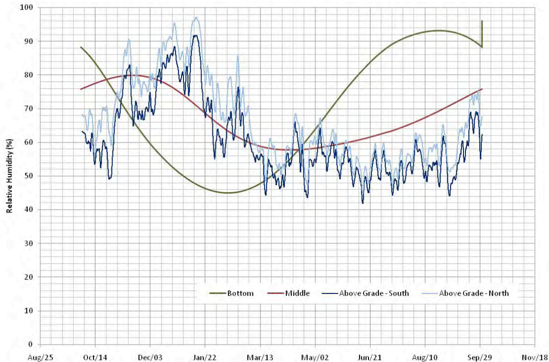
Figure 25 : Predicted Relative Humidity at the interior Surface of the XPS for Case 8
