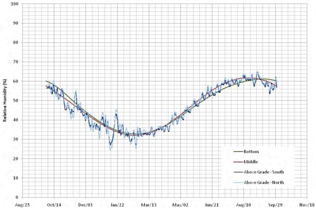
Figure 27 : Predicted Relative Humidity at the Exterior Surface of Gypsum Board for Case 8
