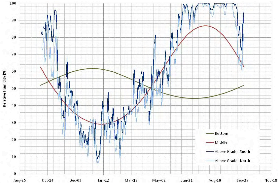
Figure 17 : Predicted Relative Humidity at the Surface of the Polyethylene Vapor Barrier for Case 3
