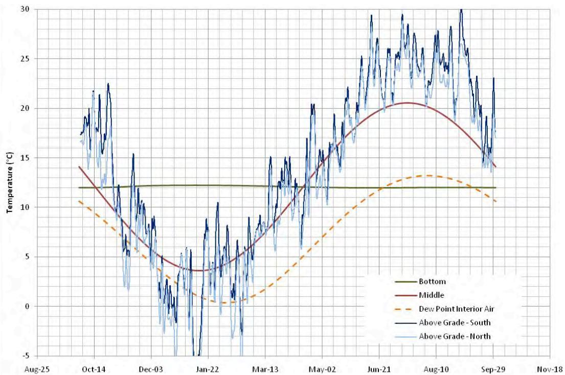
Figure 19 : Interior Air Leakage Condensation Potential for Case 4
