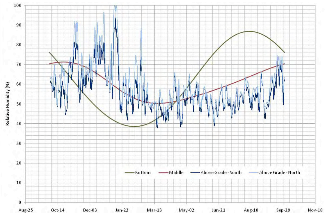
Figure 13 : Predicted RH at the Interior Surface of the Concrete Foundation Wall for Case 1
