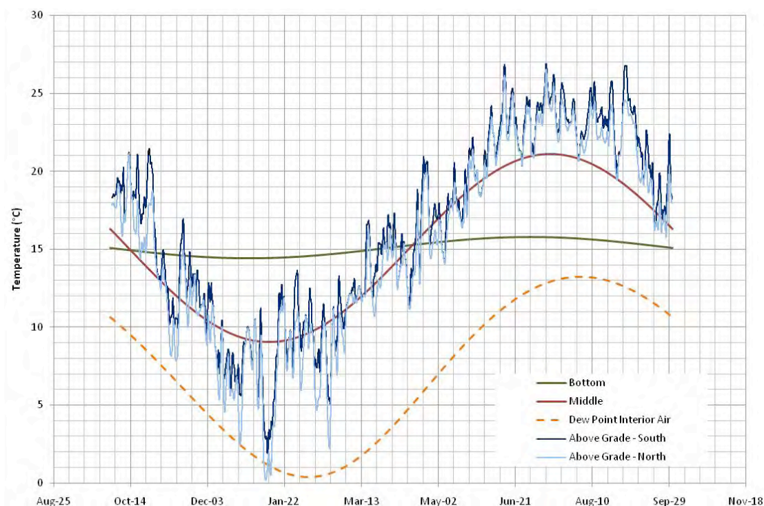
Figure 14 : Condensation Potential for Interior air on the Surface of the Concrete Foundation Wall
