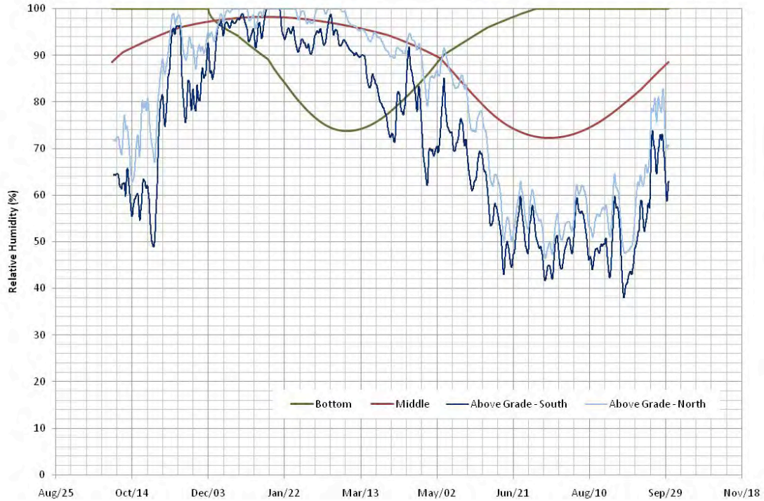
Figure 23 : Predicted Relative Humidity at the Interior Surface of the Foundation Wall of Open Cell Spray Foam Case 7
