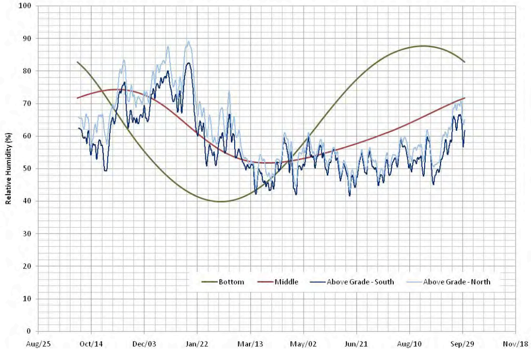
Figure 31 : Predicted Relative Humidity at the interior Surface of the PIC for Case 15
