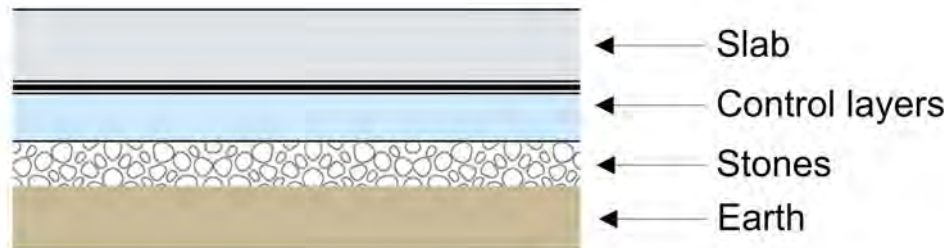
Figure 18: The optimal slab on earth design is both well established and affordable.
