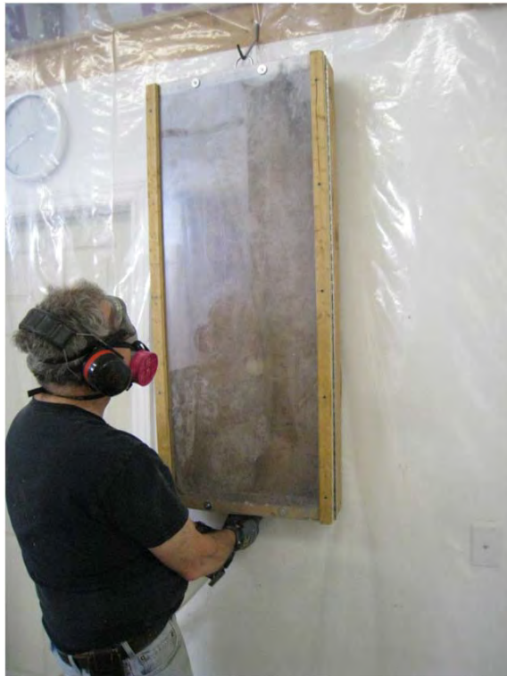
Figure 47 – Dense-packing the calibration box
