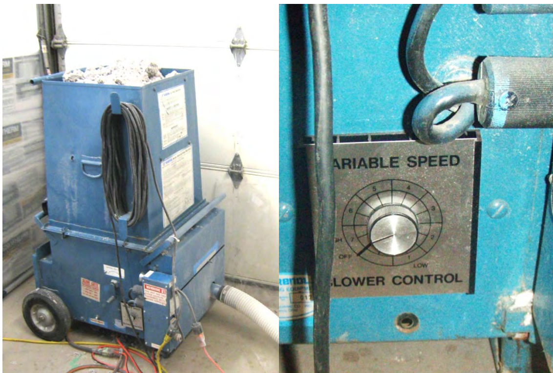
Figure 17 – Krendl 450A All-Fiber Machine (left) with variable speed blower control (right)
