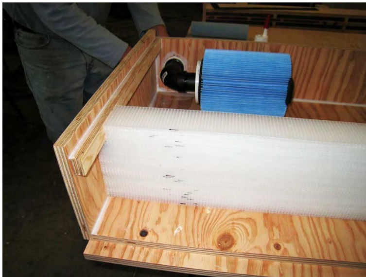
Figure 28 – Manifold shown open during construction (flow straightener and air filter visible)
