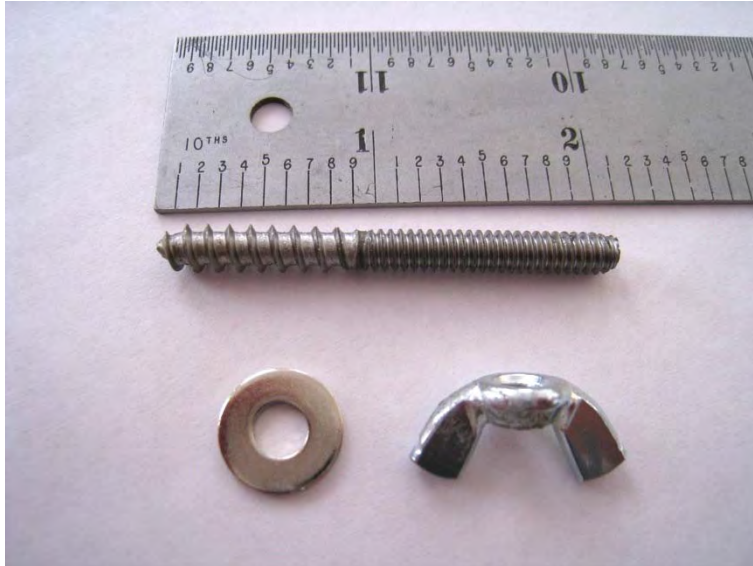
Figure 14 – Hanger bolt, washer & wing nut for attaching back panel to front panel frame
