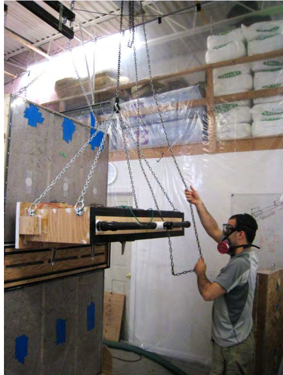
Figure 53 – Lowering the air pressure manifold into position
