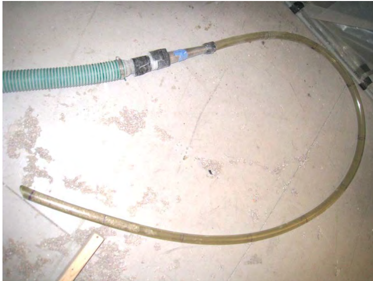
Figure 20 – 1/14 in. inside dia. smooth-walled PVC insertion tube
