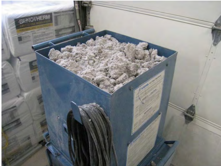
Figure 42 – Fiber-moving machine hopper filled with insulation material
