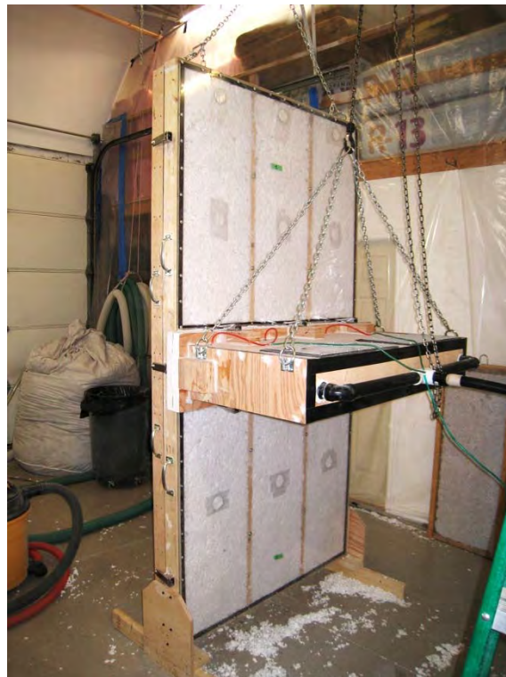
Figure 26 – Test specimen prepared and connected to manifold for airflow testing
