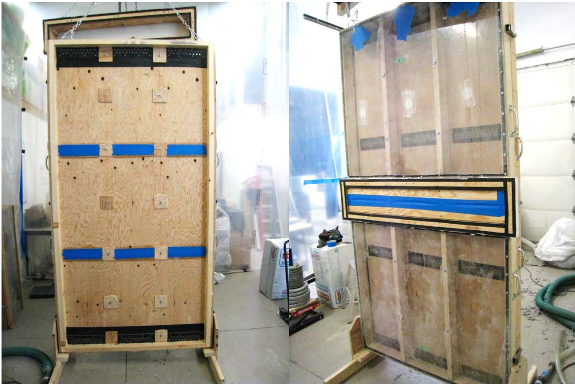
Figure 49 – Seal test wall assembly to ‘representative field condition’
