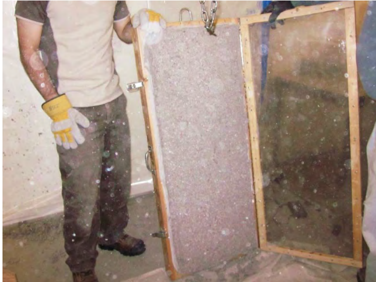
Figure 23 – Calibration box filled with insulation and opened for inspection and cleaning
