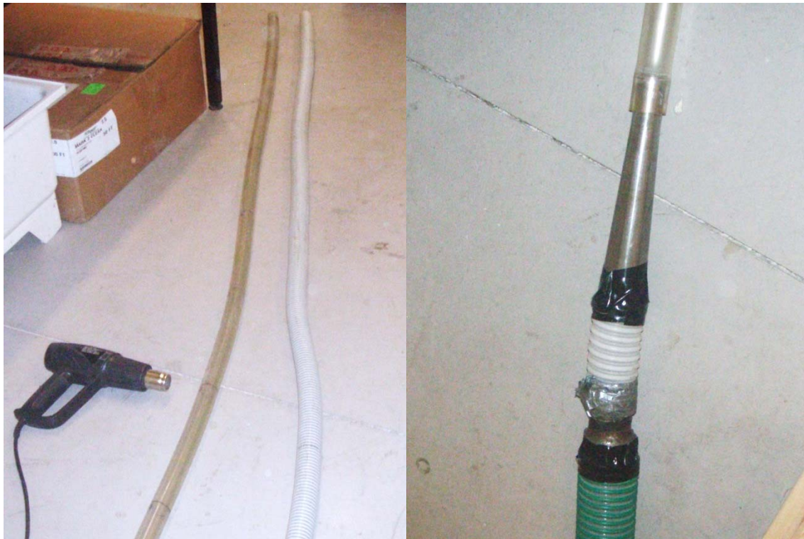
Figure 21 – Removing insertion tube memory (left) and transitioning to the 2-1/2” hose (right)
