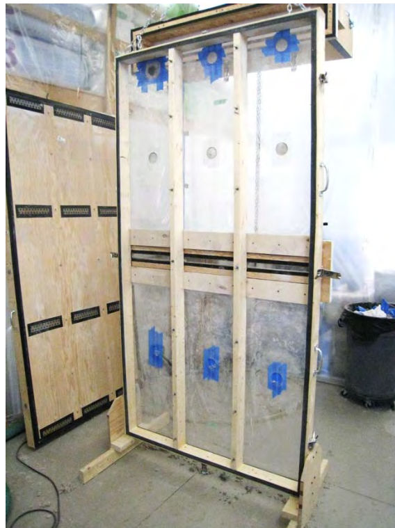
Figure 2 – Install Holes in Front Panel as seen from back (with Back Panel removed)
