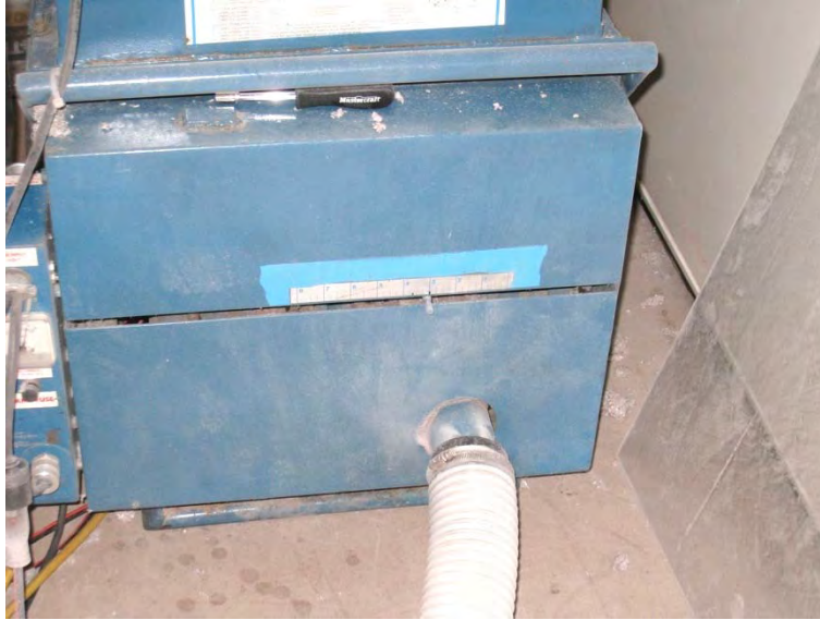
Figure 18 – 3” dia. ribbed hose attached to outlet of the Krendl 450A
