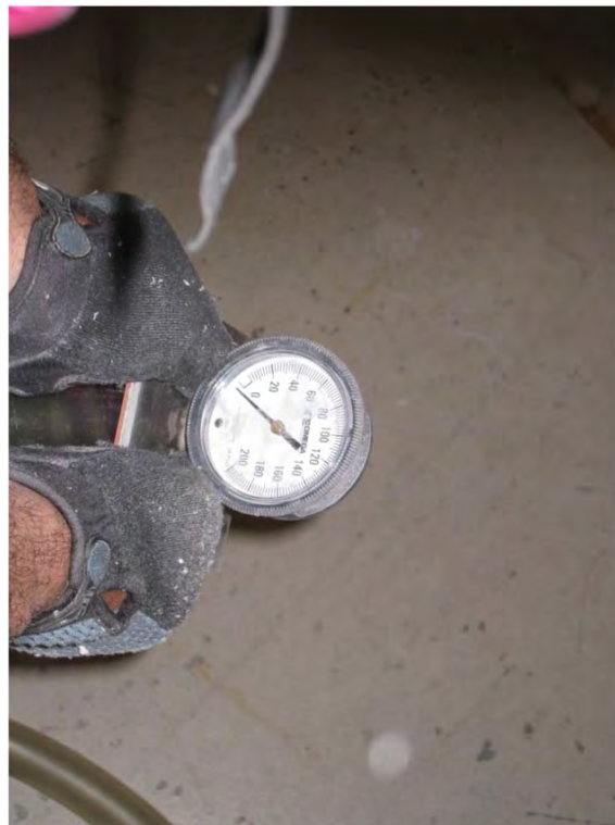
Figure 45 – Measuring fiber-moving machine blower pressure
