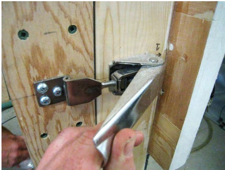
Figure 60 – Releasing the latches (qty of 6) on the sides of the test wall assembly
