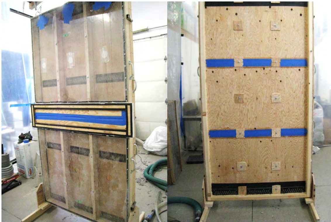
Figure 1 – Empty Test Wall Assembly as seen from front (left image) and back (right image)
