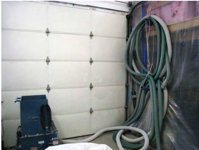
Figure 19 – 50 ft. of 3” dia. (white) & 100 ft. of 2-1/2” dia. (green) hose suspended in a ‘figure 8’ An 8 ft. long 1-1/4 in. dia. smooth-wall PVC tube (e.g. J&R products ST-125), visible in Figure 20, was used as the insertion tube. The tube was heated, as illustrated in the left image of to
