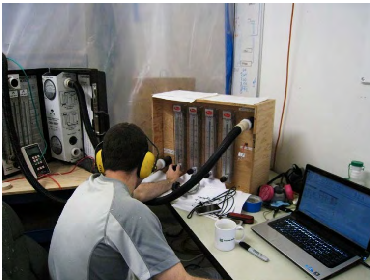
Figure 58 – Checking the background air leakage
