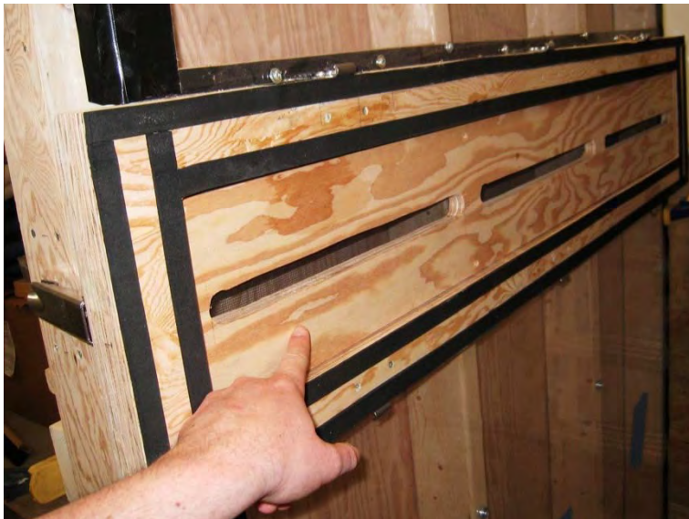
Figure 5 – Exit orifice plate with 1" wide slot opening
