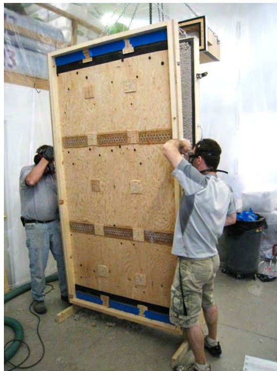
Figure 62 – Removing the back panel from the test wall assembly
