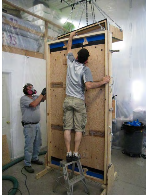
Figure 61 – Releasing the latches at the top & bottom (1 each) of the test wall assembly
