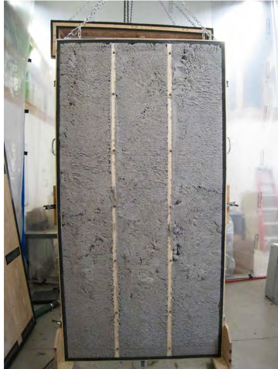
Figure 63 – Inspecting & documenting the back of the dense-packed insulation
