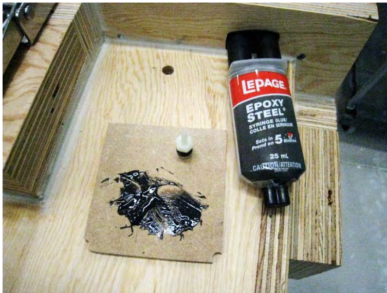
Figure 31 – Installing a pressure tap (typ. of 4) in top of manifold
