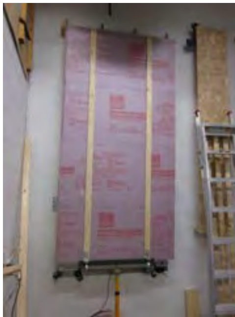
Figure 4. Short-term deflection test panel
