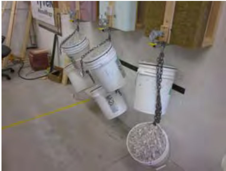
Figure 7. Dead weights attached to bottom edge of furring strips
