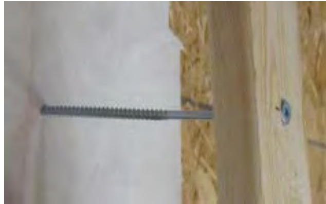
Figure 3. Example of fastener yielding in Mode IV
