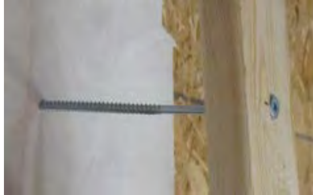
Figure 3. Example of fastener yielding in Mode IV
