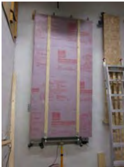
Figure 4. Short-term deflection test panel
