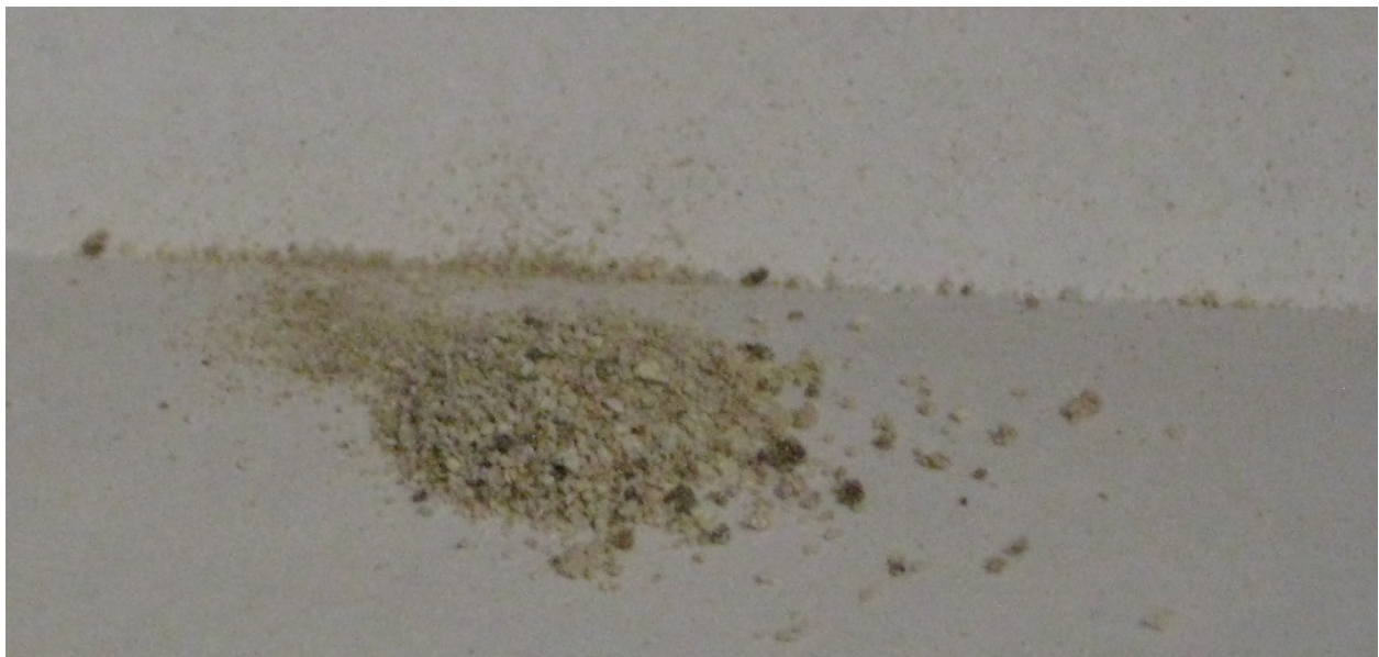
Figure 10(b). Dried mineral precipitate from inlet strainer – mostly calcium carbonate
