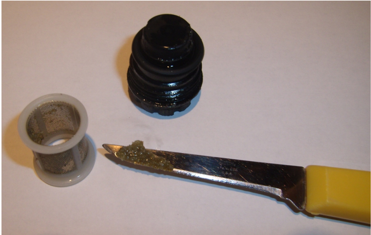
Figure 10(a). Mineral precipitate removed from clogged inlet strainer
