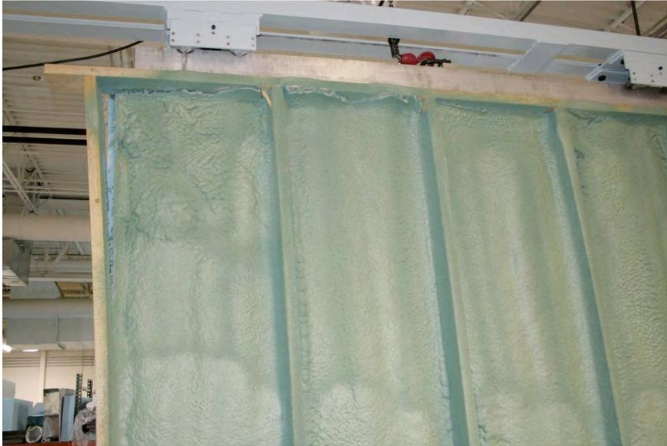
**Figure 28. ccSPF tear propagation**
