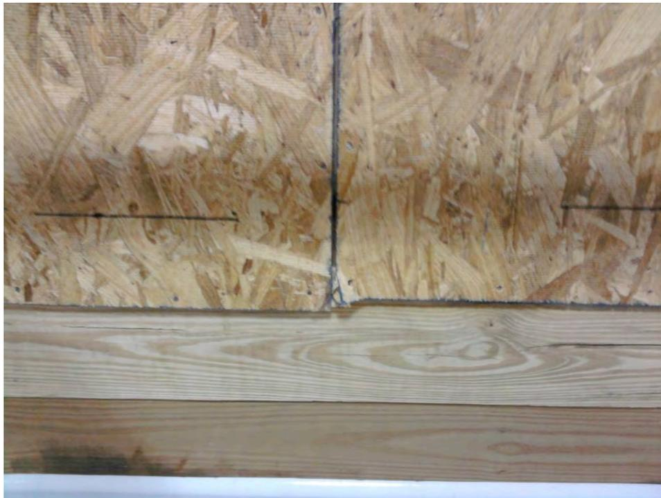
**Figure 19. OSB failure at fastener**
