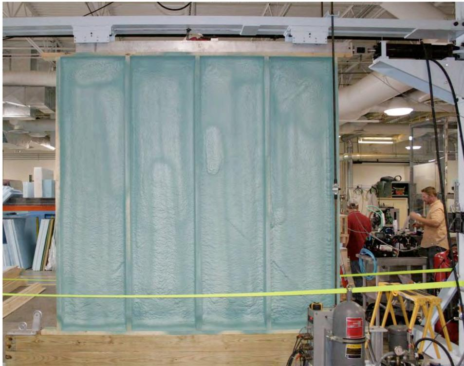
**Figure 25. Structural testing wall 2 installed in apparatus**
