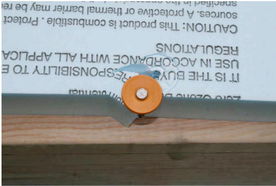
**Figure 23. Nail pulling through XPS**
