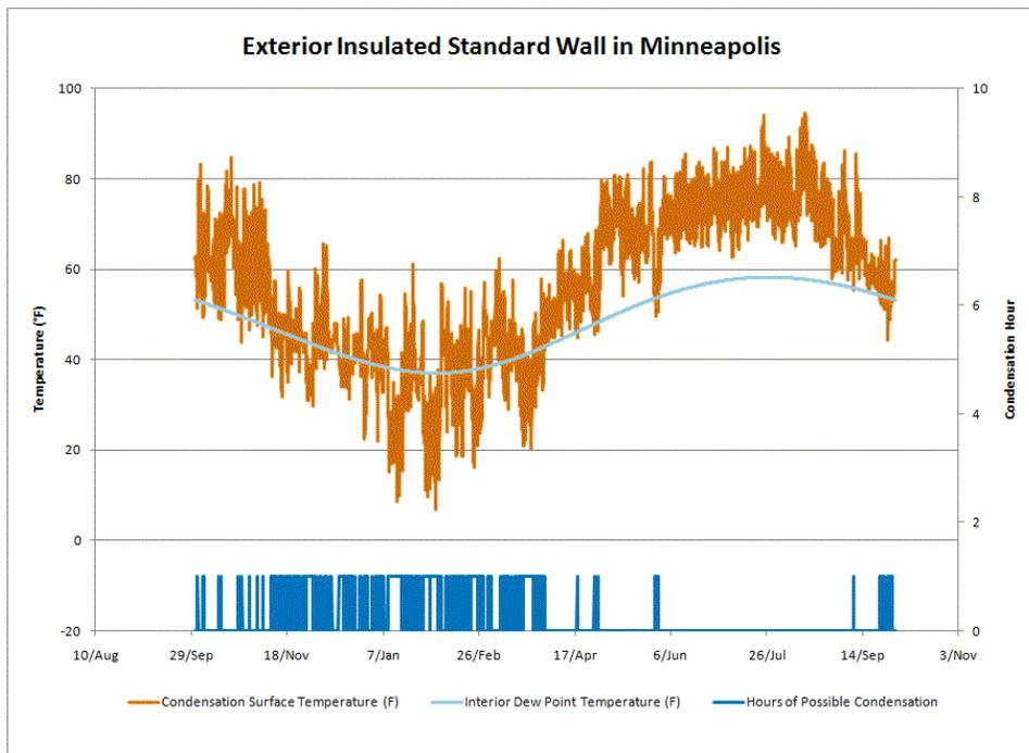
Figure 6 - Exterior insulated standard wall in Minneapolis
