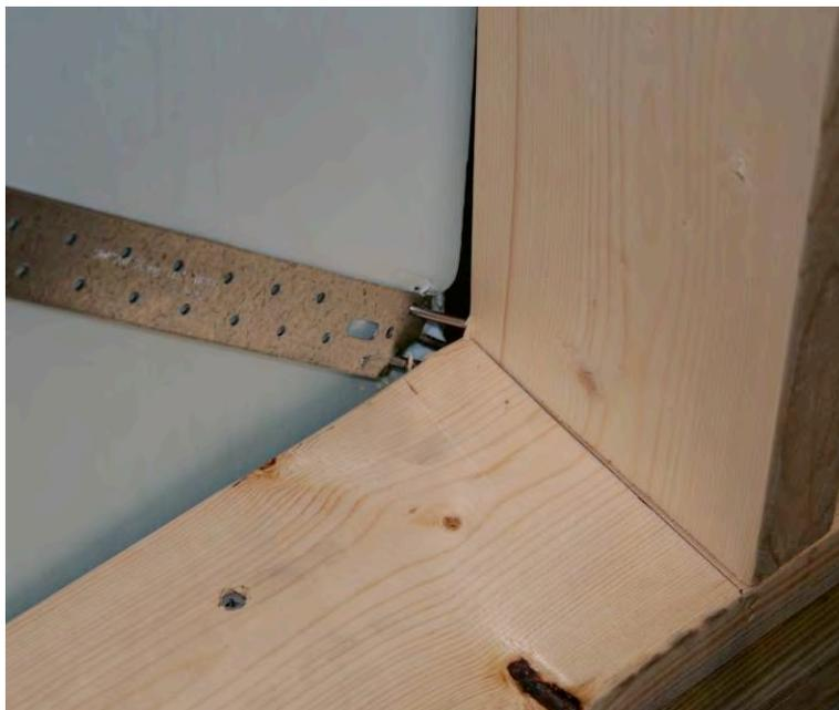
Figure 22. Metal strap nail pullout
