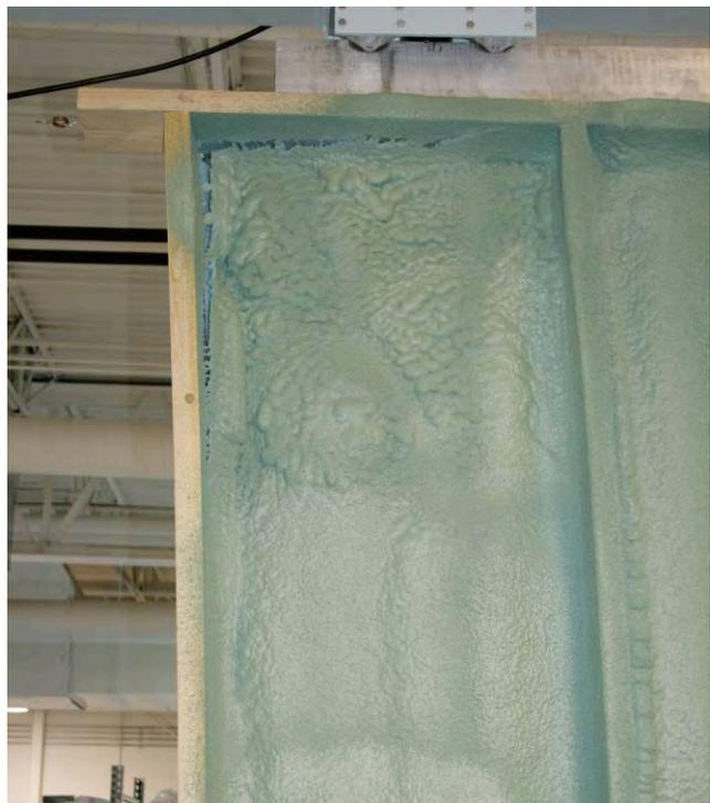
Figure 27. Stud flexure and ccSPF tearing
