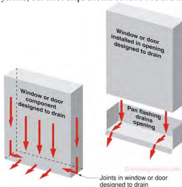
**Figure 1 - Pan Flashing to Drain Openings**
