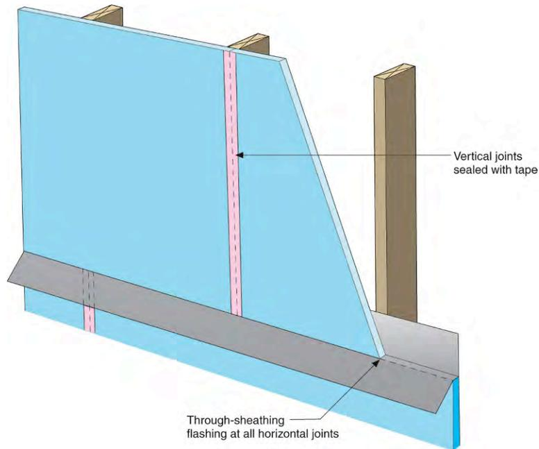
**Figure 13 – Example Through Drainage Plane Z-Flashing**
