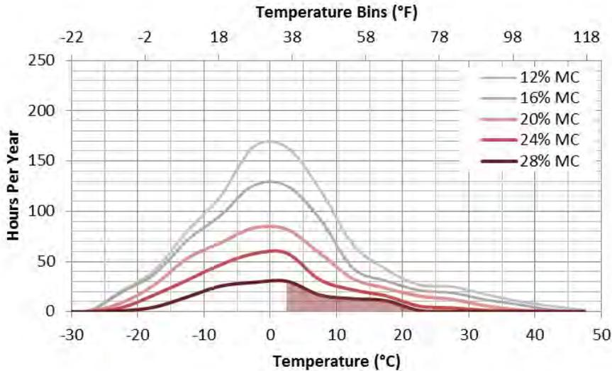
**Figure 17 – Biodegradation Risk Plot for North-facing Common Retrofit Roof with Wintertime Indoor @ 40% RH (no air leaks)**
