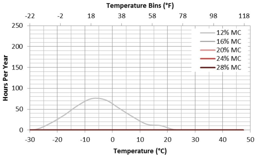
**Figure 18 – Biodegradation Risk Plot for Exterior Insulated Retrofit Roof with Wintertime Indoor @ 40%RH (no air leaks)**
