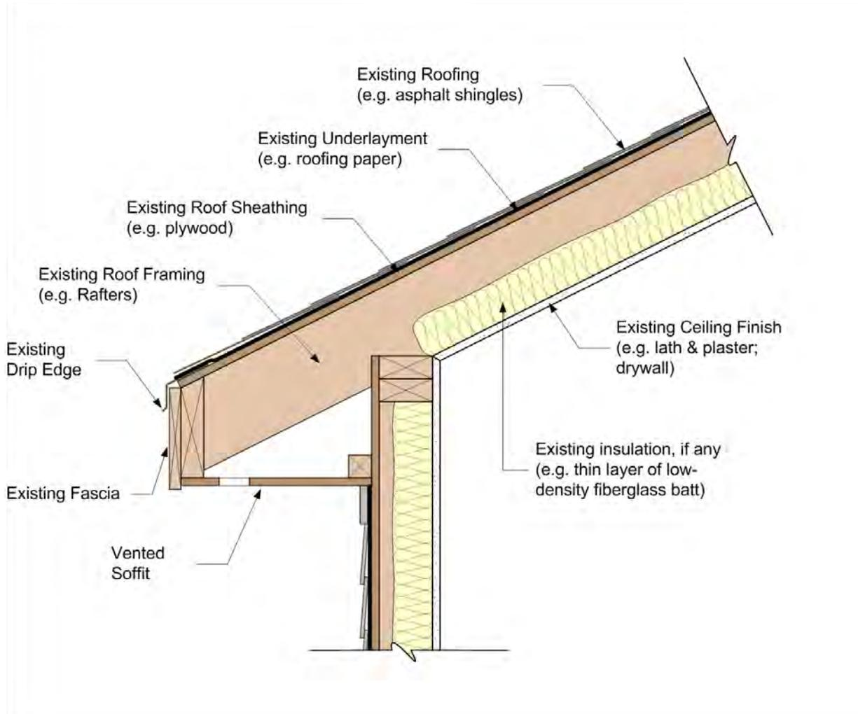
**Figure 3 – Example of Pre-Retrofit Assembly for Hygrothermal Simulations**
