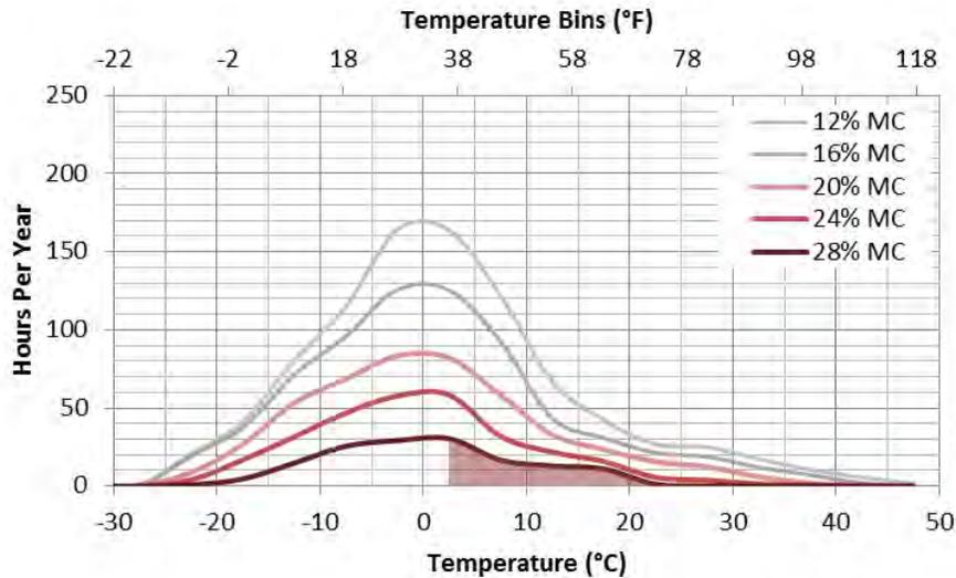
**Figure 14 – Biodegradation Risk Plot for North-facing Roof with Wintertime Indoor @ 40%RH (no air leaks)**
