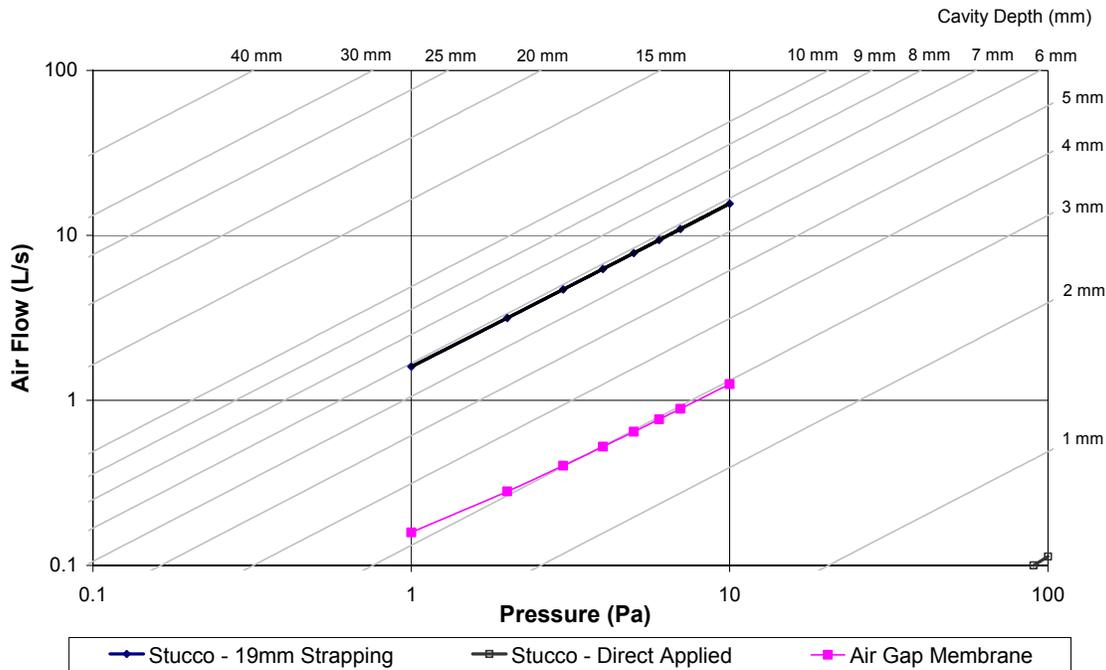
**Figure 23 – Ventilation Gap Flow Rates and Equivalent Cavity Depths (Smegal, 2006)**
