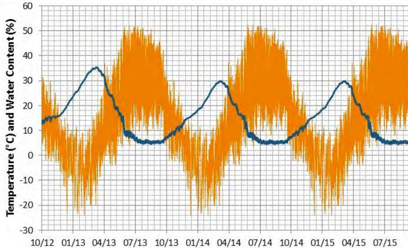
**Figure 6 – Predicted Temperature & MC at Inside of Sheathing on North-facing Common Retrofit Assembly with Wintertime Indoor 40%RH**
