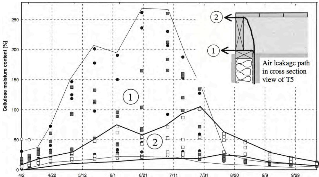
Moisture content in the cellulose insulation of T5 and L5T3 assemblies with short air leakage flow path. The bold-lined zone groups the cellulose specimens under the deck, corresponding to an airflow path 250-400 mm (10-16 in.) long. The fine-lined zone groups cellulose specimens at the bottom of the assembly, corresponding to an air leakage flow path about 100 mm (4 in.) long through the insulation. The inset gives the position of the air paths through a cross-sectional view of the assembly.
