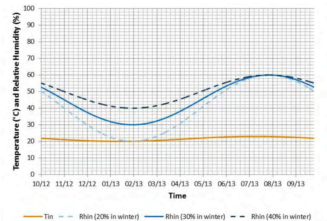
**Figure 2 – Indoor Temperature and RH Assumed for Hygrothermal Simulations**
