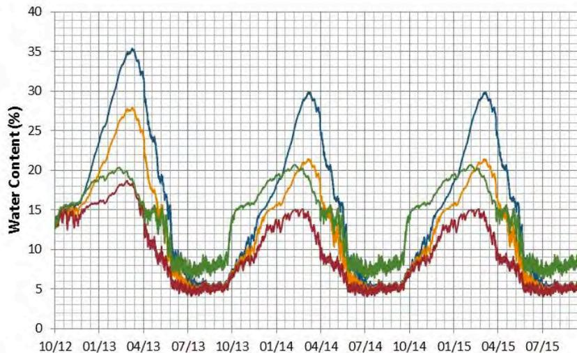
**Figure 9 - Predicted MC at Inside of Sheathing on North-facing Roof Assemblies with Various Wintertime Indoor Humidity Levels**
