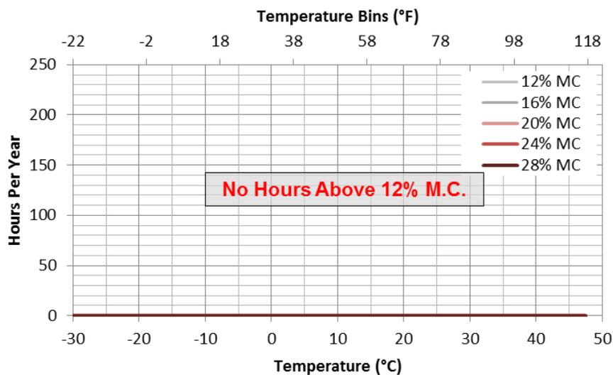
**Figure 21 – Biodegradation Risk Plot for Compact (5.5 in., R23.6) Hybrid Insulation Retrofit Roof with Wintertime indoor @ 40%RH (no air leaks)**
