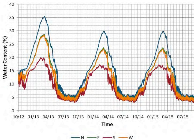
**Figure 8 – Predicted MC at Inside of Sheathing on Common Retrofit Roof Assemblies Facing Cardinal Directions and with Wintertime Indoor @ 40%RH**
