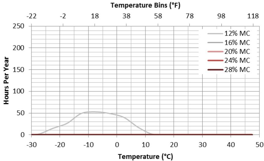
**Figure 24 – Biodegradation Risk Plot for Bottom-Ventilated Retrofit Roof with Wintertime Indoor @ 40%RH (no air leaks)**
