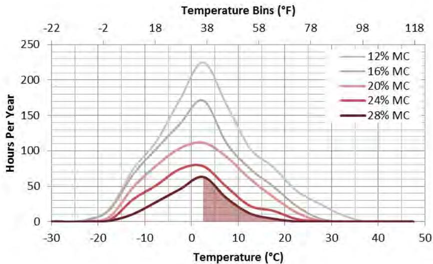
**Figure 27 – Biodegradation Risk Plot for Top-Ventilated Retrofit OSB Roof w/ Wintertime Indoor @ 40%RH and 0.0012 cfm/ ft<sup>2</sup> air leak**
