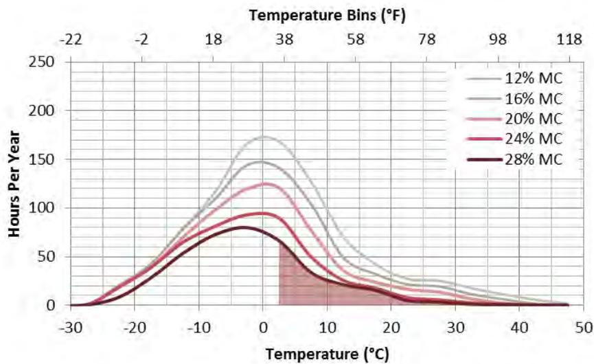
**Figure 15 – Biodegradation Risk Plot for North-facing Roof with Wintertime Indoor @ 40%RH and 0.0012 cfm/ ft<sup>2</sup> air leak**
