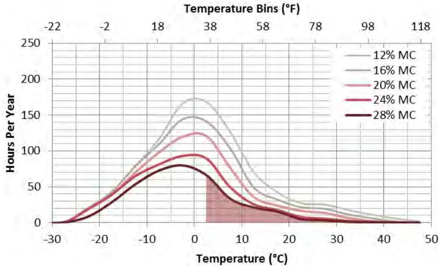
**Figure 26 – Biodegradation Risk Plot for North-facing Common Retrofit Roof with Wintertime Indoor @ 40%RH and 0.0012 cfm/ ft<sup>2</sup> air leak**
