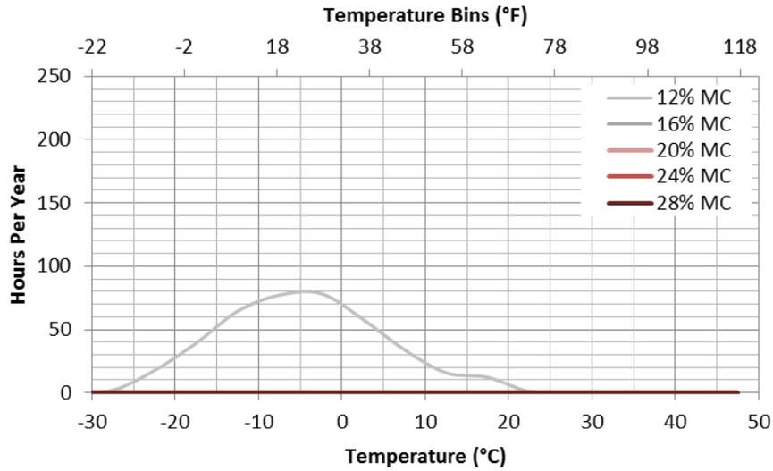
**Figure 19 – Biodegradation Plot for Exterior Insulated Retrofit Roof with Wintertime Indoor @ 40%RH and 0.0012 cfm/ ft<sup>2</sup> air leak**
