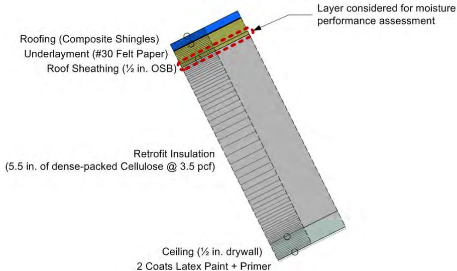
**Figure 5 – Model of Common (not recommended) Retrofit Assembly for Hygrothermal Simulations**
