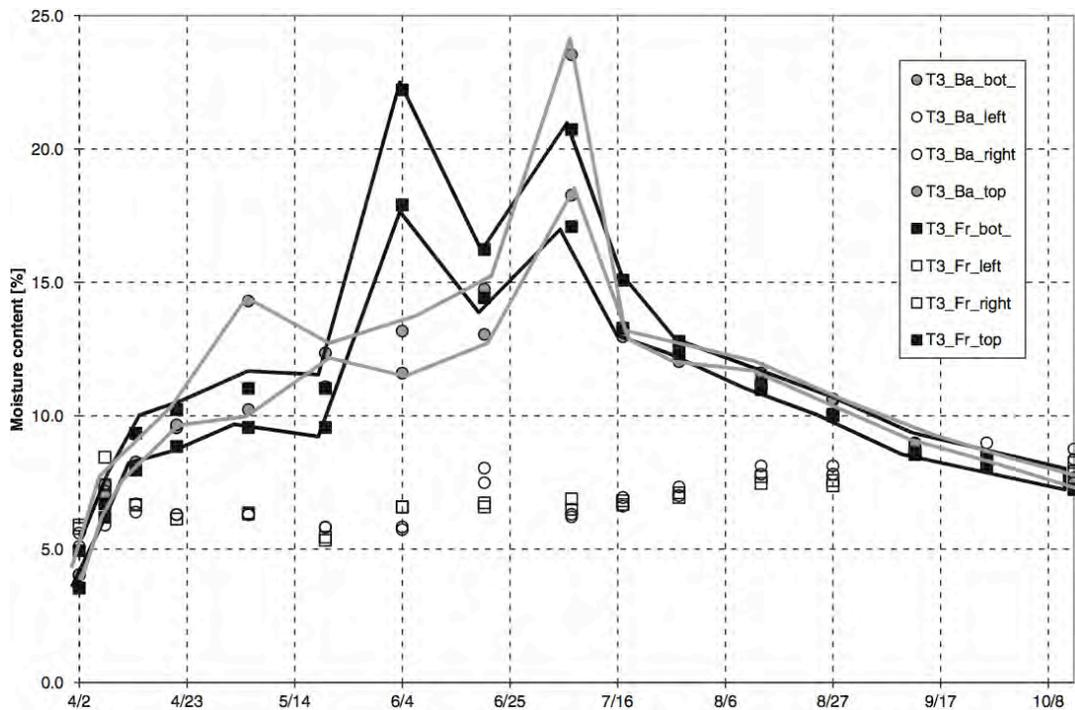
Moisture content distribution in the cellulose insulation of 200 mm (8 in.) high T3 assembly with long air leakage flow path. The black-lined zone groups the cellulose moisture content samples near the exit end of the assembly. The grey lined zone groups samples close to the interior partition (i.e. the air inlet)
