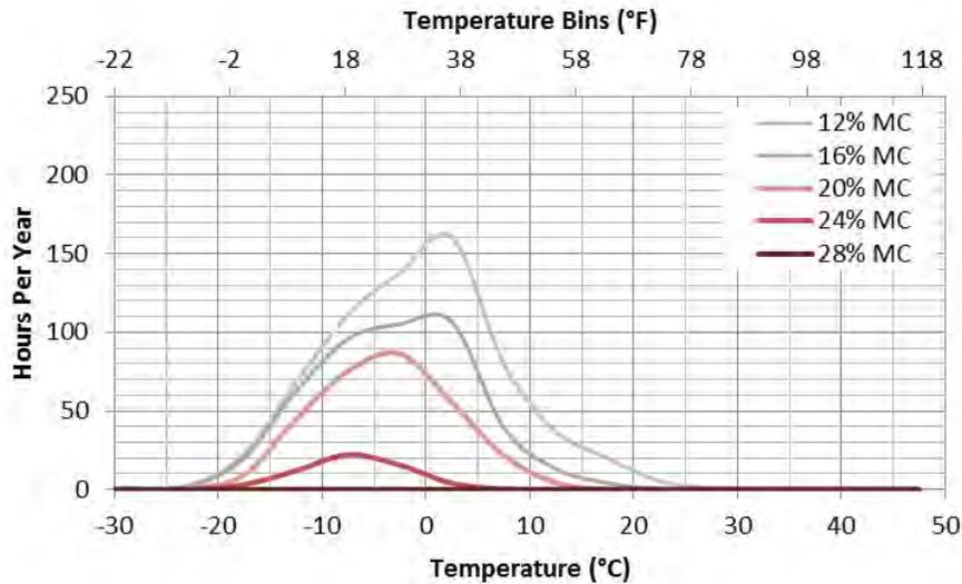
**Figure 28 – Biodegradation Risk Plot for Top-Ventilated Retrofit Plywood Roof w/ Wintertime Indoor @ 40%RH and 0.0012 cfm/ ft<sup>2</sup> air leak**
