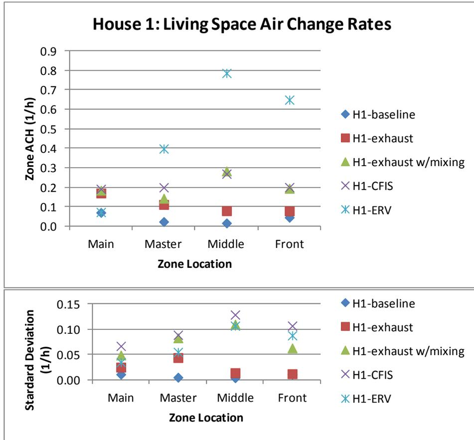
**Figure 19. Air change rates in the living space zones for House 1 (vented attic), for the Baseline test and four different ventilation systems**
