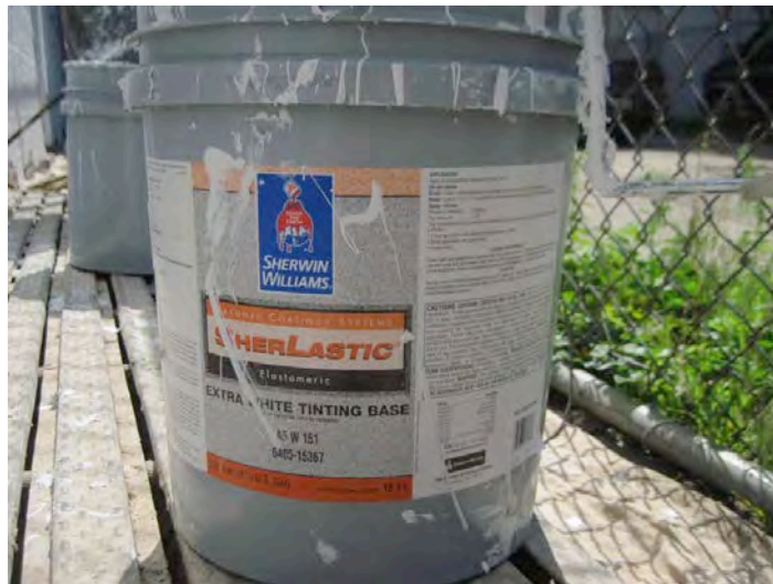
Figure 12. Commercially available elastomeric paint used by over-clad contractor (Credit: Scott Sanders, CEDA).
