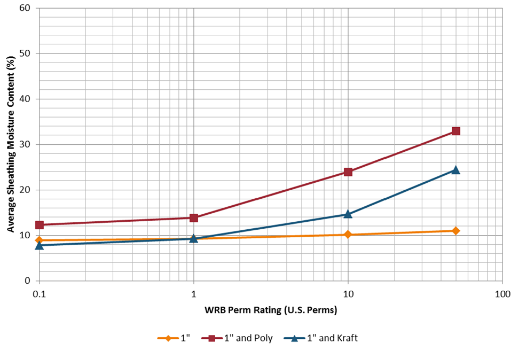
Figure 17. Average interior side sheathing MC for 1 in., 1 in.+ Poly, and 1 in.+ Kraft at various WRB permeances.
