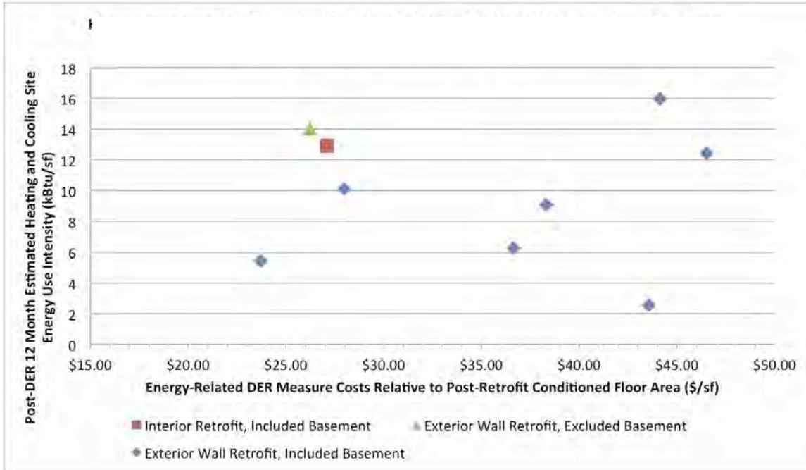
**Figure 51. Heating and cooling site EUI versus combined energy-related DER measure costs/ft<sup>2</sup> conditioned floor area**
