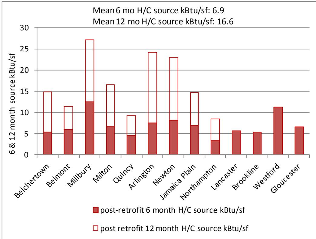
**Figure 25. Post-retrofit 6- and 12-month source kBtu/ft<sup>2</sup> for heating and cooling**
