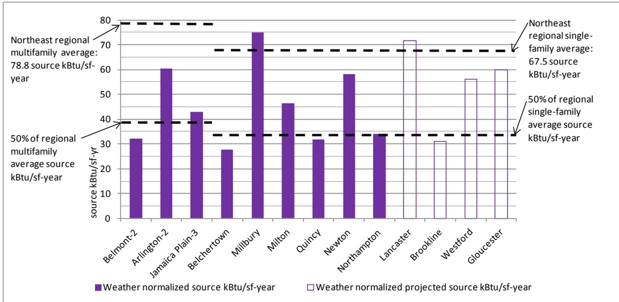
**Figure 19. Weather-normalized post-retrofit source kBtu/ft<sup>2</sup>-yr**
