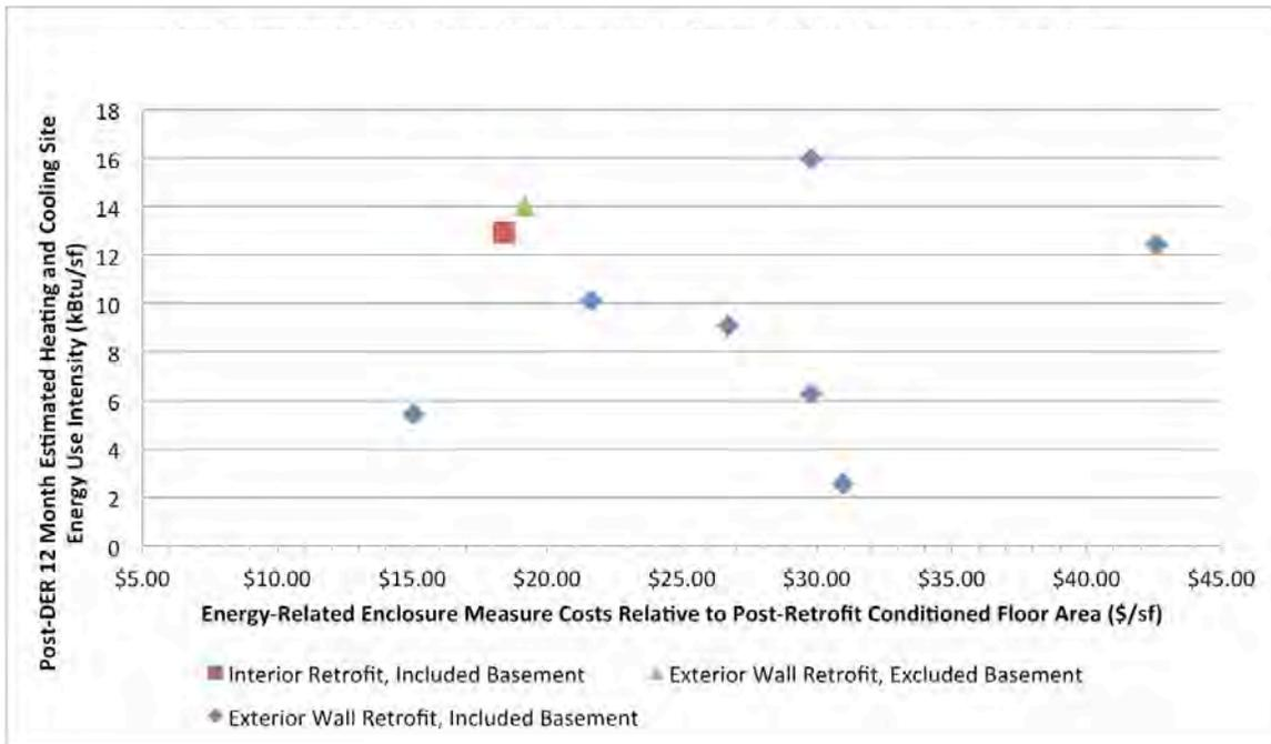
**Figure 49. Heating and cooling site EUI versus energy-related enclosure measure costs/ft<sup>2</sup> conditioned floor area**
