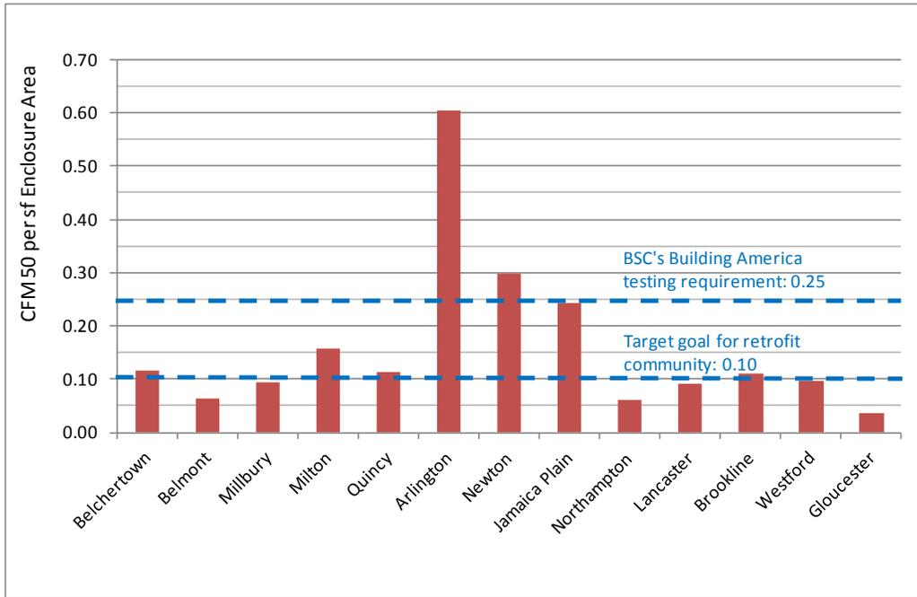
**Figure 5. Post-retrofit CFM50/ft<sup>2</sup> enclosure area results**
