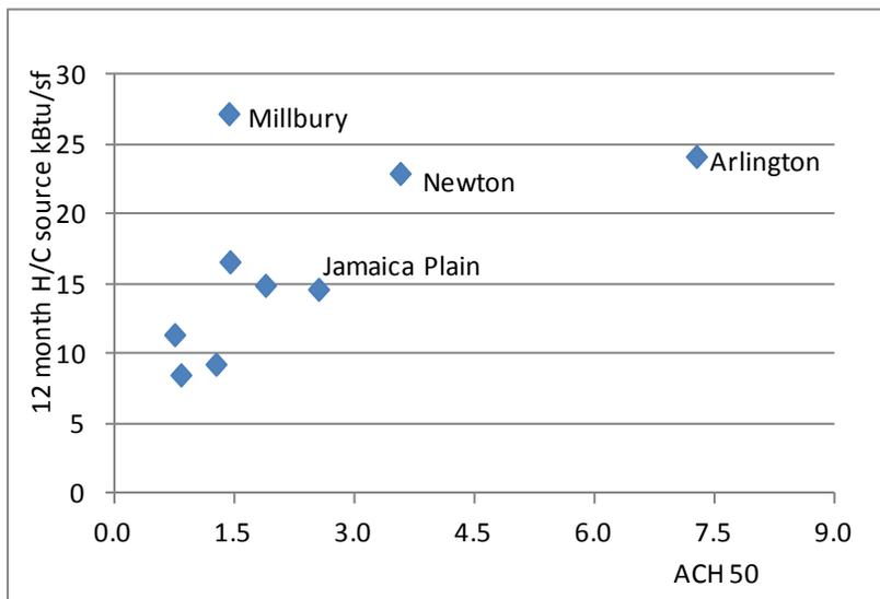
**Figure 32. Relationship between 12-month heating and cooling source kBTU/ft<sup>2</sup> and ACH50**
