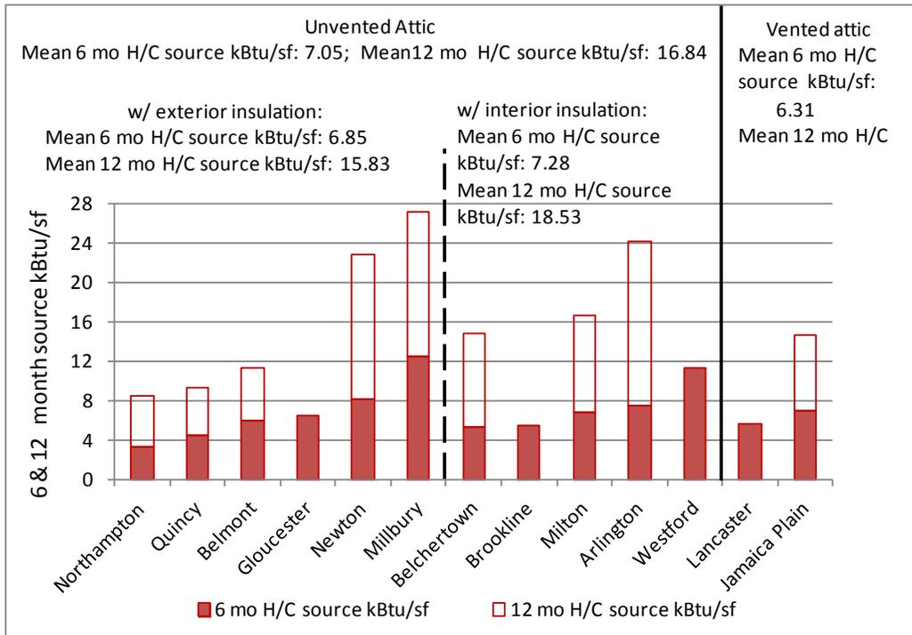
**Figure 30. 6- and 12-month heating and cooling source kBtu/ft<sup>2</sup> grouped by roof and attic treatment**
