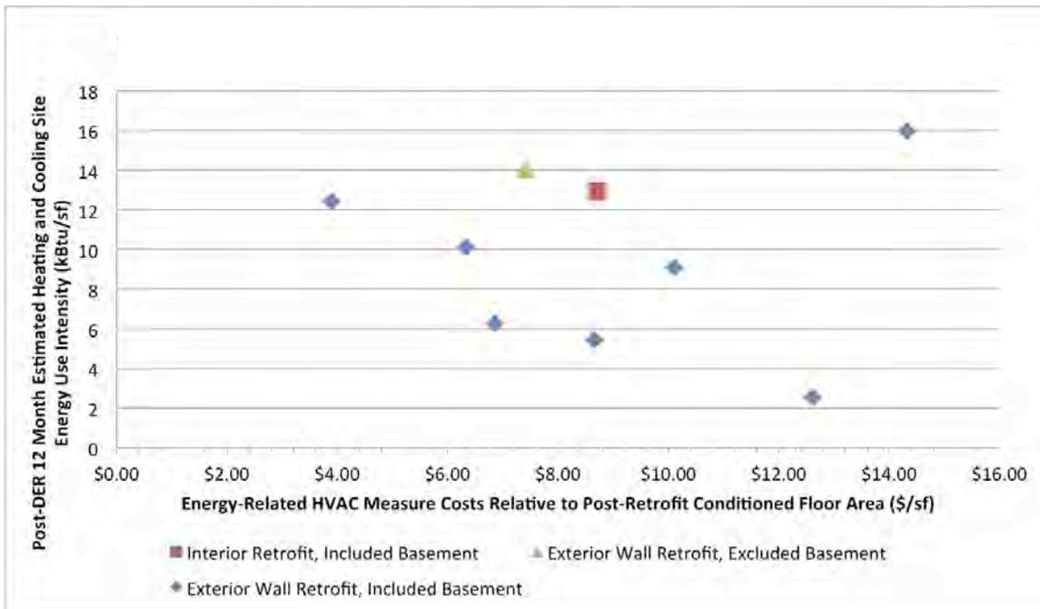
**Figure 50. Heating and cooling site EUI versus energy-related HVAC measure costs/ft<sup>2</sup> conditioned floor area**
