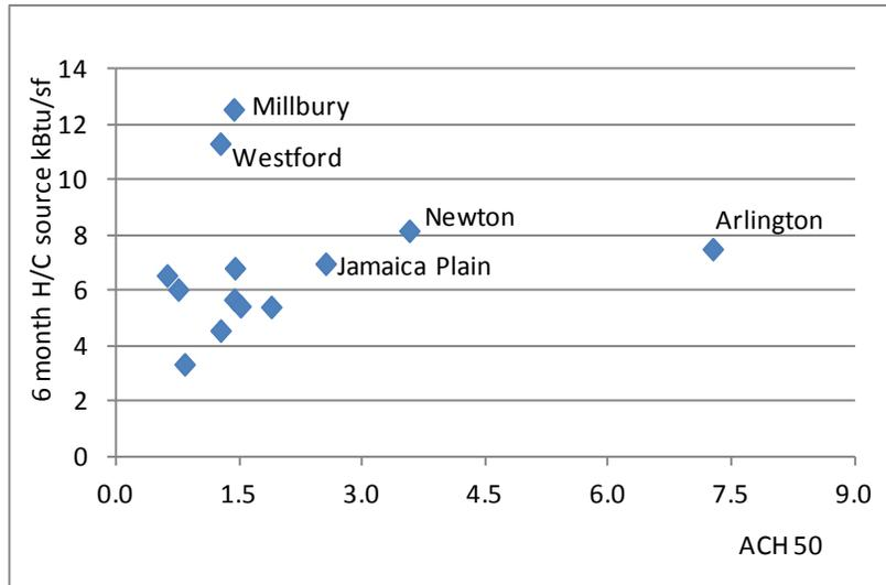
**Figure 31. Relationship between 6-month heating and cooling source kBTU/ft<sup>2</sup> and ACH50**
