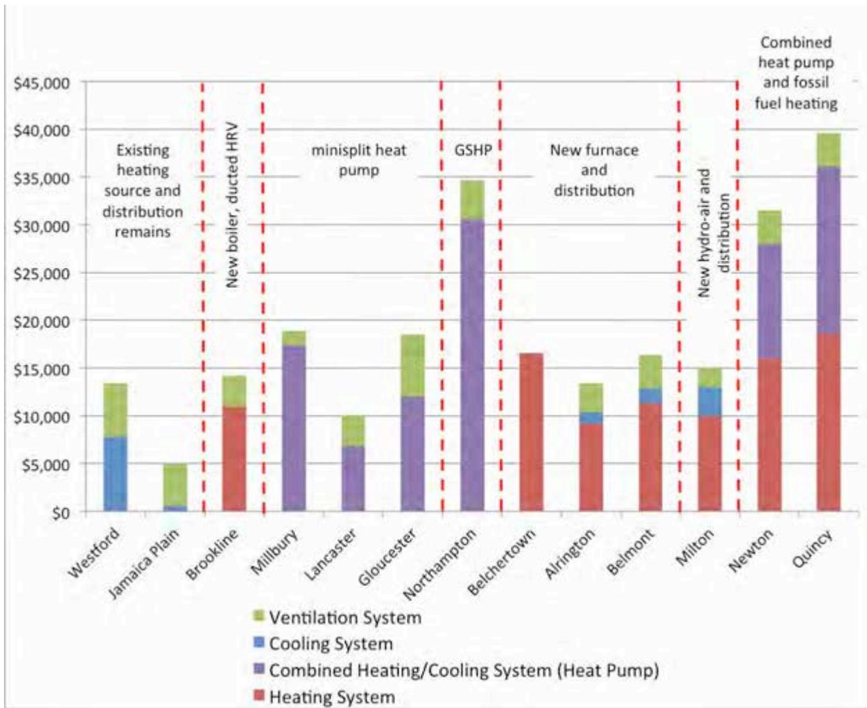
**Figure 46. Unit (per system) costs for HVAC measures**
