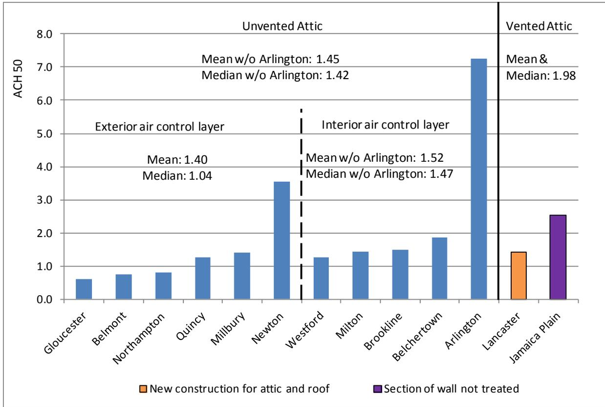
**Figure 12. ACH50 results for unvented versus vented attic**
