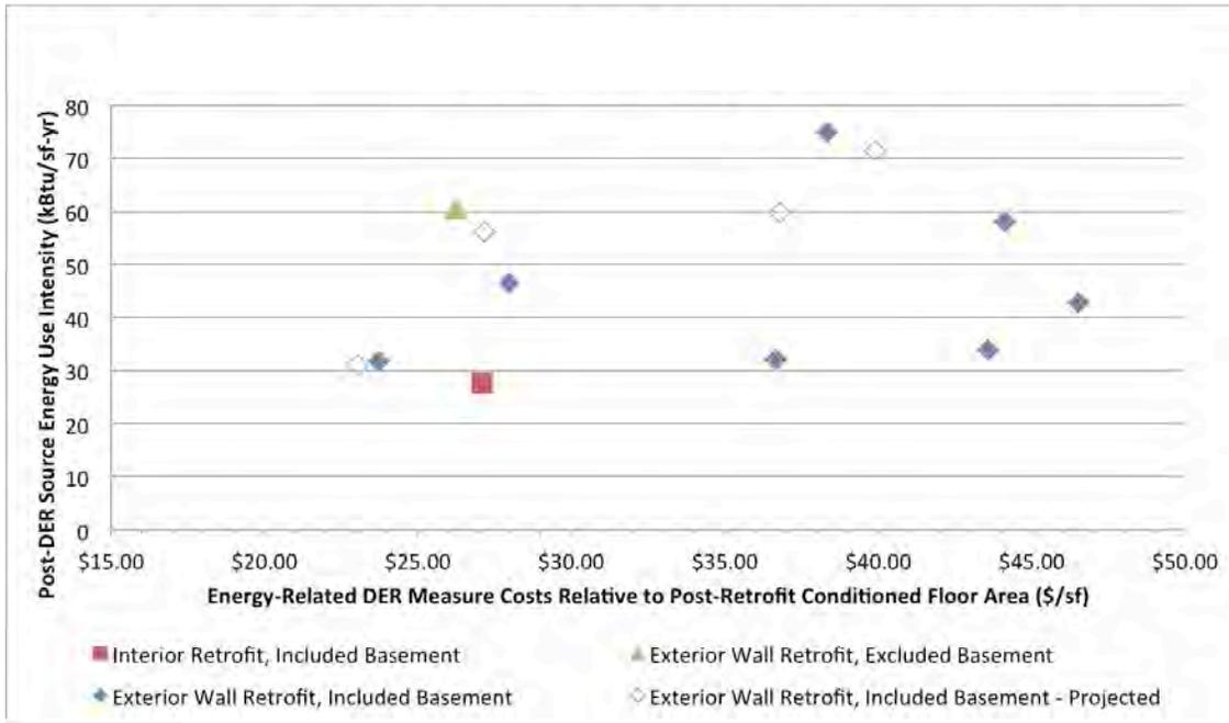
**Figure 53. Source EUI versus combined energy-related DER measure costs/ft<sup>2</sup> conditioned floor area**
