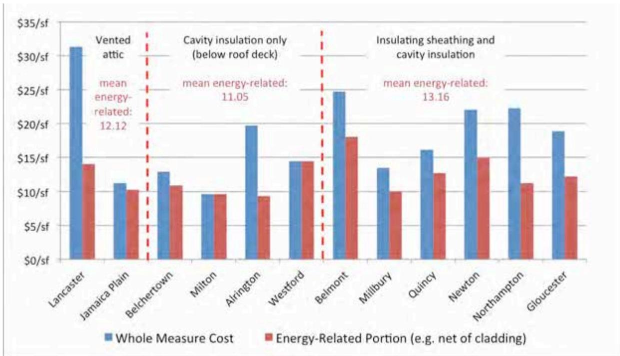
**Figure 35. Unit costs for attic and roof measures**
