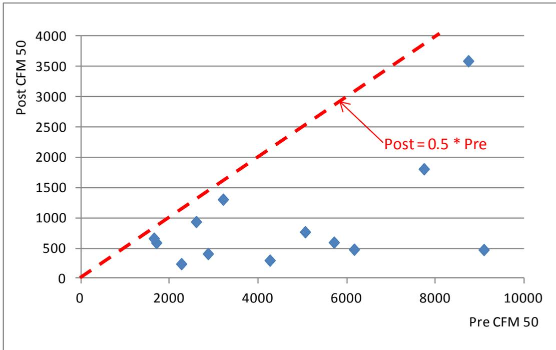
**Figure 4. Post-retrofit CFM50 versus pre-retrofit CFM50**
