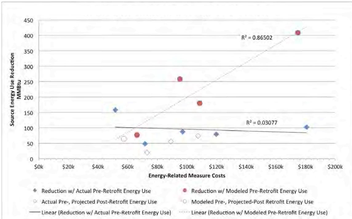
Figure 55. Source energy use reduction versus combined energy-related DER measure costs
