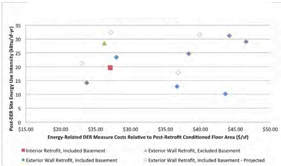
**Figure 52. Site EUI versus combined energy-related DER measure costs/ft<sup>2</sup> conditioned floor area**
