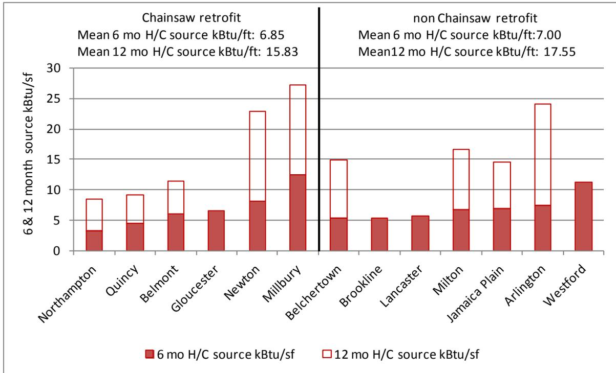
**Figure 28. Chainsaw versus non-chainsaw 6- and 12-month heating and cooling source kBtu/ft<sup>2</sup>**
