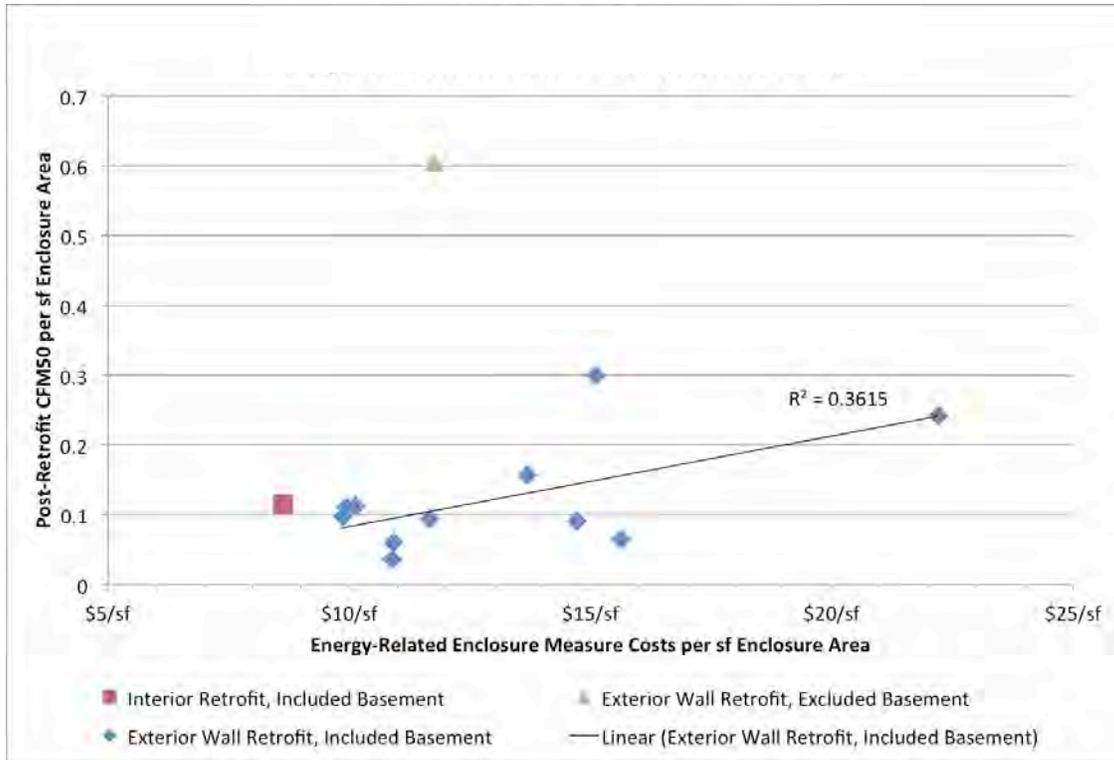
**Figure 47. Post-retrofit CFM50/ft<sup>2</sup> enclosure area versus energy-related enclosure measure costs/ft<sup>2</sup> enclosure area**
