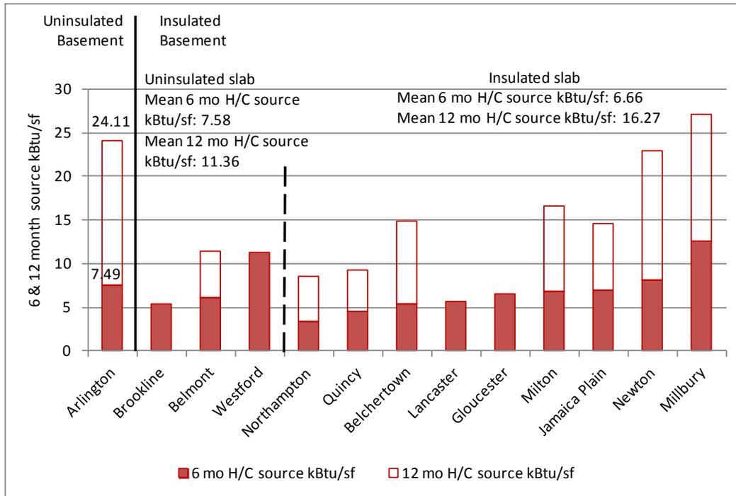
**Figure 29. 6- and 12-month heating and cooling source kBTU/ft<sup>2</sup> grouped by basement treatment**
