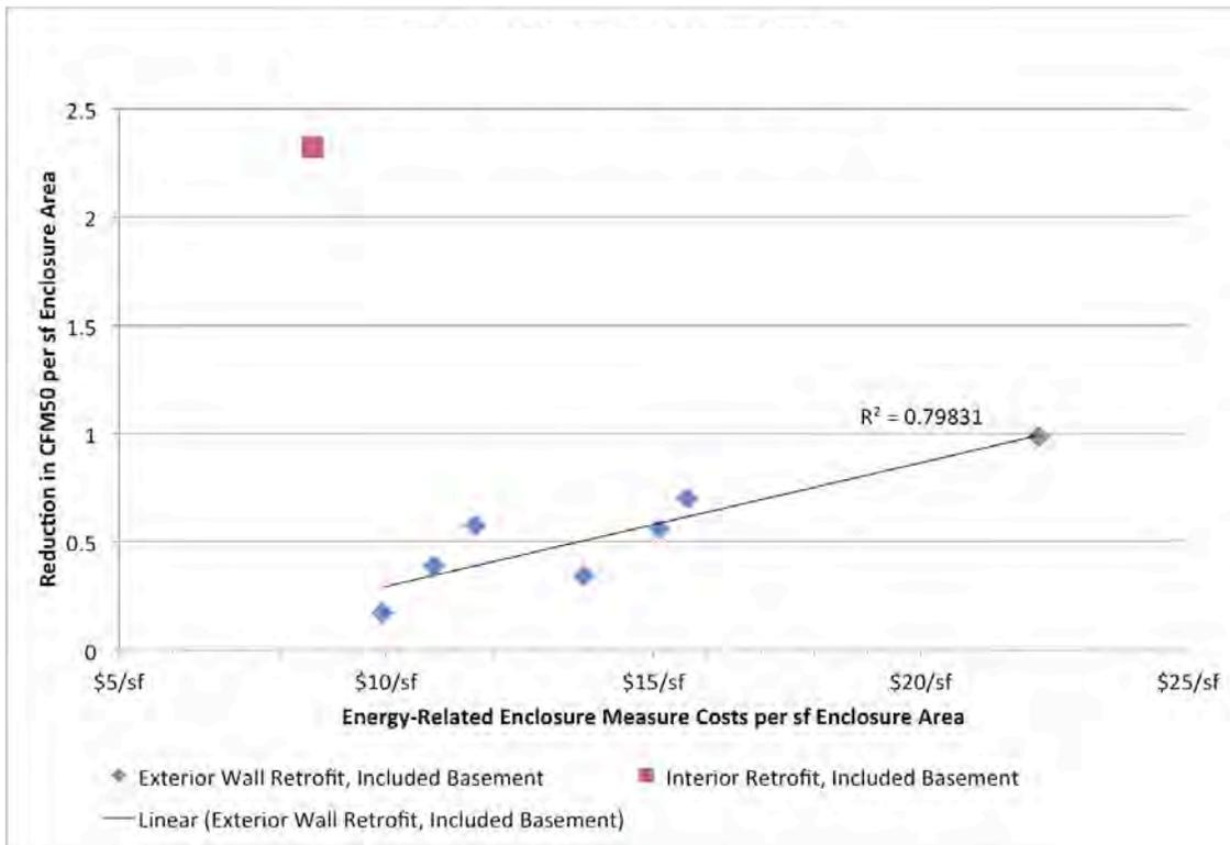
**Figure 48. Reduction in post-retrofit CFM50/ft<sup>2</sup> enclosure area versus energy-related enclosure measure costs/ft<sup>2</sup> enclosure area**
