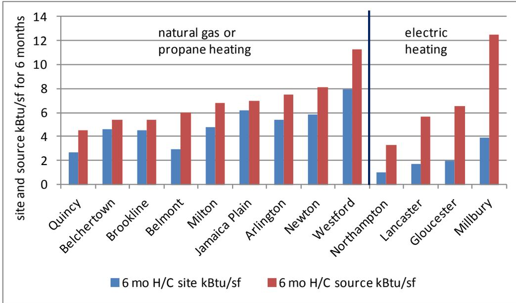
**Figure 27. Electric versus nonelectric 6-month site and source heating and cooling kBtu/ft<sup>2</sup> for February 12–July 12**
