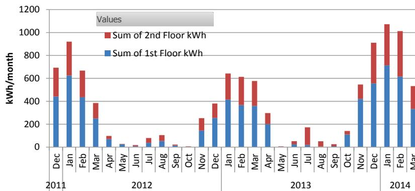
Figure 35. Devens Lot 3 monthly MSHP kilowatt-hour consumption (heating and cooling)
