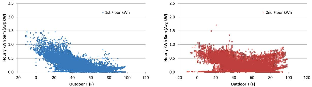
**Figure 26. Easthampton Lot 13 hourly kilowatt-hour versus outdoor temperature**
