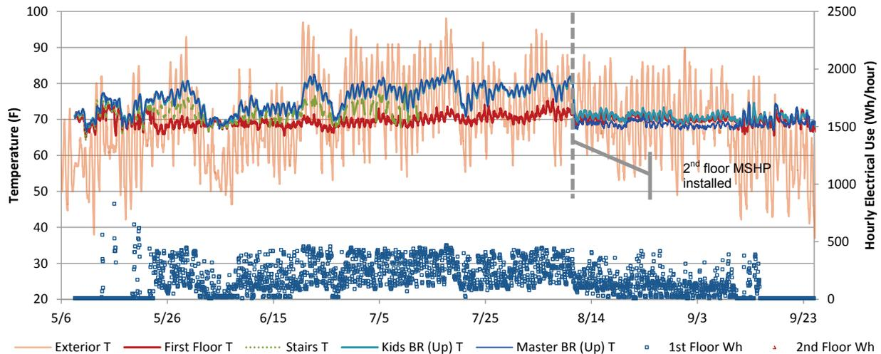
**Figure 77. Summer 2012 interior and exterior temperatures at Lot 17, pre- and post-retrofit**
