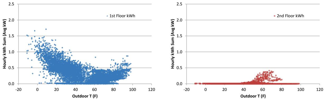
**Figure 27. Easthampton Lot 17 hourly kilowatt-hour versus outdoor temperature**
