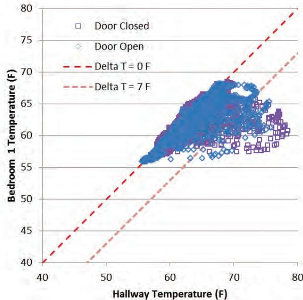
**Figure 1. Townsend data of hall temperature versus bedroom 1 temperature, door open/closed**
