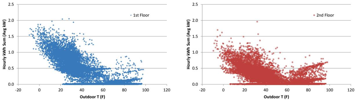
**Figure 25: Devens Lot 3 hourly kilowatt-hours versus outdoor temperature**
