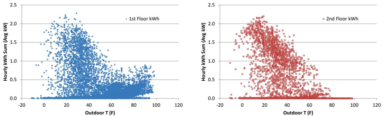
**Figure 28. Easthampton Lot 23 hourly kilowatt-hours versus outdoor temperature**
