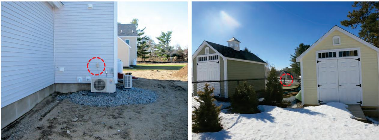
**Figure 19. Devens measurement of exterior conditions (T/RH)**
