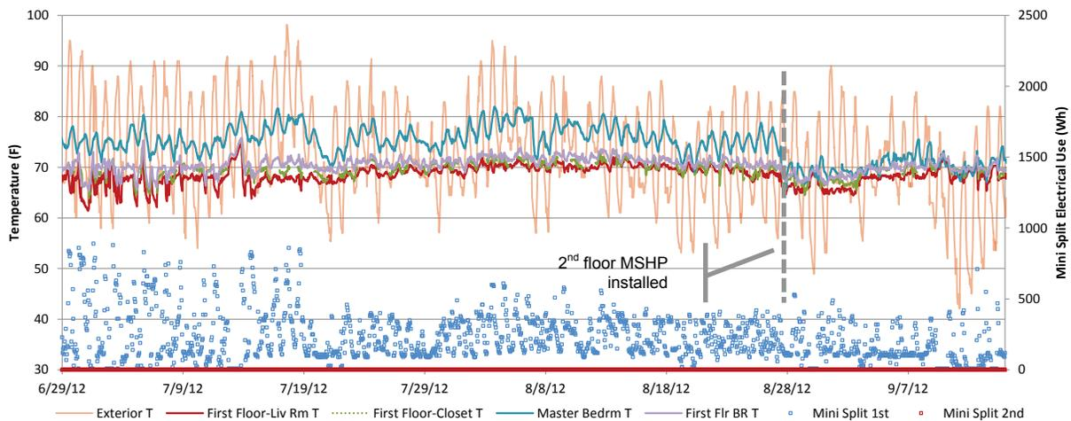
**Figure 78. Summer 2012 interior and exterior temperatures at Lot 23, pre- and post-retrofit**
