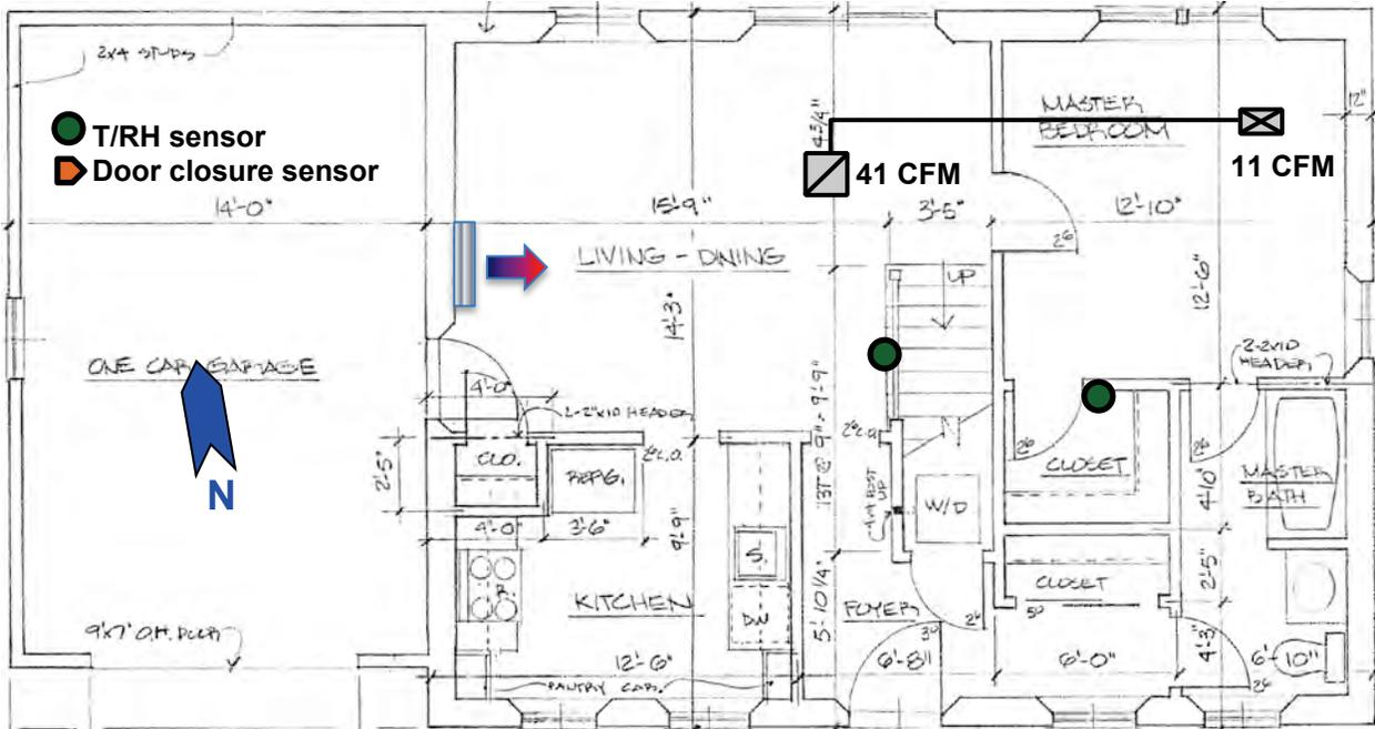
Figure 121. Easthampton Lot 17 first-floor plan, MSHP locations, monitoring locations
