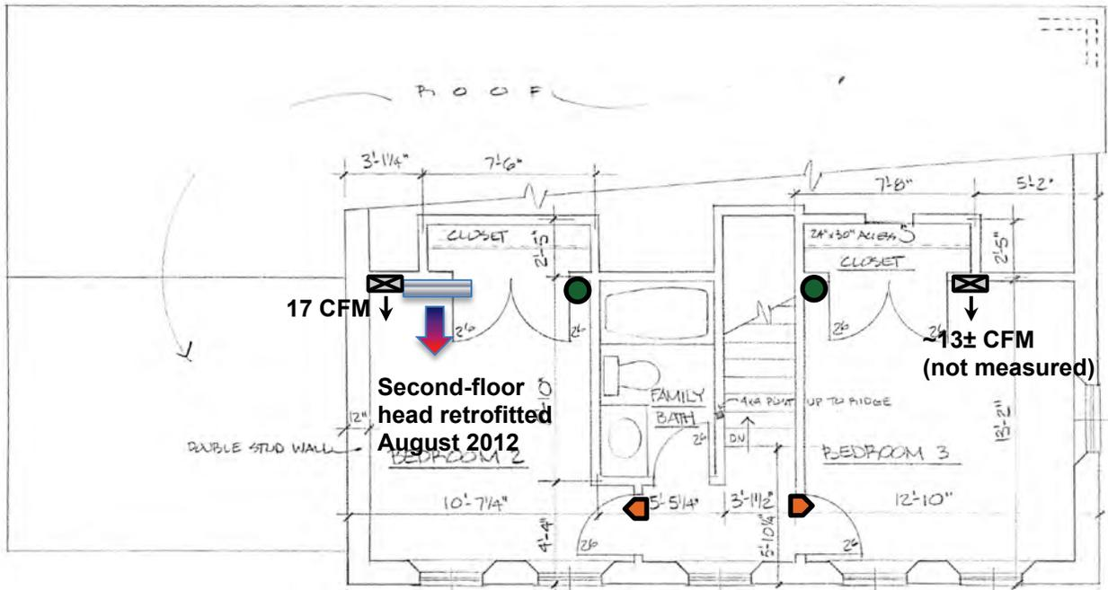
Figure 122. Easthampton Lot 17 second-floor plan, MSHP locations, monitoring locations
