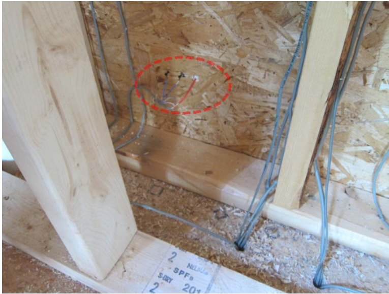
Figure 19. Sheathing MC/temperature sensor locations (bottom shown in picture)
