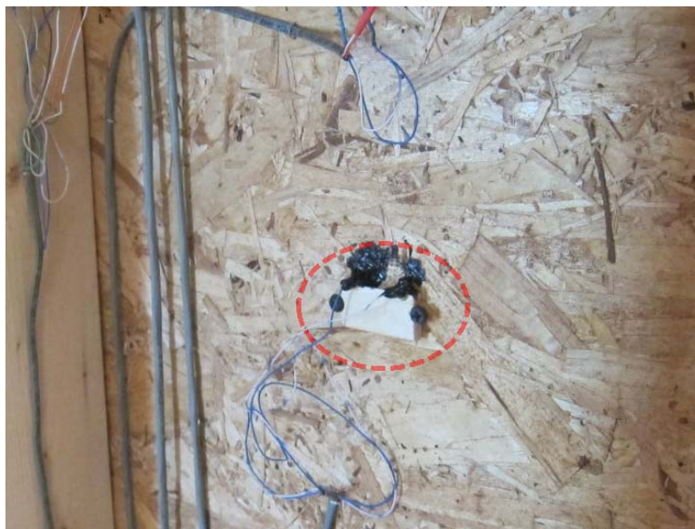
Figure 22. Sheathing-insulation interface wafer sensor location
