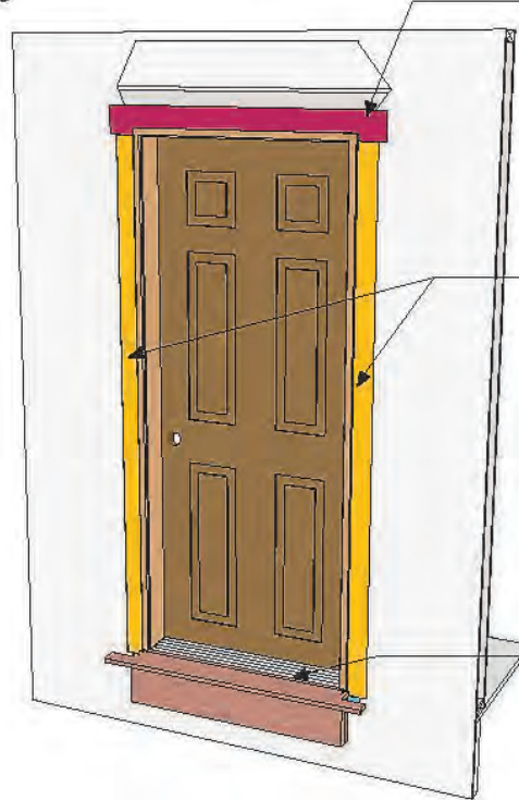
Figure 54. Steps 9 and 10 of installation sequence for new door or reinstalled door in a high performance mineral fiber retrofit wall assembly
