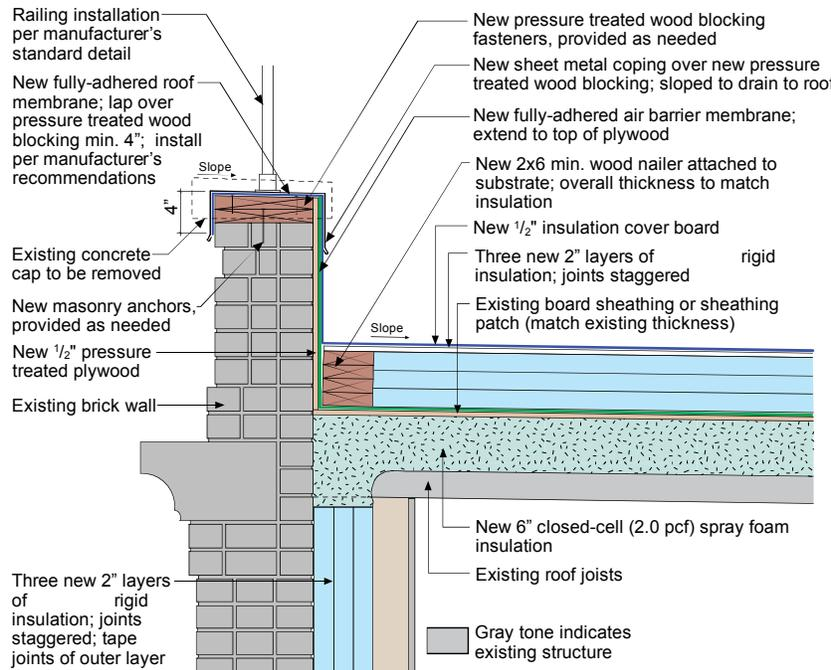
**Figure 8: Flat roof retrofit detail at parapet**
