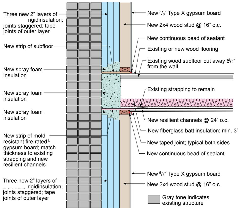
**Figure 10: Unit-to-unit floor/ceiling assembly at exterior wall**
