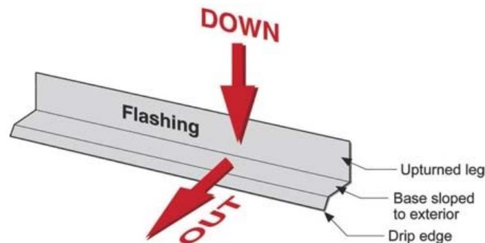
**Figure 3: The "down" and "out" approach to flashing**
