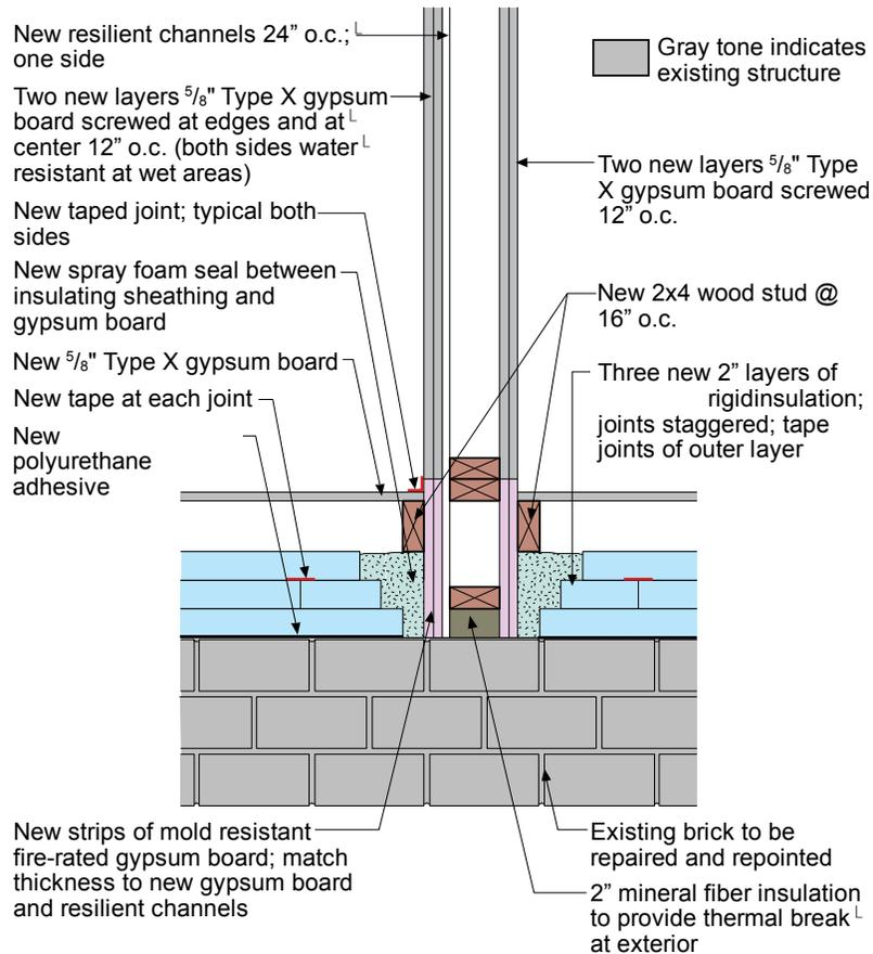
**Figure 11: Rated partition intersection with exterior wall**
