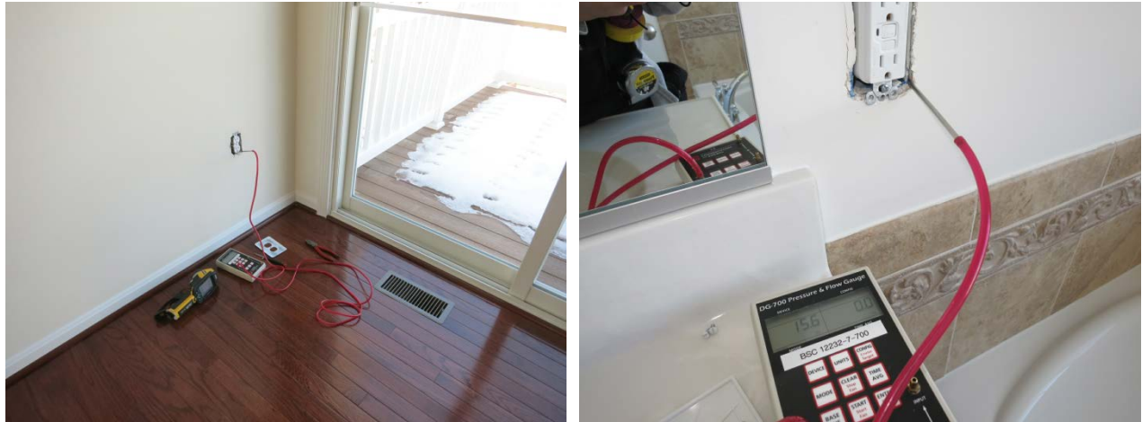
Figure 62. Pressure difference measurements at electrical box penetrations
