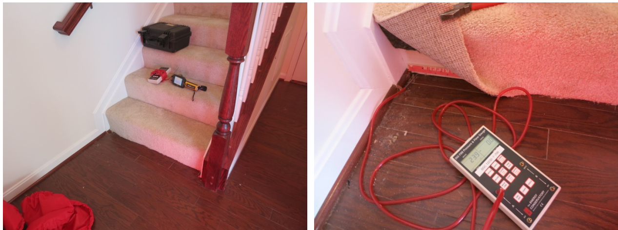
Figure 49. Measurement of pressure difference under stairs, location A
