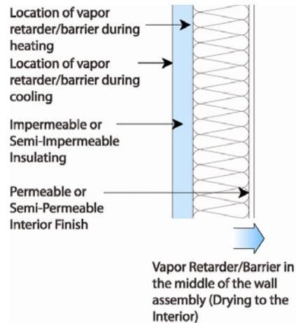
The thermal gradient can be predicted by examining the individual proportion of thermal resistance provided by each component. Each different component will provide a percentage of the total thermal resistance of the assembly. Therefore, the change in temperature of any component is based on the percentage of thermal resistance provided by that component multiplied by the overall temperature difference across the assembly.
