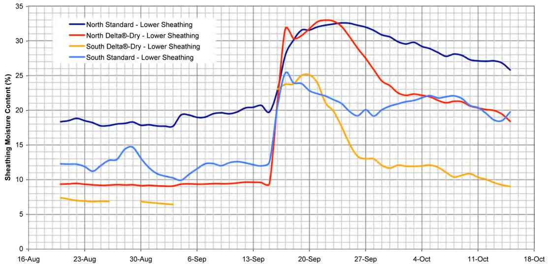
**Figure 7: Lower sheathing moisture content comparison during an intentional wetting event**
