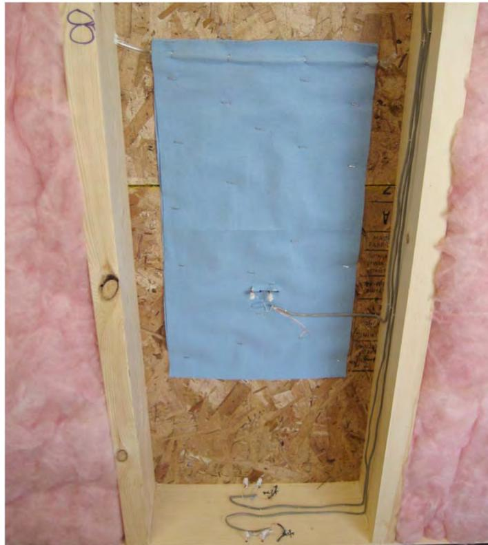
**Figure 4: Installed Wetting Apparatus in a Test Wall**
