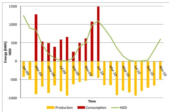
Figure 4 Electrical consumption and production; Heating Degree Days 2009-2010
