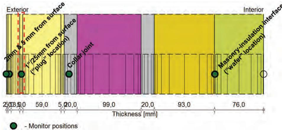
Figure 14 WUFI model of Wall S1/N1 (insulated “thin” wall) with materials and monitor positions.
