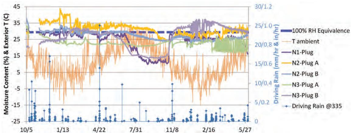
**Figure 10** North insulated wall plug sensor moisture contents with exterior temperatures and driving rain.
