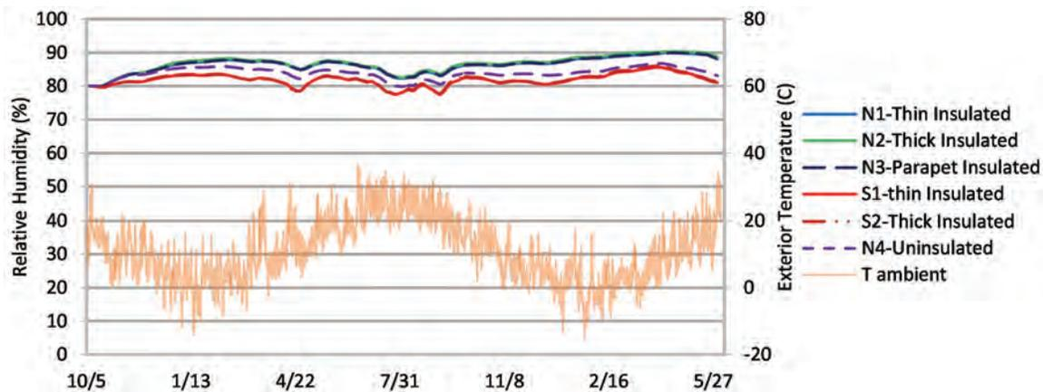
Figure 16 Simulation collar joint (mortar layer) relative humidity; exterior temperature for reference.
