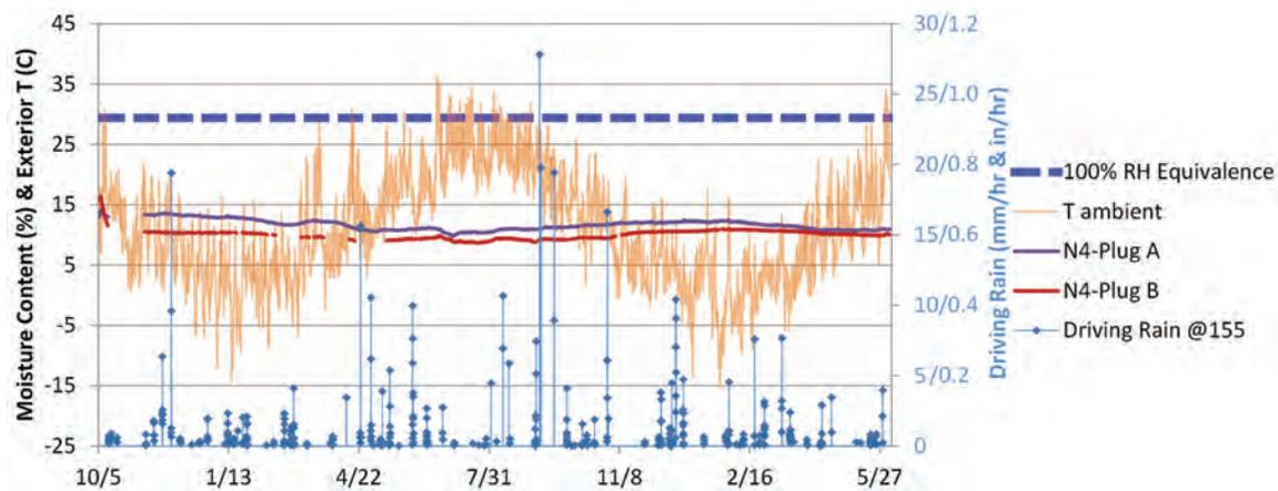
Figure 12 North uninsulated wall plug sensor moisture contents with exterior temperatures and driving rain.
