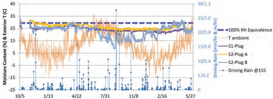
Figure 11 South insulated wall plug sensor moisture contents with exterior temperatures and driving rain.
