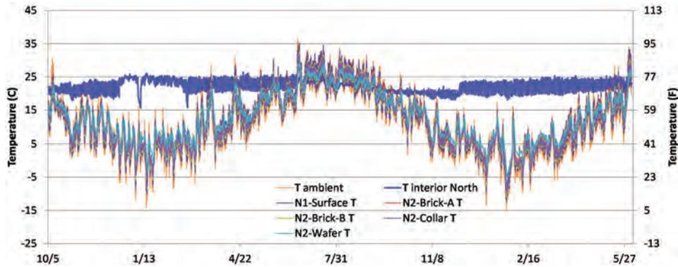
Figure 8 North insulated wall representative temperatures, with interior and exterior temperatures.
