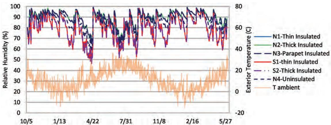
Figure 15 Simulation brick layer 1 in. (25 mm) from exterior face relative humidity; exterior temperature for reference.
