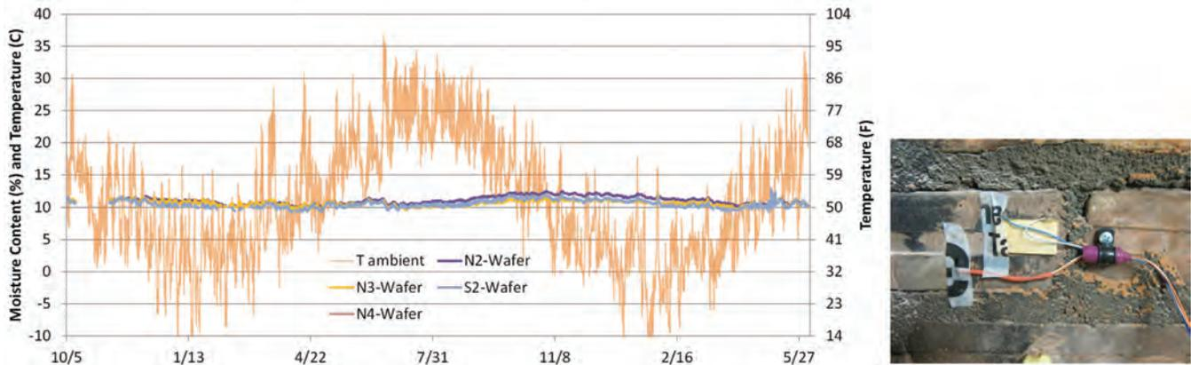
**Figure 13** (L) Moisture wafer results, with exterior temperature for reference; (R) example of wafer sensor.
