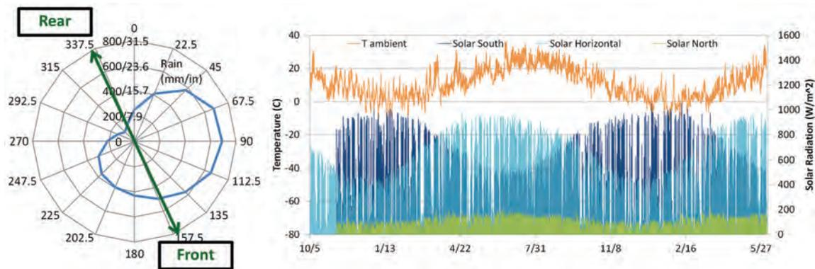
Figure 7 (Left) Driving rain rosette in mm (in.) (calculated from Boston airport data), with building faces shown; (right) solar radiation at building for horizontal, north wall, and south wall.
