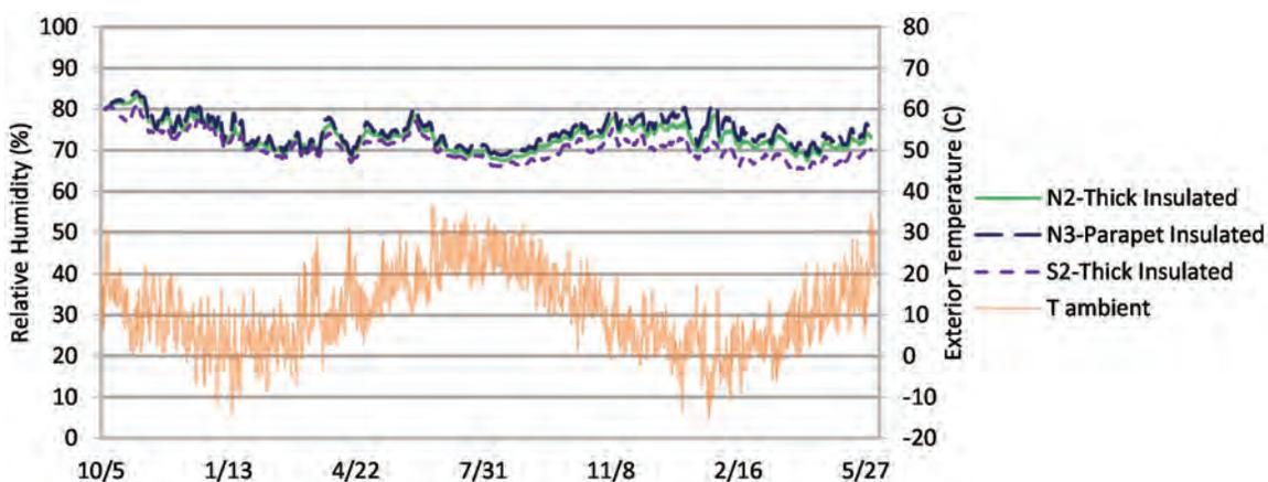
Figure 17 Simulation wafer (masonry-insulation interface) relative humidity; exterior temperature for reference.
