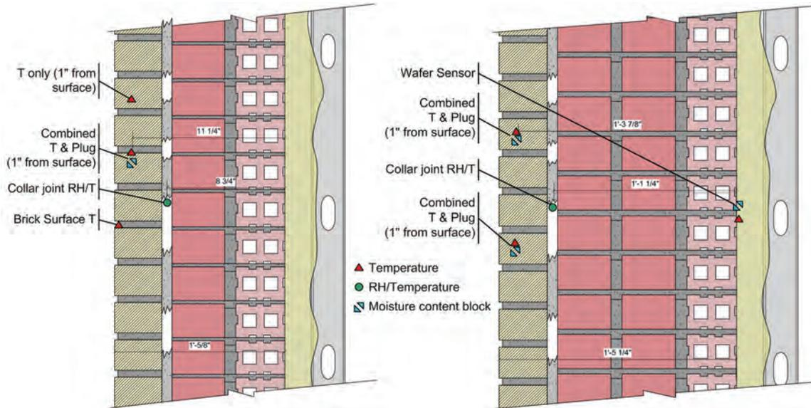
**Figure 3** Sensor package for “thin” wall (N1/S1) left; “thick” wall (N2/S2) right.
