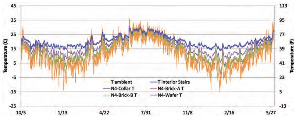
Figure 9 North uninsulated wall representative temperatures, with interior and exterior temperatures.
