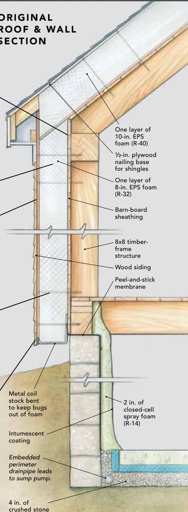
Most of the details worked well, but some could have worked better. Three main changes were incorporated: adding plywood for structural stability, switching to a better air-barrier layer, and adding multiple layers of foam.
