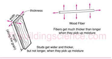
Figure 1 **Wood Shrinkage**
