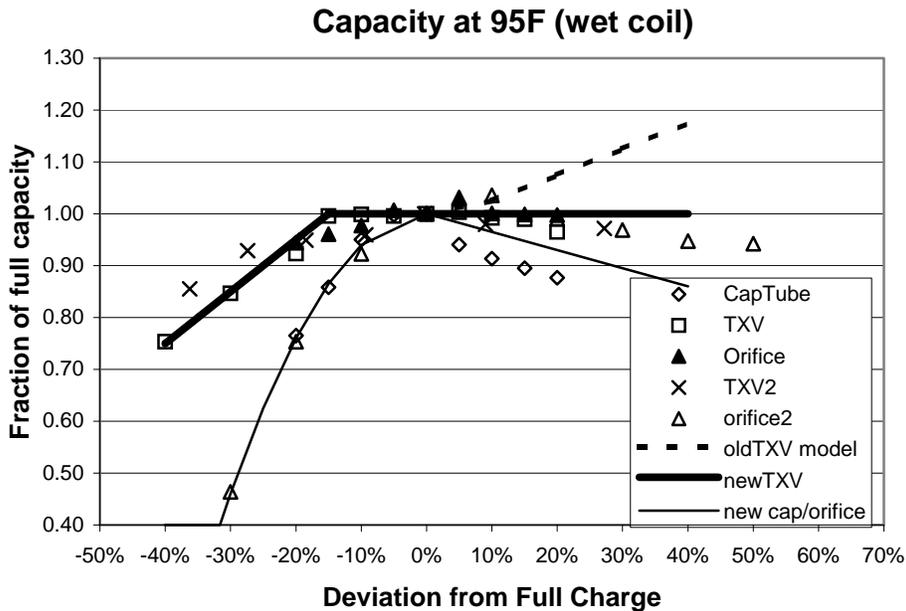
**Figure C10. Wet Coil capacity variation with charge**
