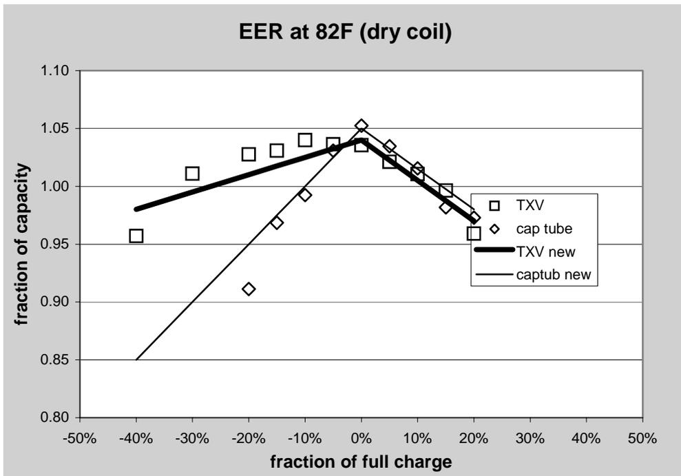
Figure C13. Dry Coil EER variation with charge
