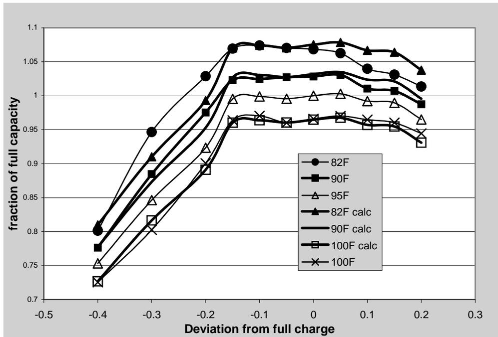
Figure C14. Dry Coil capacity variation with outdoor temperature
