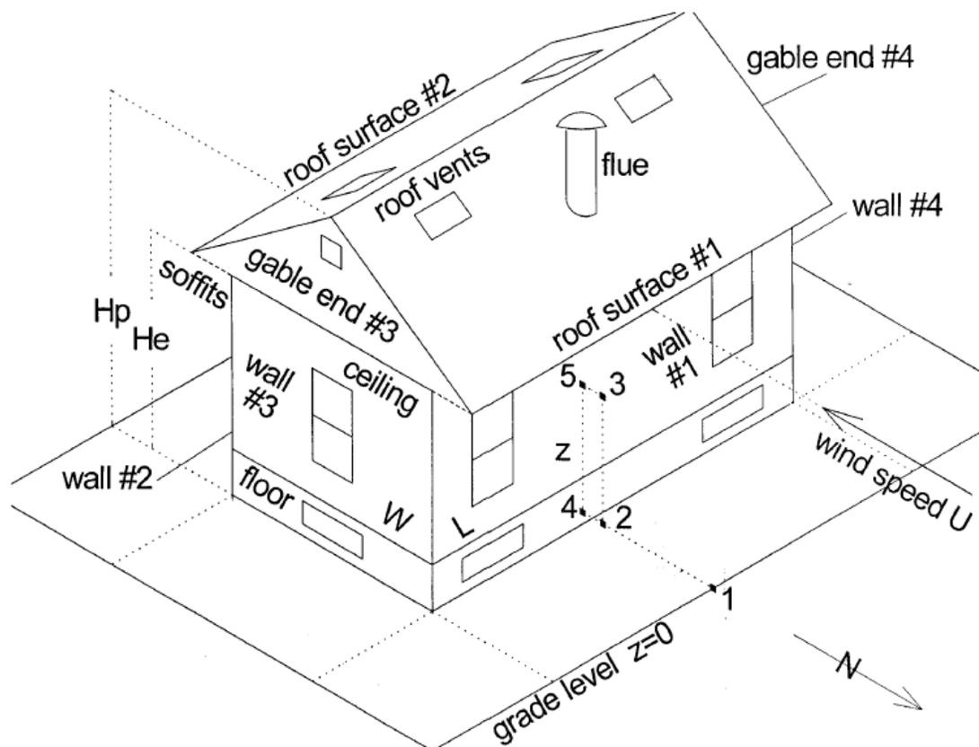
Figure C1. Illustration of house and attic airflow components
