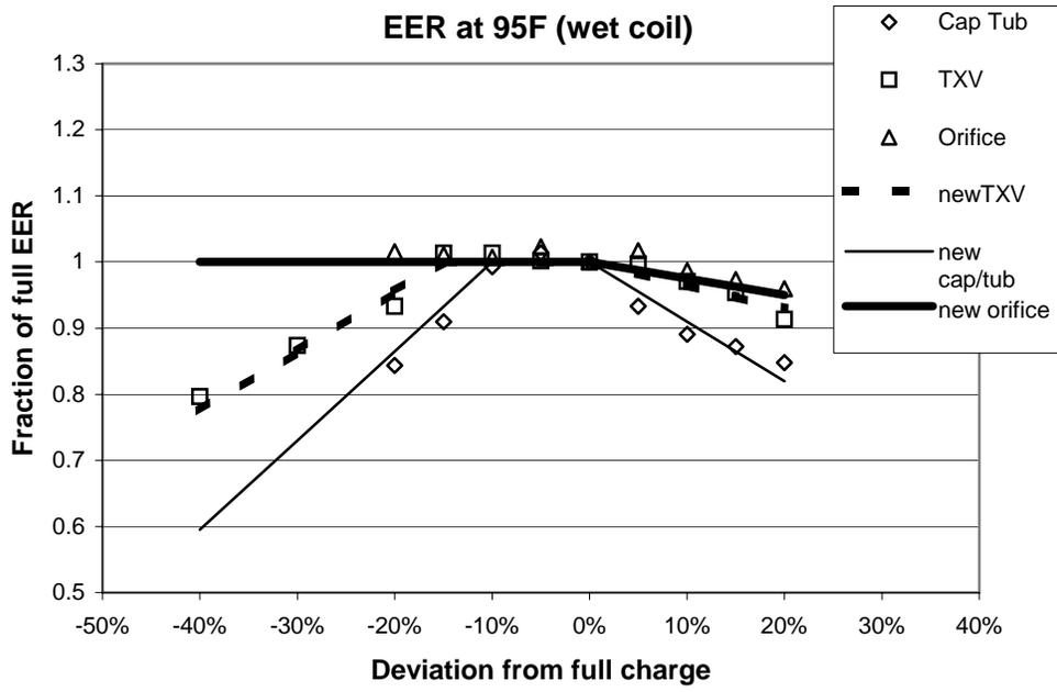
Figure C11. Wet Coil EER variation with charge
