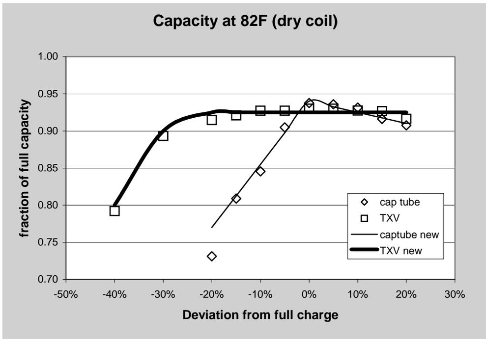
Figure C12. Dry Coil capacity variation with charge
