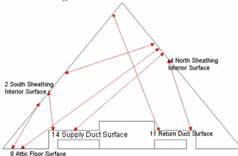
Figure C9: Radiation Transfer for Ducts in Attic
