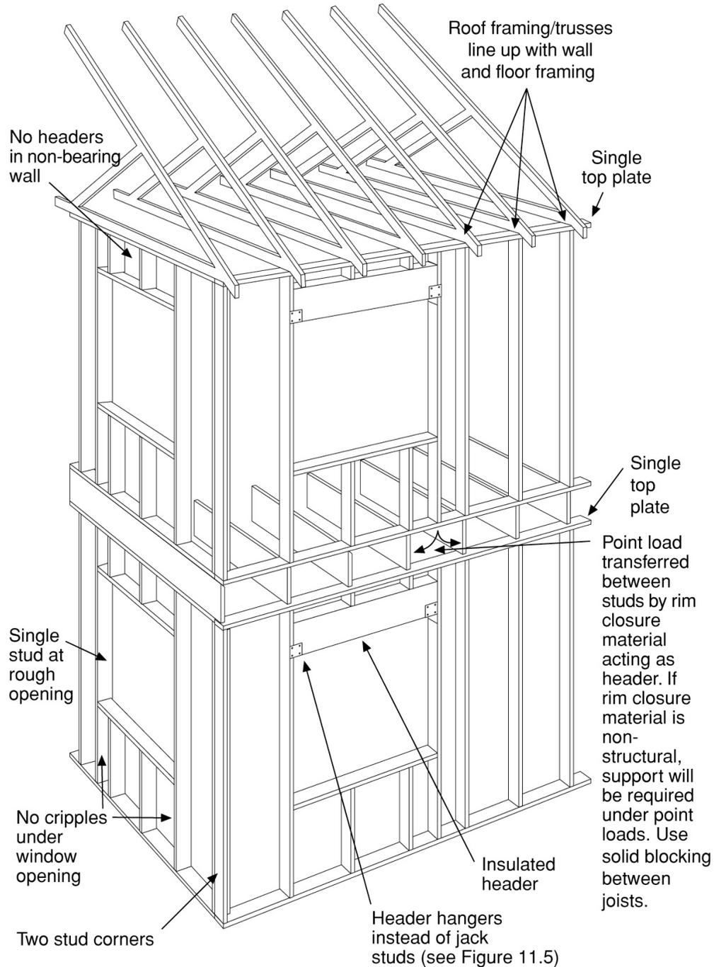
**Figure 6: Advanced Framing Techniques Reduce Thermal Bridging as Well as Waste**
