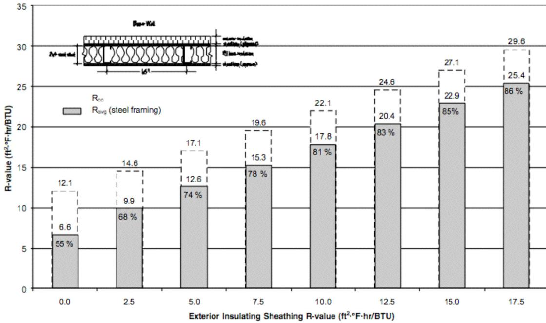
**Figure 4: Impact of Adding Exterior Insulating Sheathing to 3.5 in Steel Stud with R-11 Batt (Bombino & Burnett 1999)**
