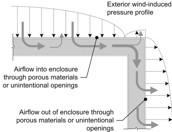
**Figure 15: Airflow through and/or behind insulation driven by exterior wind gradients is termed windwashing**
