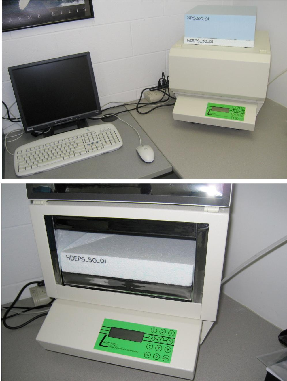
**Figure 1: Commercial Apparatus for Conducting the C518 Standard Thermal Conductivity Test**
