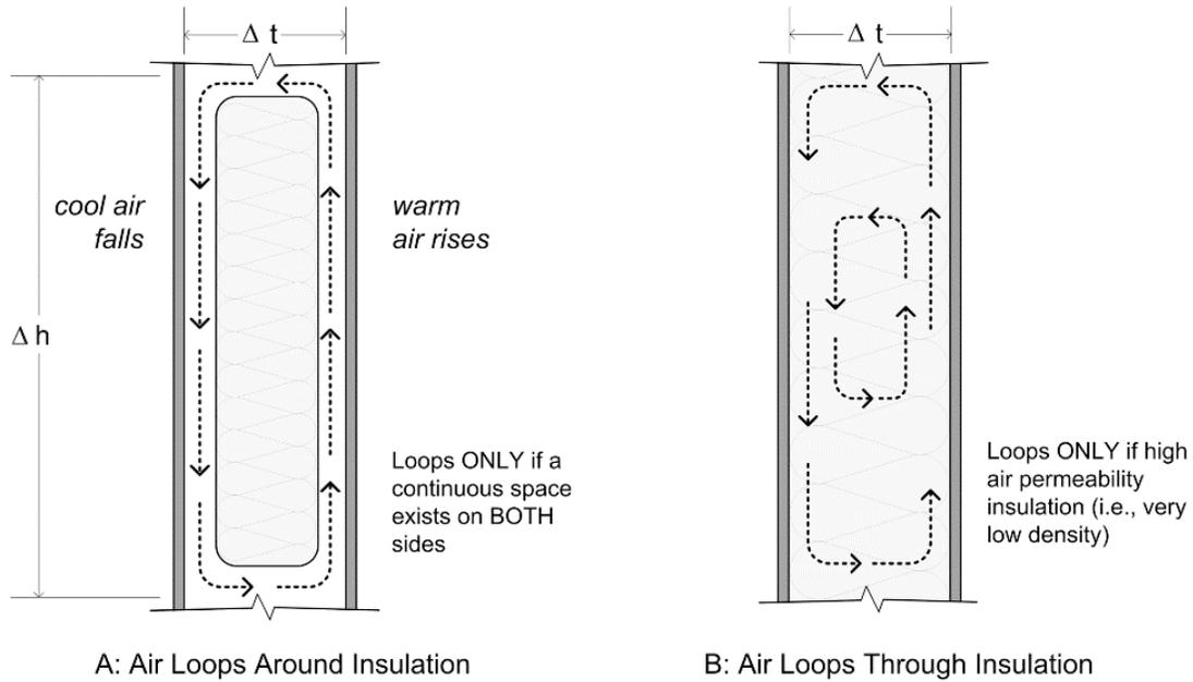
**Figure 8: Convective loops can form around insulation or within insulation. A complete flow path is needed and the larger the temperature difference the larger the driving pressure.**
