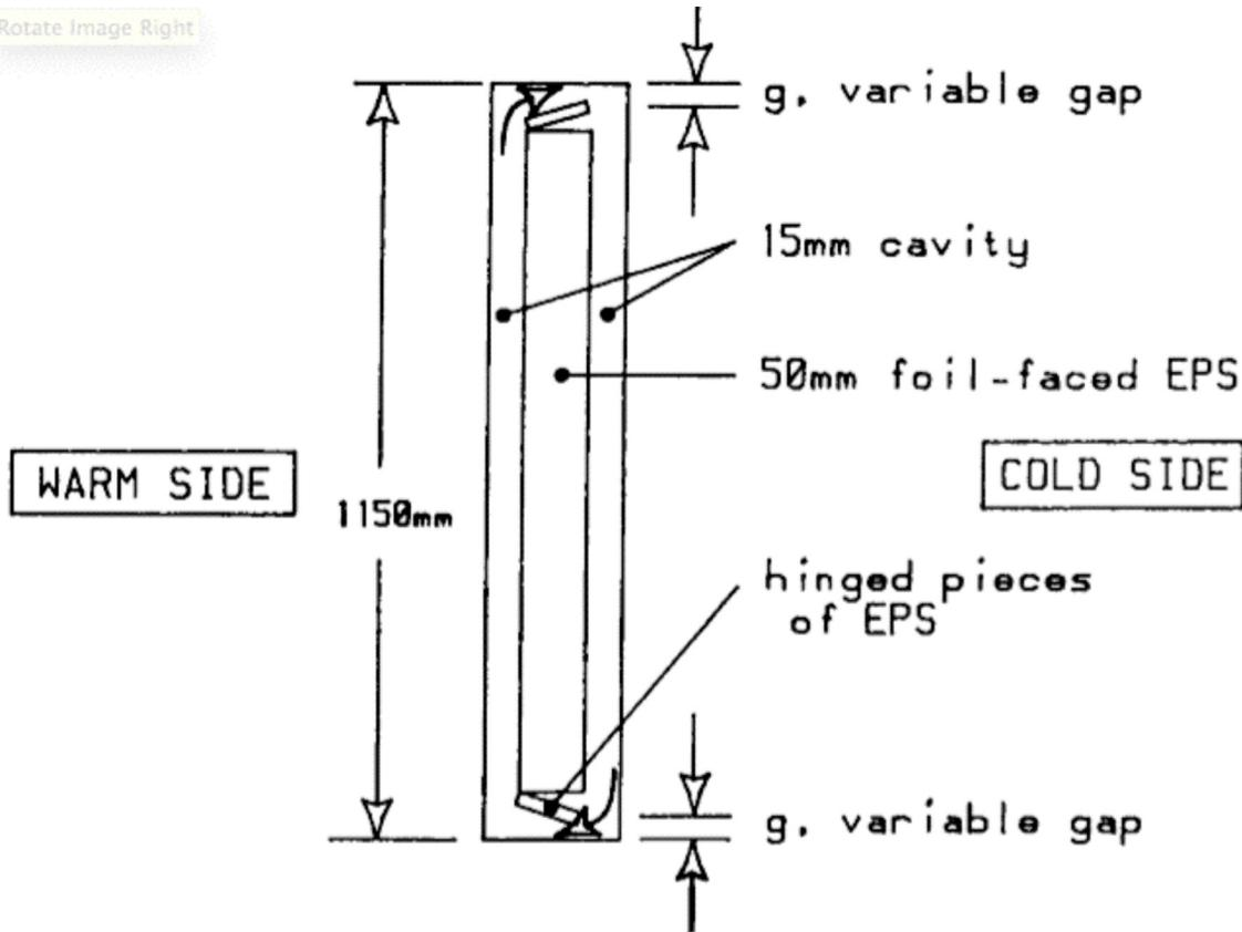
**Figure 14: Experimental Setup to Test Convective Heat Loss around Air Impermeable Insulation (from Trethewen 1991)**
