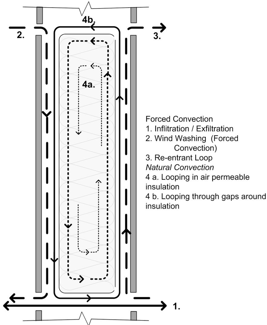
Figure 7: Common Convective Heat Flow Paths in Enclosures
