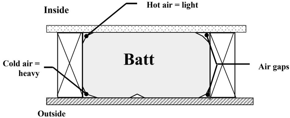
**Figure 9: Gaps that Form at the Corner of improperly-installed Friction-fit Batts can allow Convection Loops to Form**
