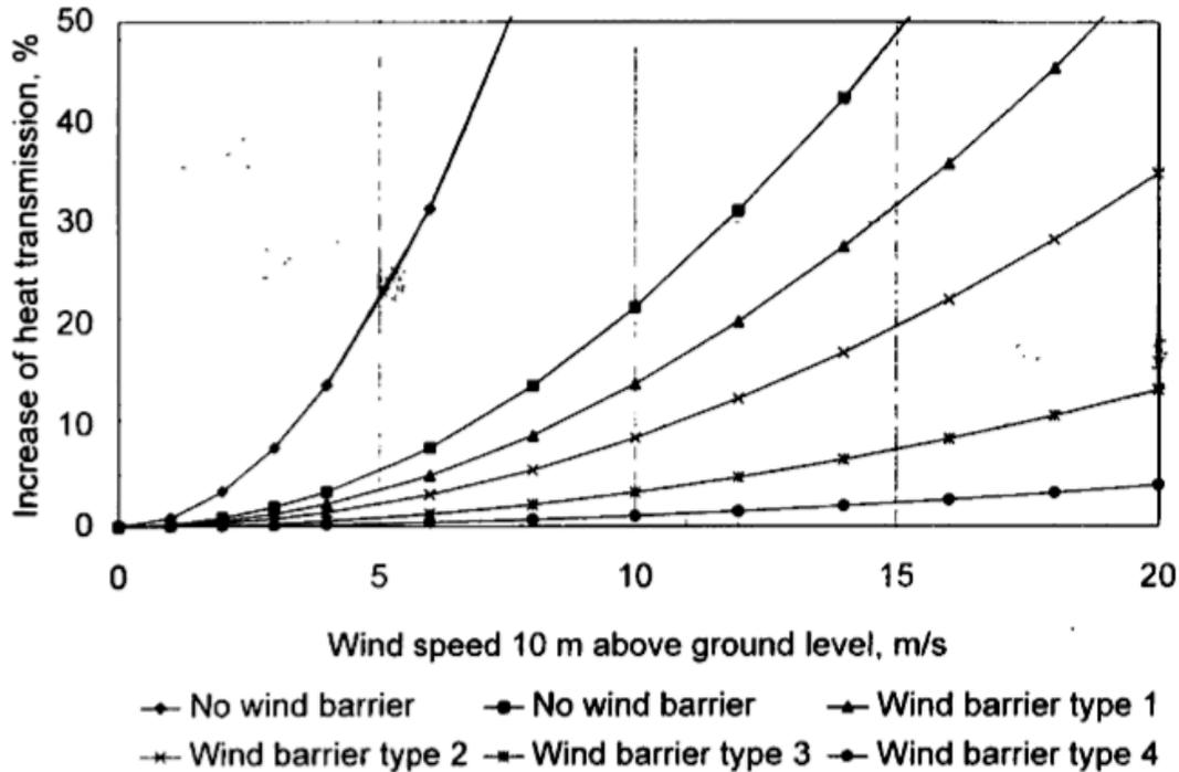
**FIGURE 11.** Estimated increase of heat loss through a timber frame wall, because of forced convection. Construction variant 1. The values are *average values* regarding both the wall area of the house and wind approach angle. The measurements with no wind barrier represent two ways of mounting the thermal insulation into the wall cavity. The permeance for the four wind barriers including joints are 4.9E-5, 1.9E-5, 0.73E-5 and 0.22E-5 m<sup>3</sup>/m<sup>2</sup> s Pa, respectively.
