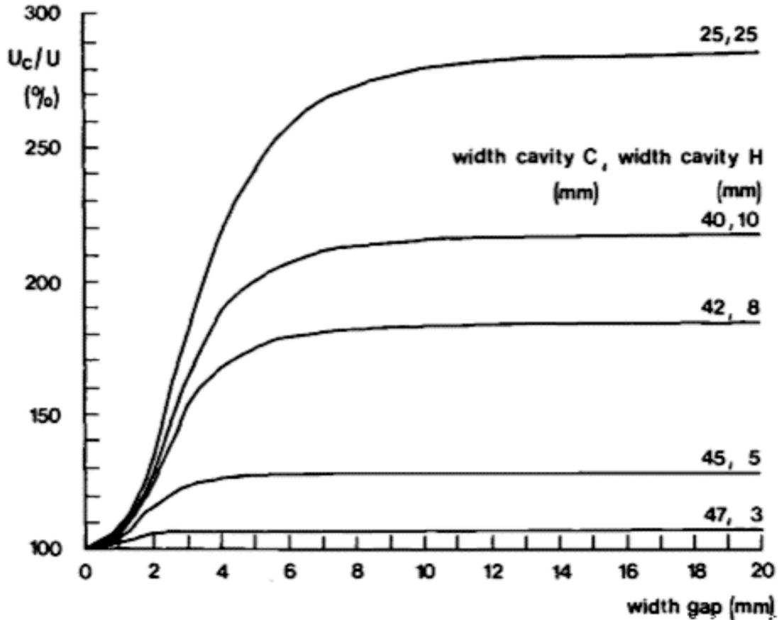
**Figure 13: Increase in U-value (i.e., heat flow) because of convective looping around vertically installed air impermeable insulation as a function of Cold (C) and Hot (H) vertical cavity size and gap width between sheets (from Lecompte 1991).**
