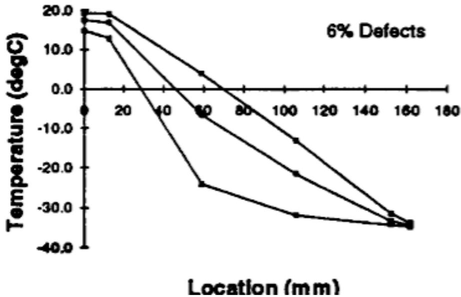
Figure 12: Temperature Plot through Insulated Wall with Defects (from Bomberg et al 1993)
