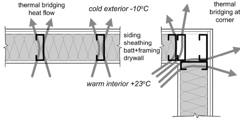
**Figure 2: Thermal Bridging Through Steel Stud Wall**
