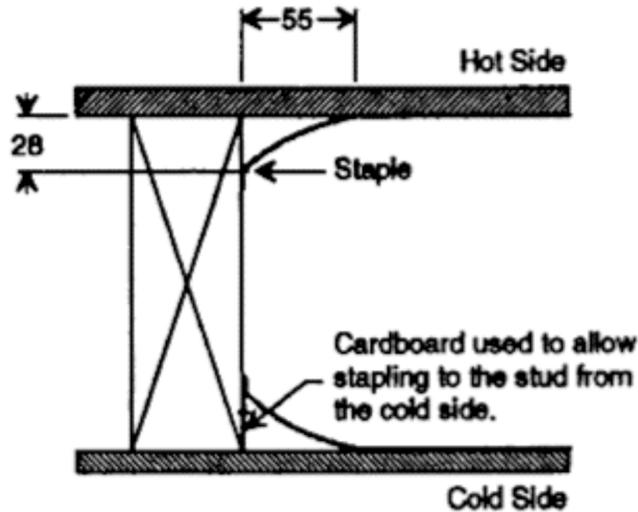
**Figure 10: Experimentally Tested Idealized Gaps in Bomberg & Brown (1993) representing a 6% installation defect (dimensions in mm)**
