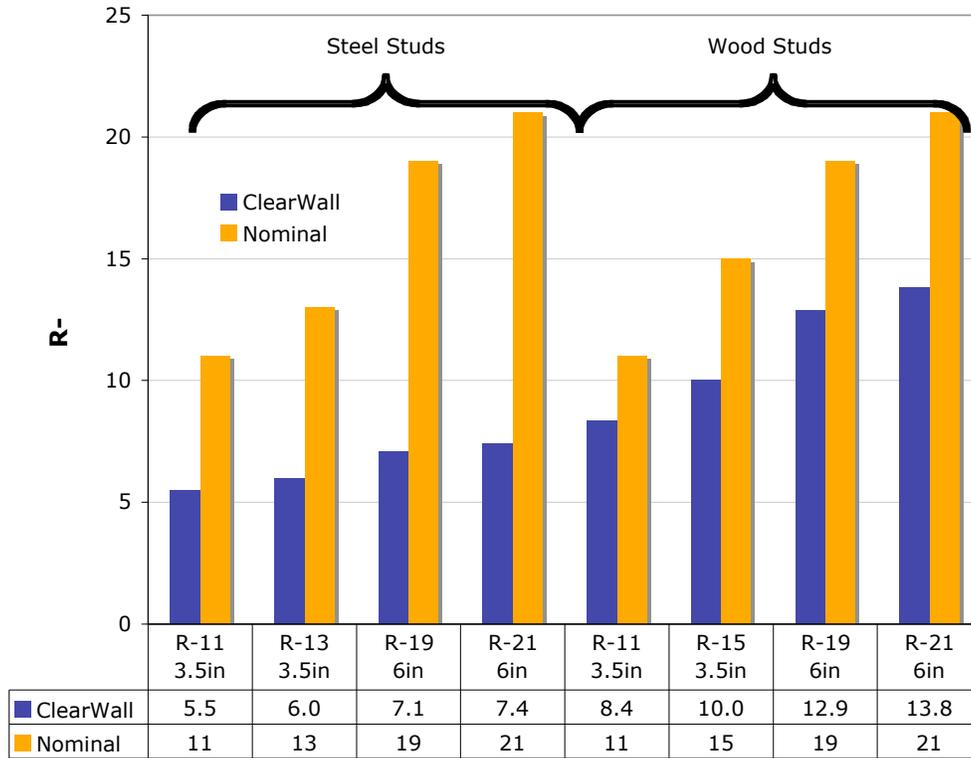
**Figure 3: Nominal and Clear Wall Insulation R-values (after ASHRAE 90.1-1999) for Several Different Stud Materials and Insulation**
