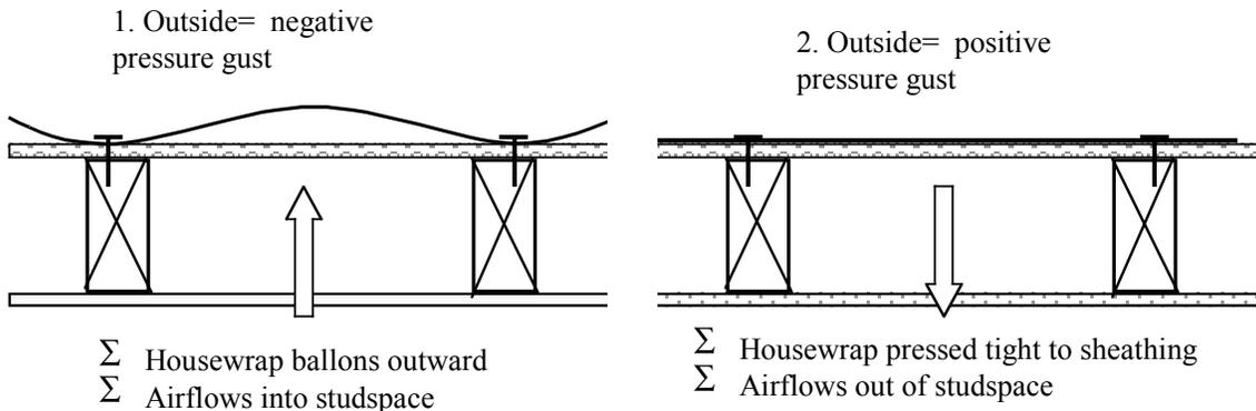
**Figure 16: Loose-applied membranes can pulse and flutter in dynamic wind conditions, thereby causing air “pumping”**
