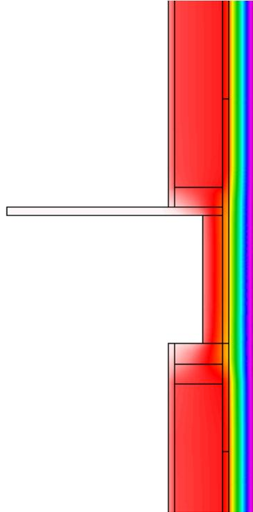
**Figure 33 : Therm modeling of Wall 9 - 2x4 framing with 2" XPS exterior insulation and no stud cavity insulation**
