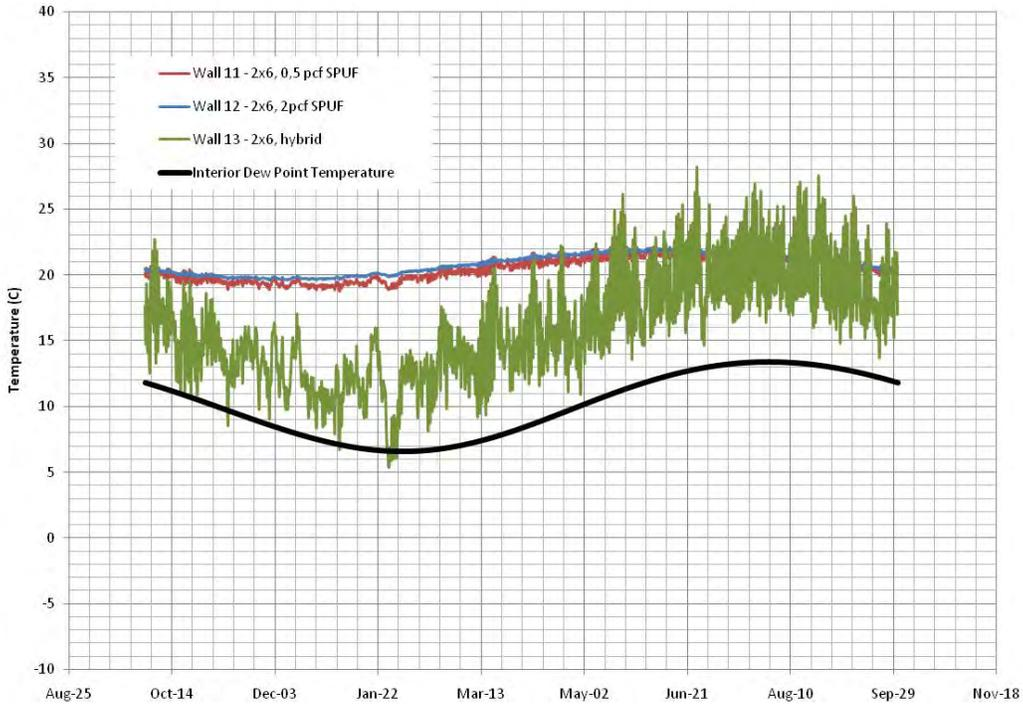
**Figure 14 : Winter air leakage condensation potential for Walls 11, 12, and 13**
