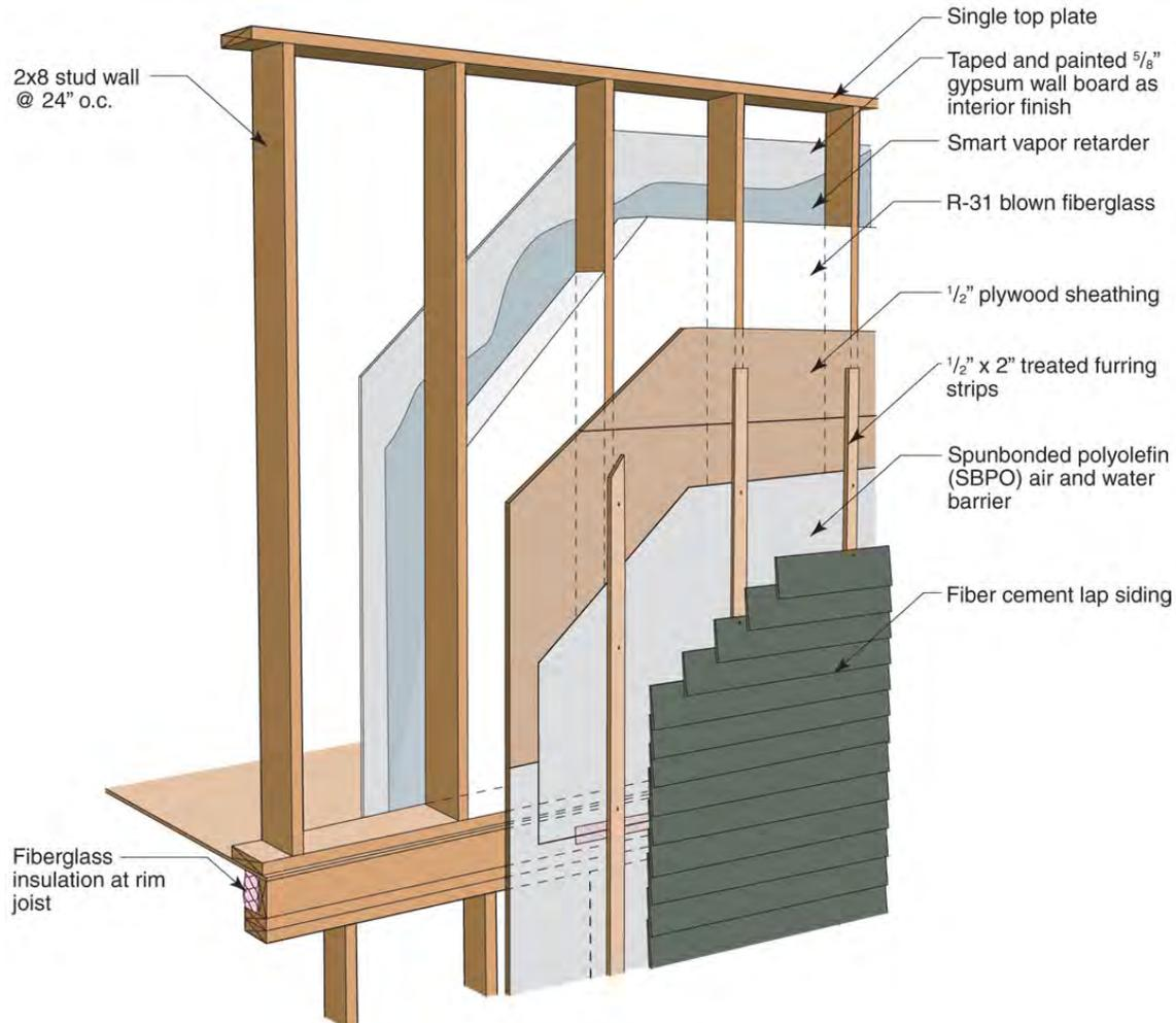
**Figure 28 : 2x8 advanced framing with blown fiberglass insulation**
