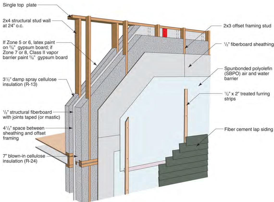
**Figure 44 : Double Stud wall with an interior structural wall**
