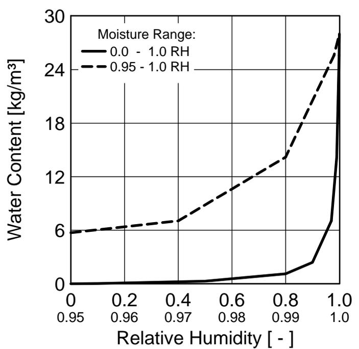
Material : Expanded Polystyrene Insulation (EPS)
