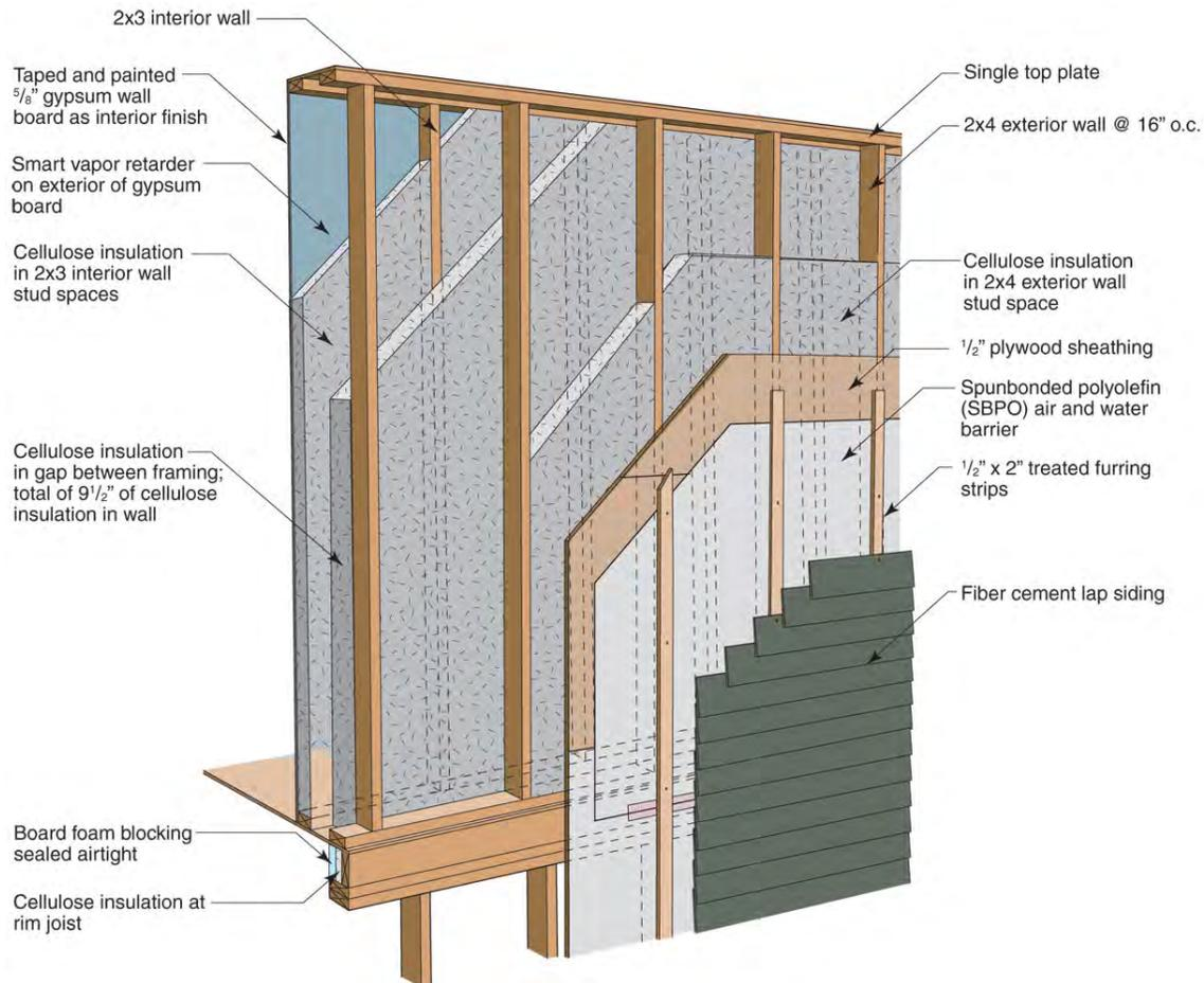
Figure 42 : Double Stud wall with an exterior structural wall
