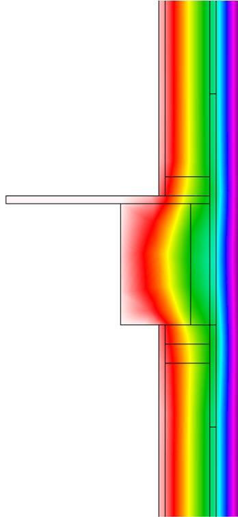
**Figure 35 : Therm modeling of Wall 10 - 2x4 construction with exterior insulation and fiberglass batt**
