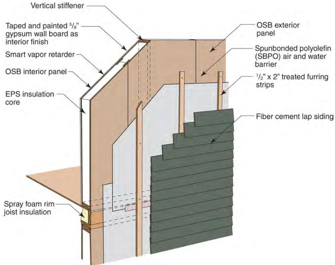
Figure 46 : Wall construction using SIPs
