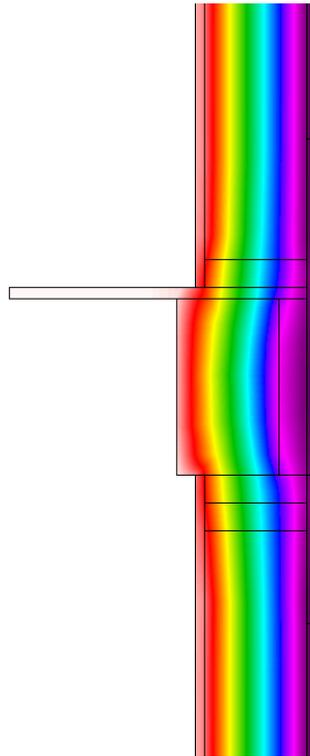
**Figure 23 : Therm modeling of Wall 2 – 2x6 advanced framing with fiberglass batt insulation**
