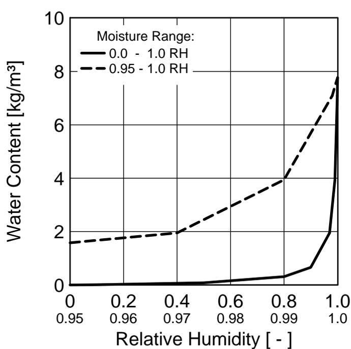
Material : Spun Bonded Polyolefine Membrane (SBP)
