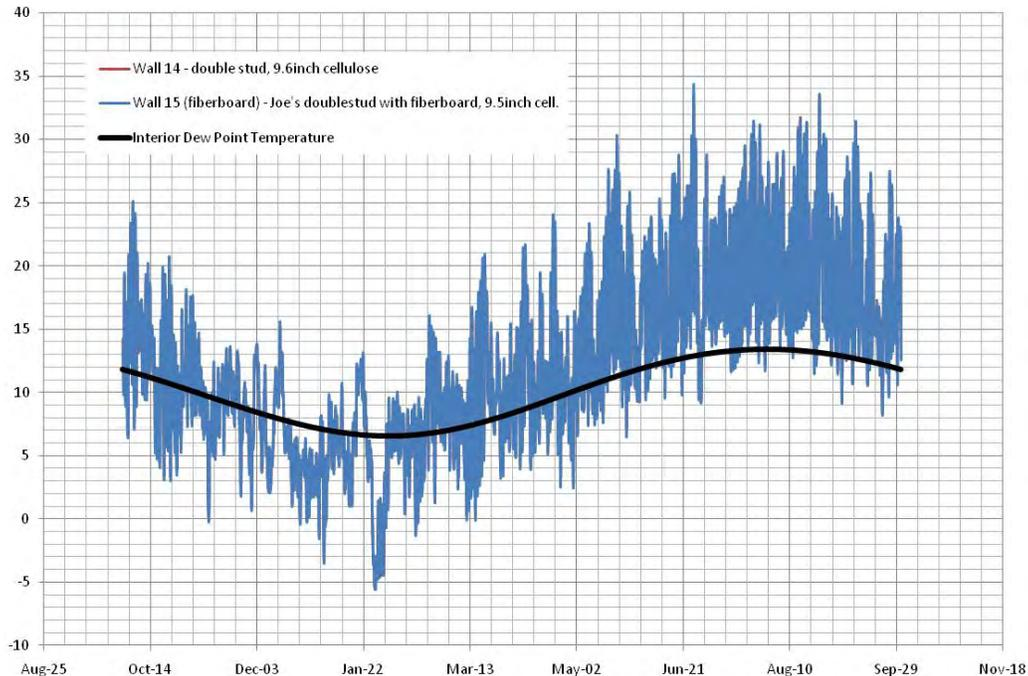
**Figure 16 : Winter air leakage condensation potential for Walls 14 and 15**
