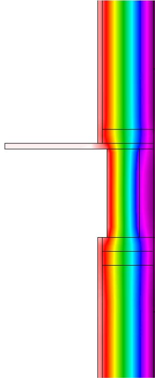
**Figure 37 : Therm analysis of Advanced Framing with 0.5pcf Spray Foam**
