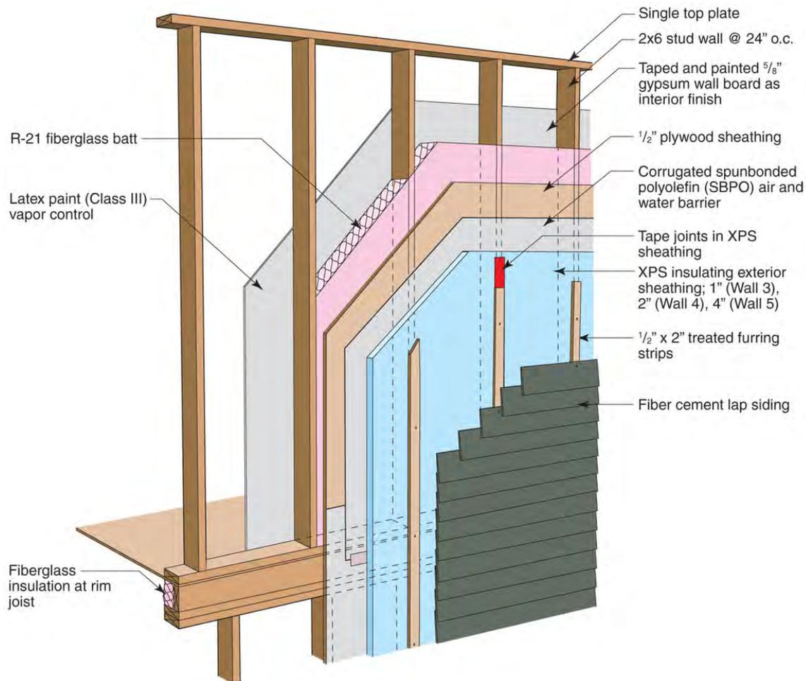
Figure 24 : 2x6 advanced framing construction with exterior XPS insulation
