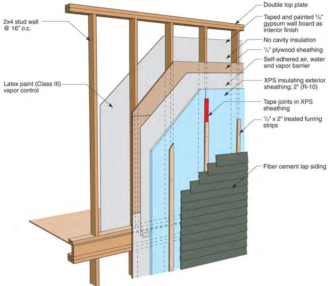
**Figure 32 : 2x4 wall with exterior XPS insulation, without stud cavity insulation**
