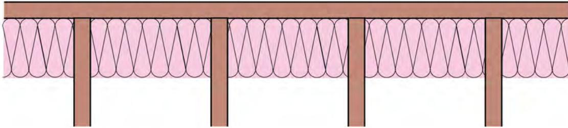
**Figure 3 : Plan section of rim joist, floor joists, and fiberglass batt insulation**
