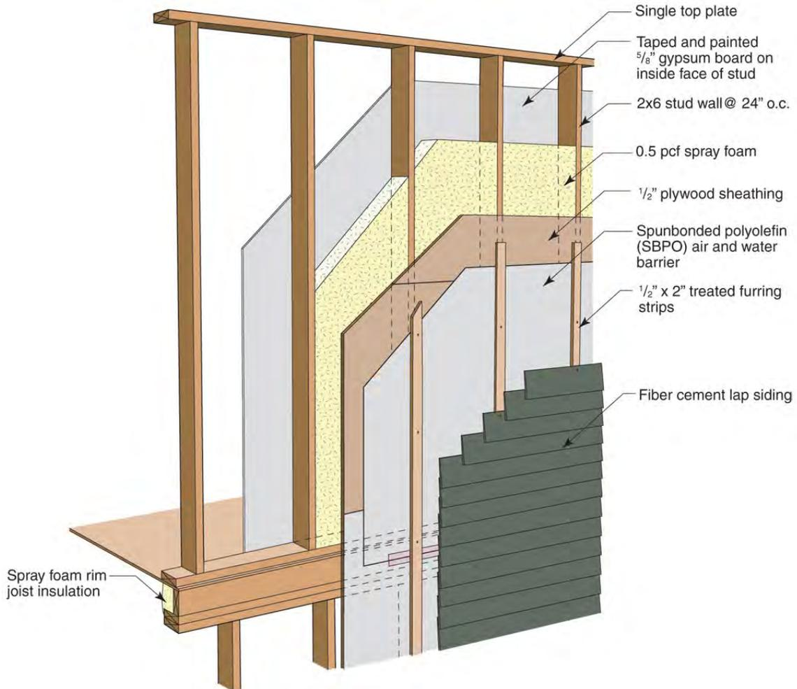
**Figure 36 : 2x6 advanced framing with 0.5pcf Spray Foam**
