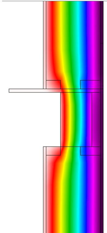
**Figure 43 : Thermal modeling of Wall 14 - Double stud wall with an exterior structural wall**
