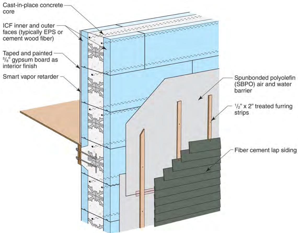
**Figure 47 : Wall construction using ICF**
