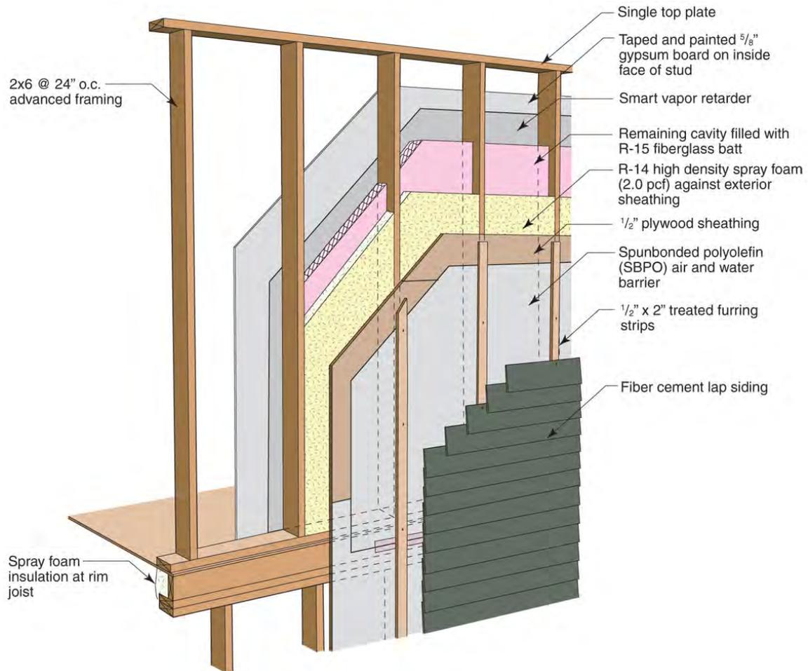
**Figure 40 : Advanced framing with hybrid cavity insulation (Flash and Batt)*****Thermal Control***
