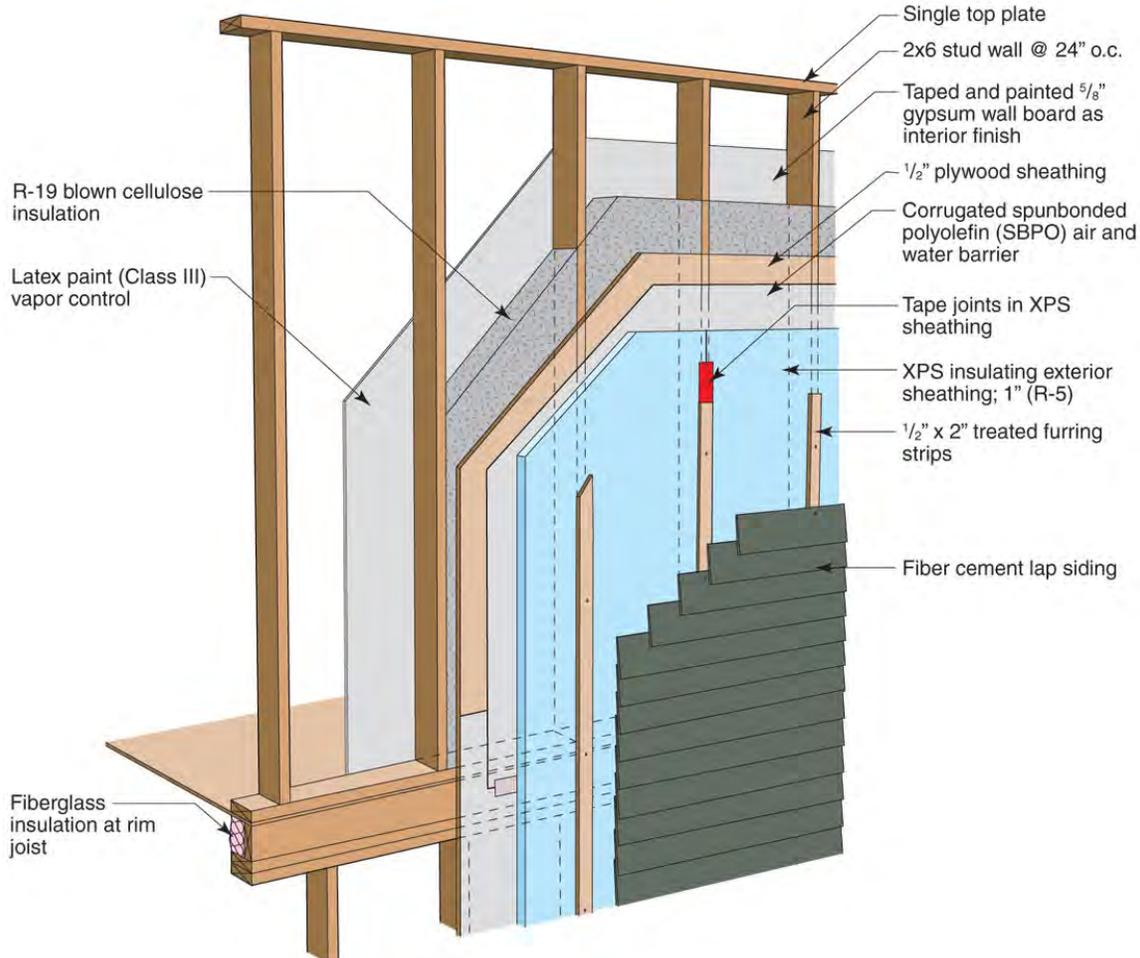
**Figure 26 : Advanced framing with cellulose cavity insulation and 1" of XPS exterior insulation**
