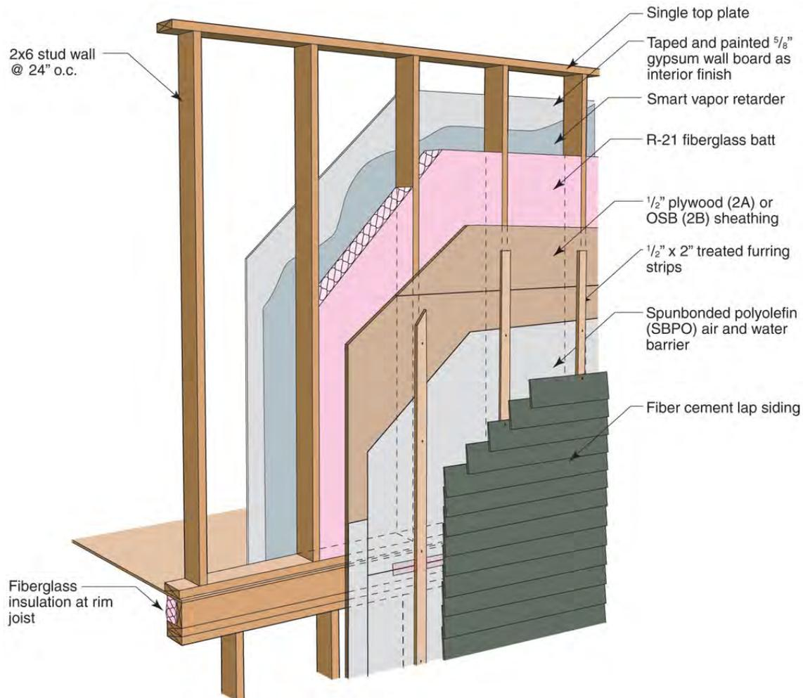
Figure 22 : 2x6 advanced framing construction
