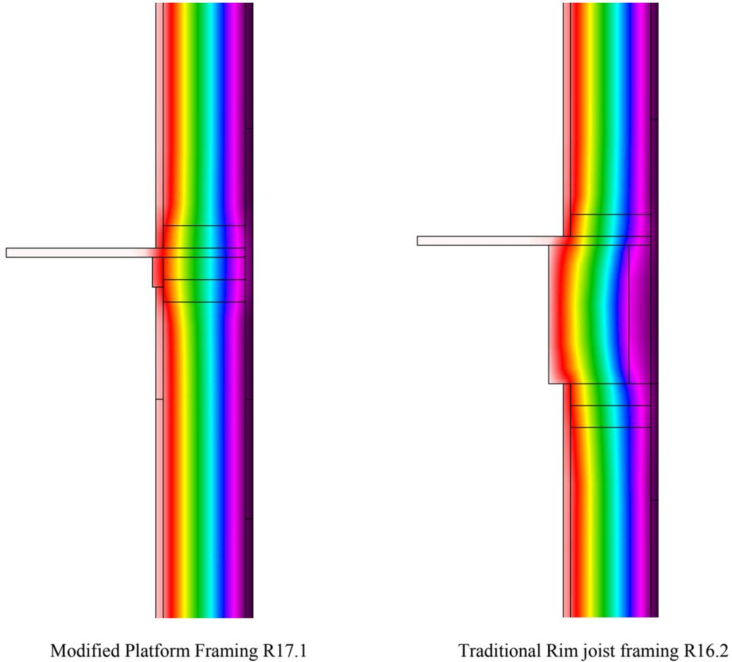
**Figure 4 : Thermal Performance Comparison Between Tradition Rim Joist Framing and Modified Platform Framing**
