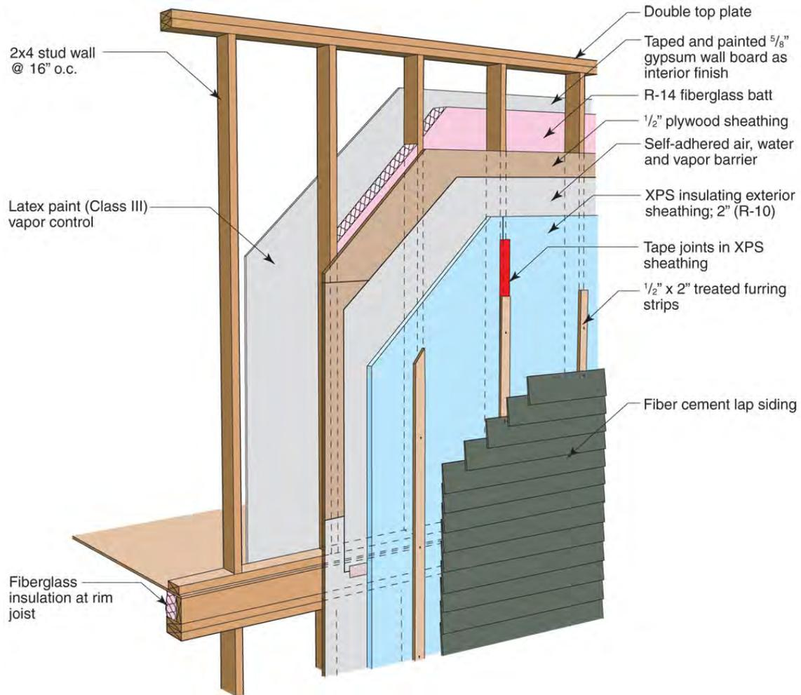
**Figure 34 : 2x4 wall construction with XPS insulation and fiberglass batt**
