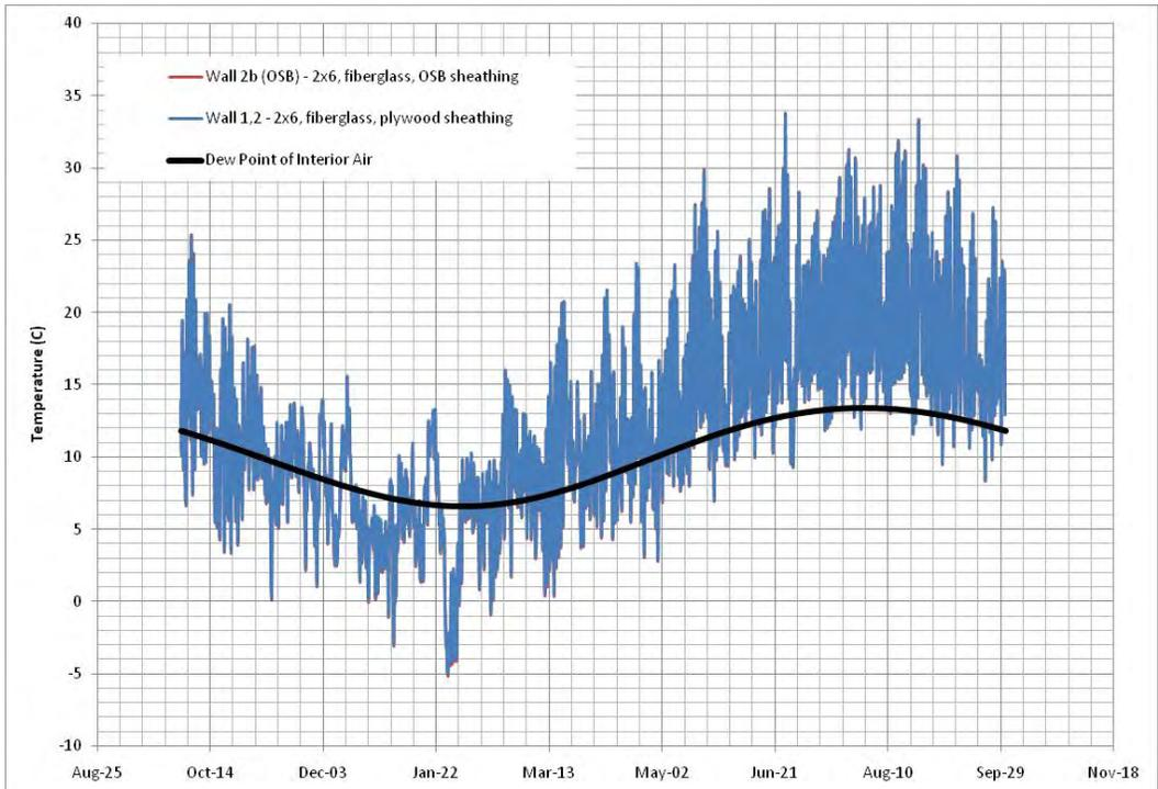
**Figure 10 : Winter air leakage condensation potential for Wall 1 and Wall 2**
