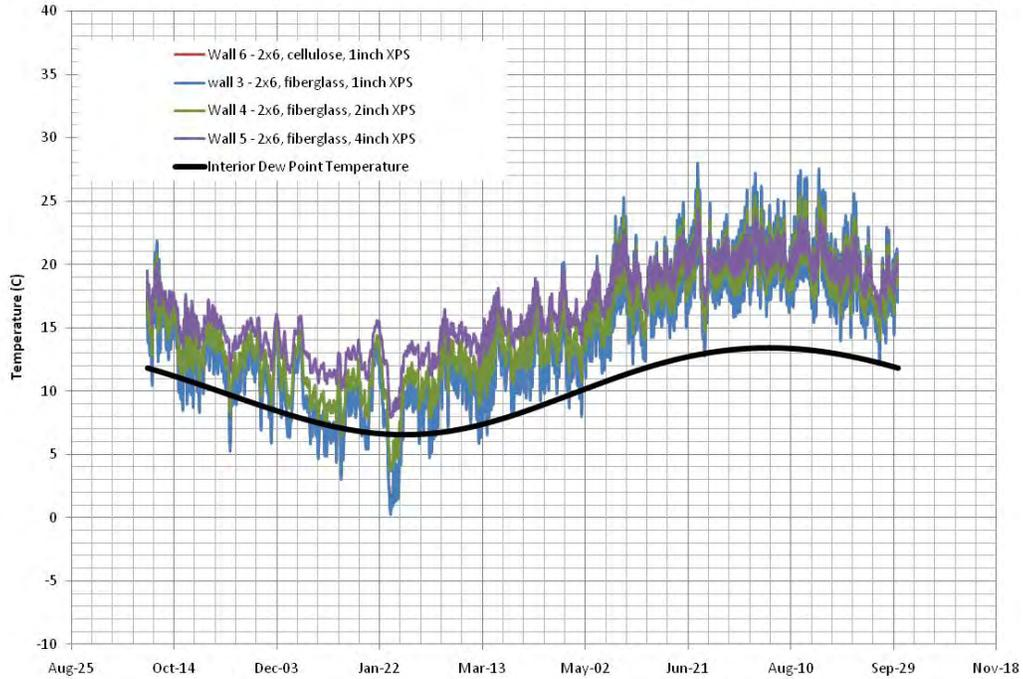
**Figure 11 : Winter air leakage condensation potential for Walls 3, 4, 5, and 6**
