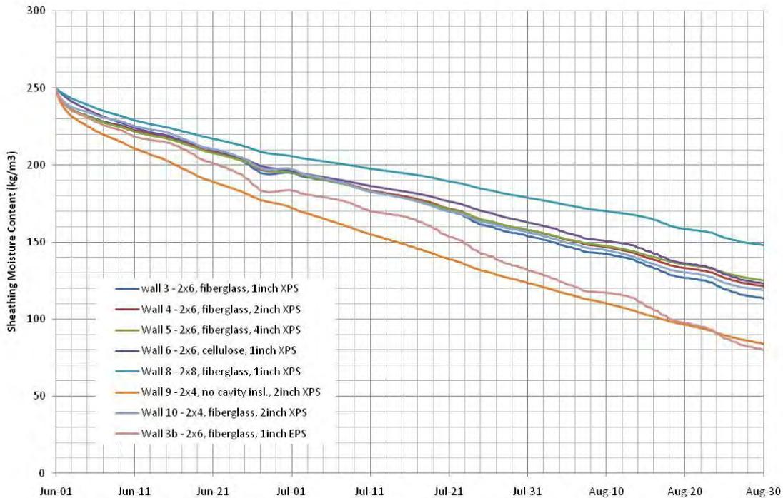
**Figure 19 : Analysis of Drying Curves of Walls With Exterior Insulation**
