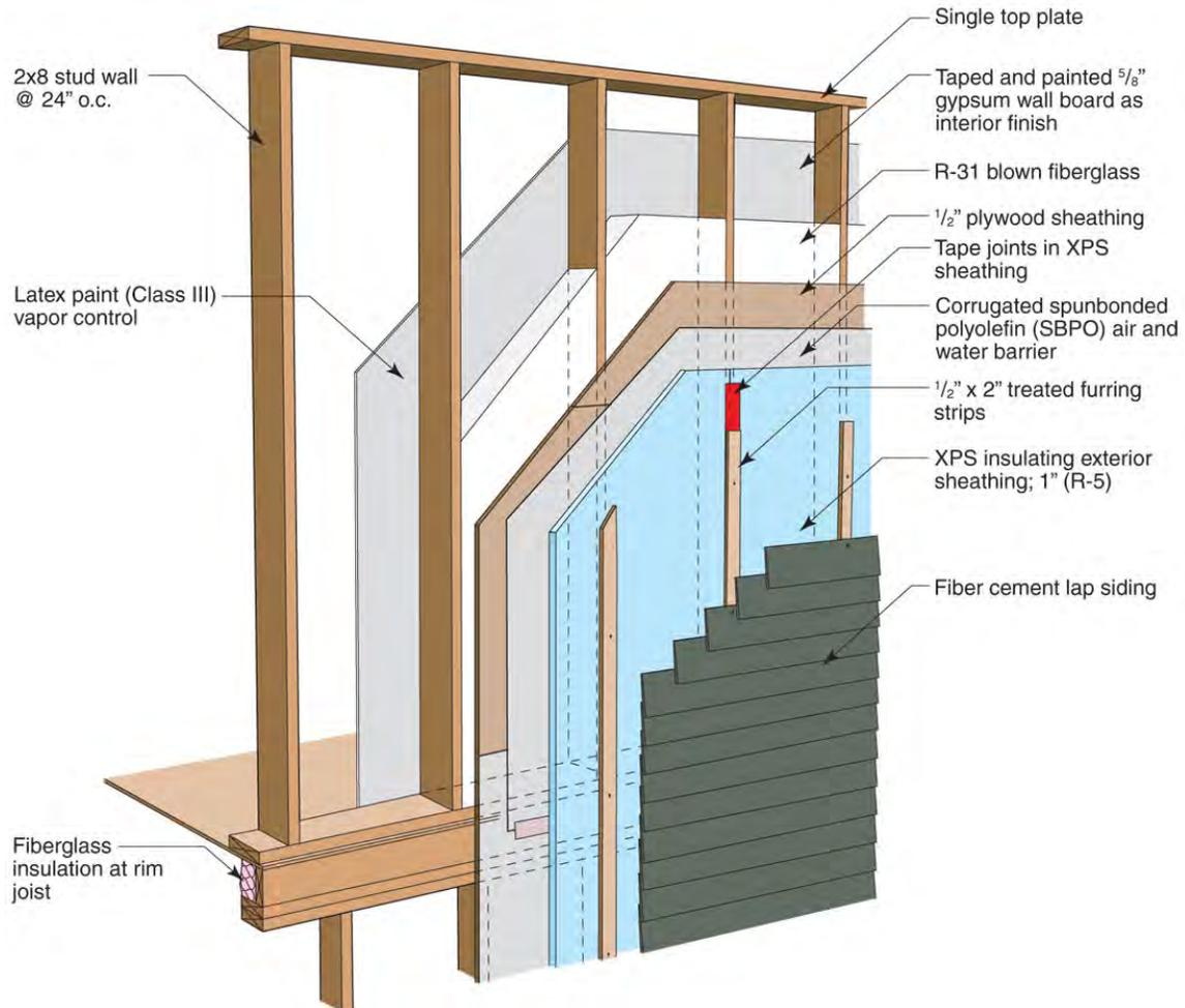
Figure 30 : 2x8 advanced framing with blown fiberglass cavity insulation and exterior insulation
