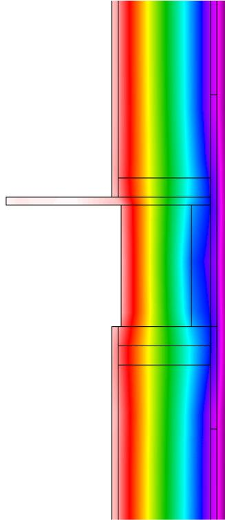
**Figure 31 : Therm modeling of Wall 8 - 2x8 advanced framing with blown fiberglass cavity insulation and exterior insulation**
