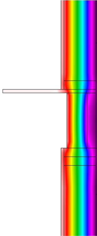
**Figure 39 : Therm modeling of Wall 12 - Advanced framing with 2.0pcf Spray Foam**
