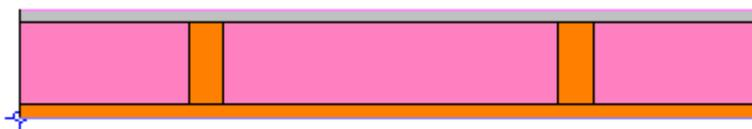
**Figure 6 : Typical framing 16" o.c. - 9% framing factor**
