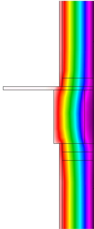
**Figure 21 : Therm modeling of Wall 1 – Standard 2x6 construction**
