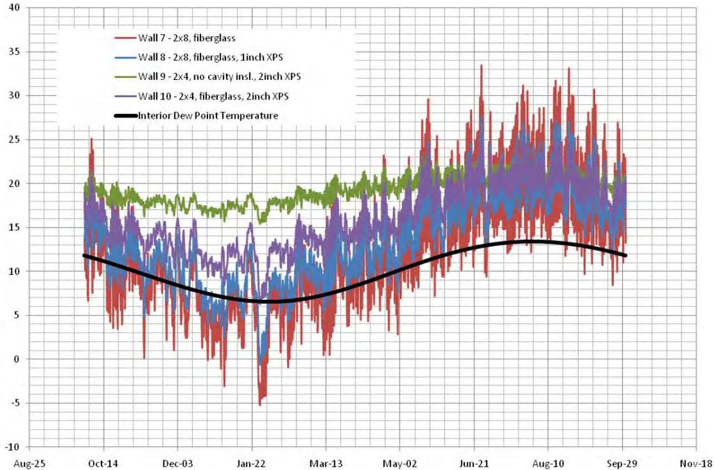
**Figure 13 : Winter air leakage condensation potential for Walls 7 to 10.**
