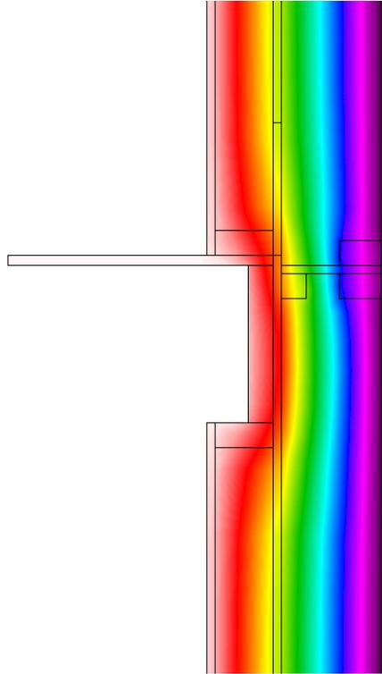
**Figure 45 : Thermal modeling of Wall 15 - Double stud wall system with an interior structural wall**
