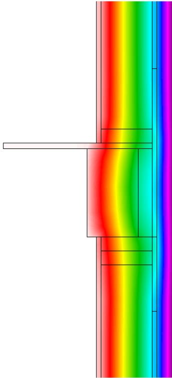
**Figure 25 : Therm modeling of advanced framing with fiberglass cavity insulation and 2” XPS exterior insulation**
