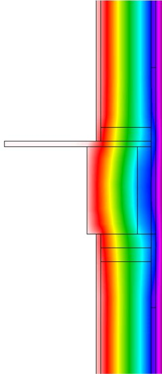
**Figure 27 : Therm modeling of Wall 6 - of an advanced framing with cellulose cavity insulation and 1" XPS exterior insulation**
