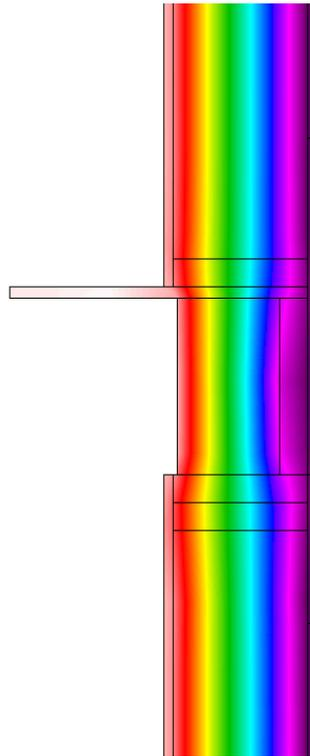
**Figure 29 : Therm modeling of Wall 7 - of the 2x8 advanced framing with blown fiberglass**
