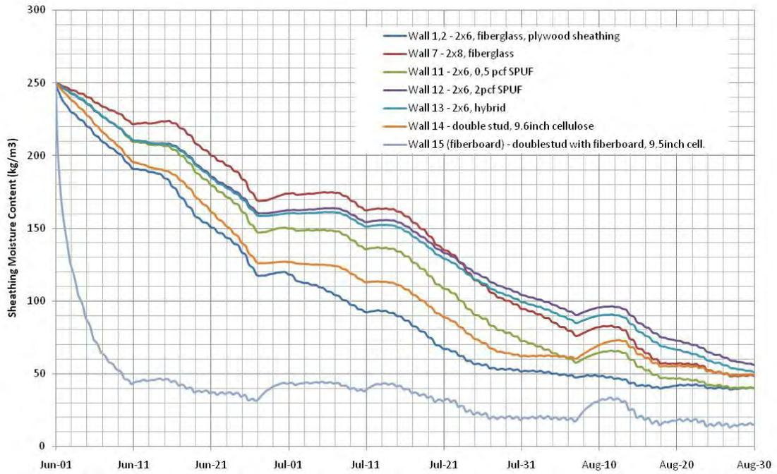
**Figure 18 : Analysis of Drying Curves of Walls without Exterior Insulation**
