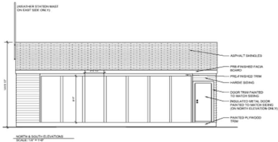
**Figure 2 : Elevation drawing of Coquitlam test hut**
