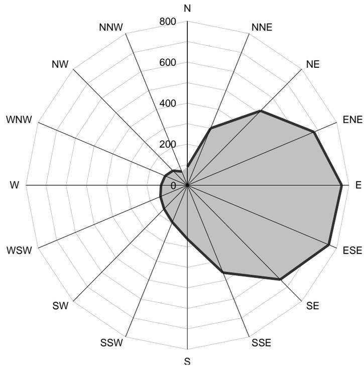
**Figure 11 : Vancouver, BC driving rain rose**
