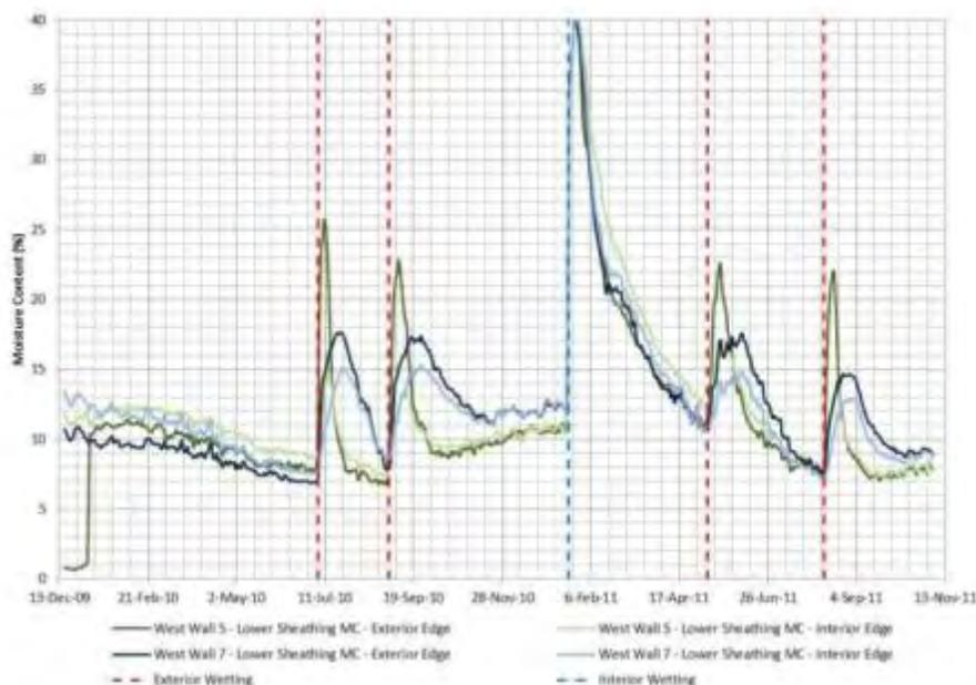
**Figure 17 : Lower OSB sheathing measured moisture content comparison between West Wall 5 (ventilated stucco) and West Wall 7 (exterior insulation)**
