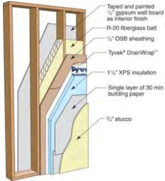
**Figure 14 : Construction of Wall 7 on all four orientations**
