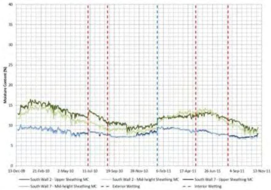
**Figure 26 : South Wall 2 (direct applied stucco), and South Wall 7 (exterior insulation) middle and upper OSB sheathing measured moisture content**
