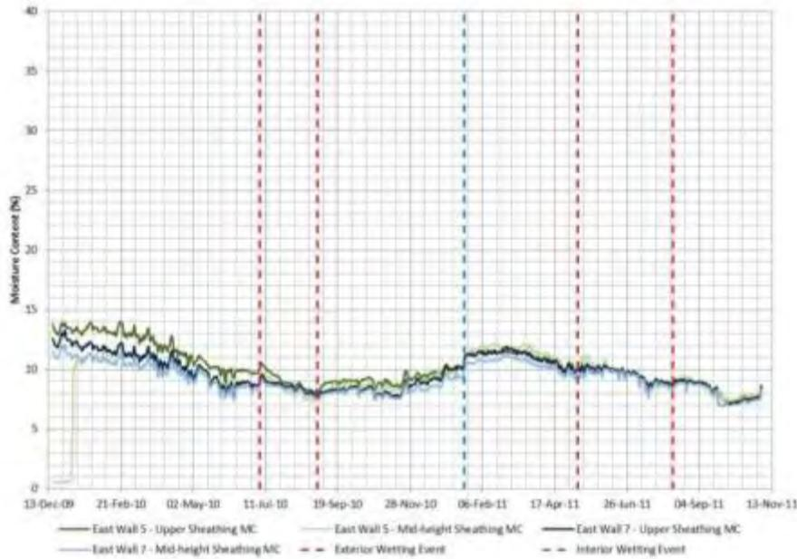
**Figure 20 : Middle and upper OSB sheathing measured moisture content comparison between East Wall 5 (ventilated stucco) and East Wall 7 (exterior insulation)**
