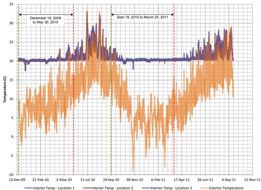
**Figure 30 : Measured interior and ambient temperatures**
