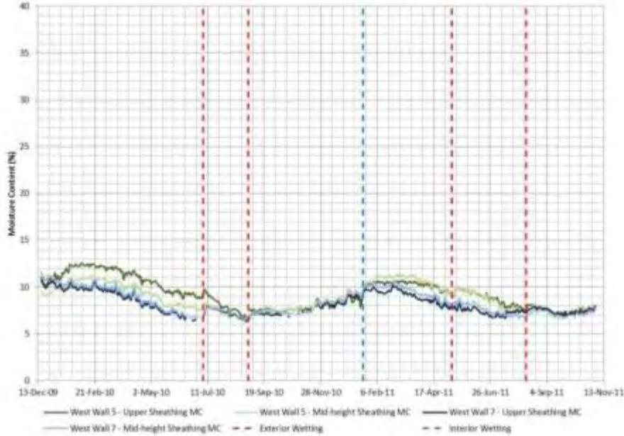
**Figure 18 : Middle and upper OSB sheathing measured moisture content comparison between West Wall 5 (ventilated stucco), and West Wall 7 (exterior insulation)**
