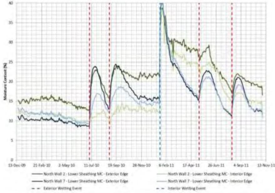
**Figure 21 : Lower OSB sheathing measured moisture content comparison between North Wall 2 (direct applied stucco) and North Wall 7 (exterior insulation)**
