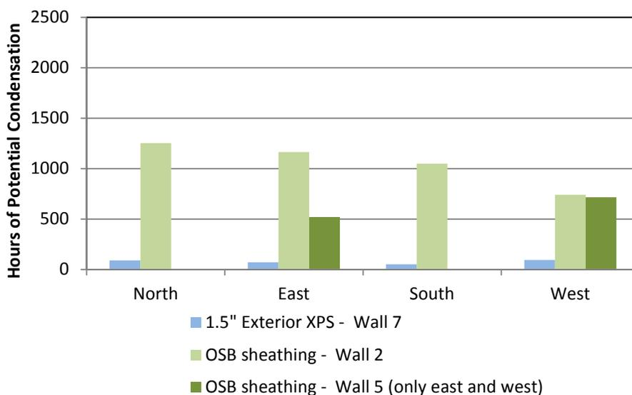
**Figure 32 : Comparison of the hours of potential condensation between Wall 2 and Wall 7 from December 18, 2009 to May 30, 2010 using measured interior dew point and sheathing temperature**
