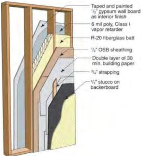
**Figure 15 : Wall 5 on the East and West orientation**
