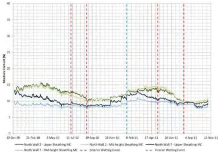
**Figure 22 : Middle and upper OSB sheathing measured moisture content comparison between North Wall 2 (direct applied stucco), and North Wall 7 (exterior insulation)**
