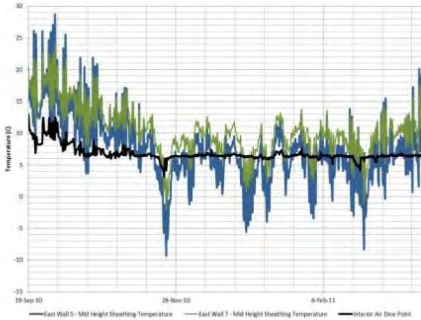
Figure 35 : Comparison of condensation potential between East Walls 5 and 7, Sept to March 2010
