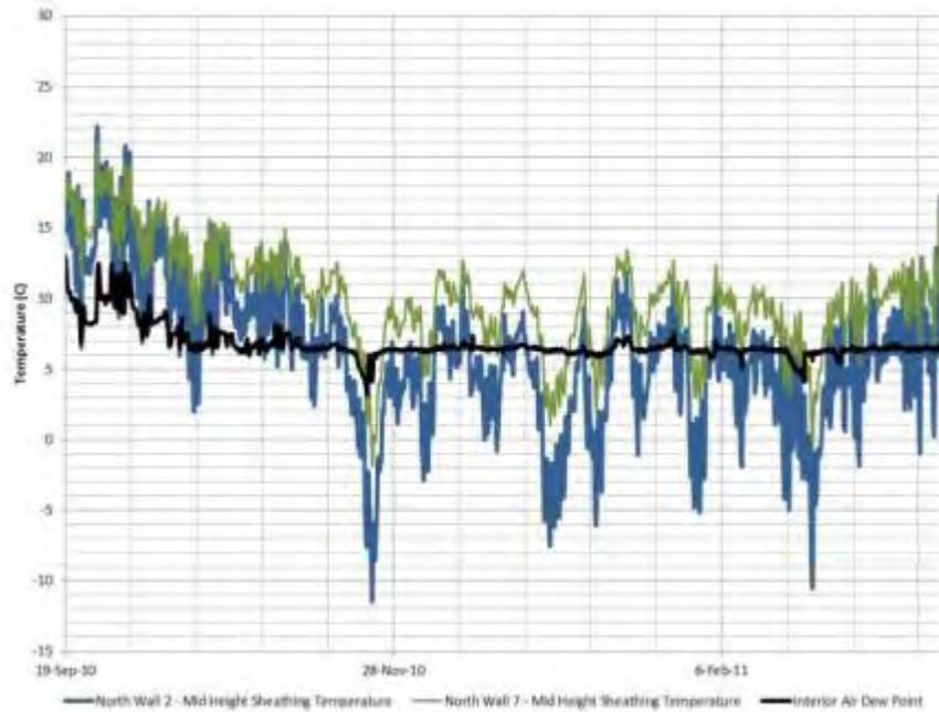
Figure 37 : Comparison of condensation potential between North Walls 2 and 7, Sept to March 2010
