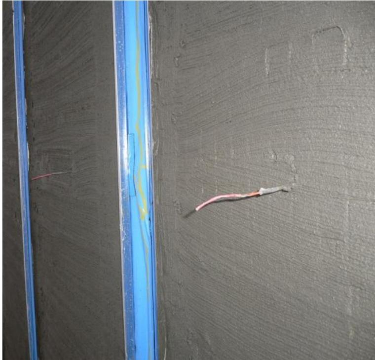
**Figure 18 - Stucco Base Coat and Mid-Height T Sensor**
