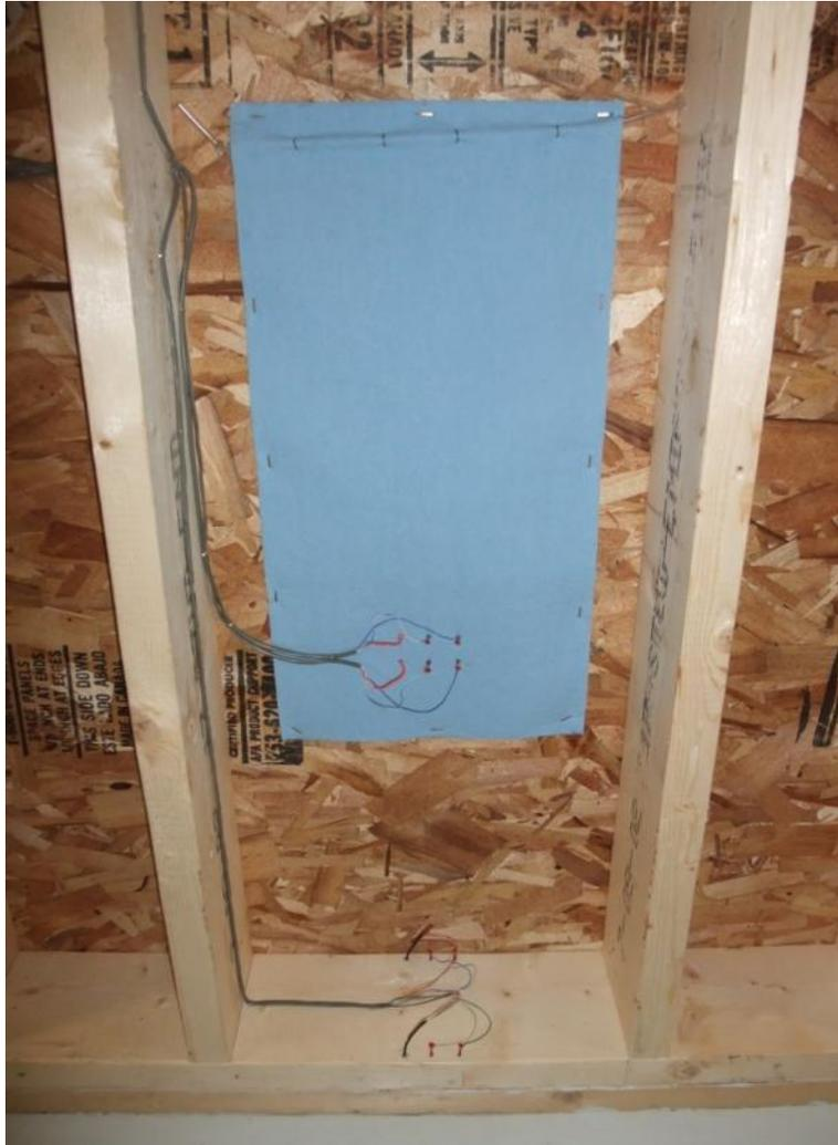
Figure 15 - Interior Wetting Apparatus
