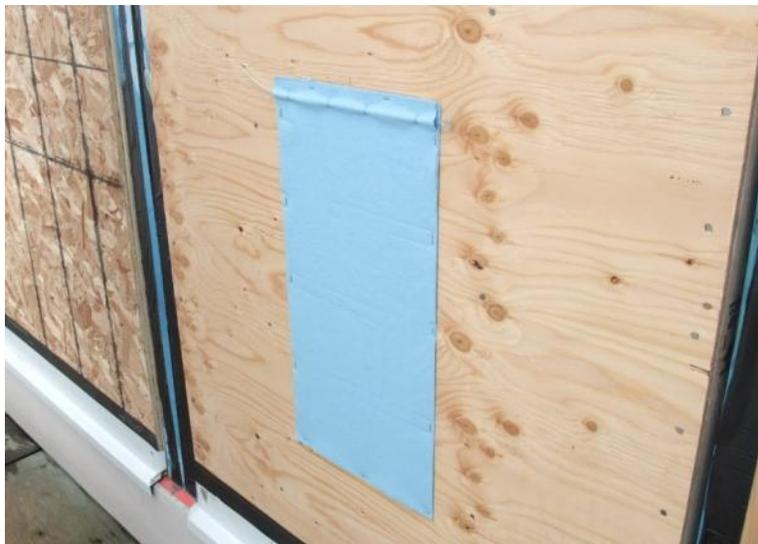
**Figure 14 - Exterior Wetting Apparatus**
