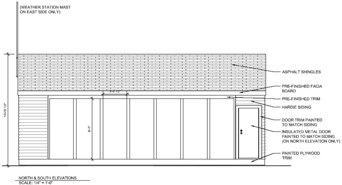
**Figure 3 - North & South Elevation**
