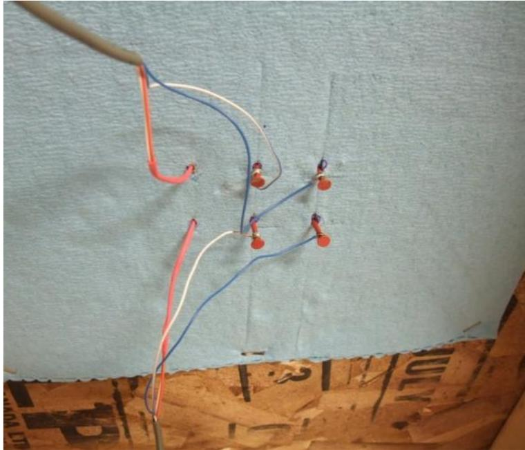
**Figure 6 - Interior and Exterior Sheathing MC/T Sensors**
