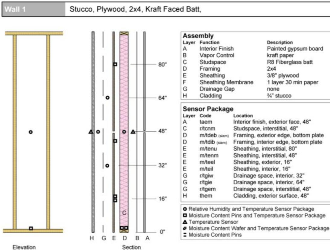
Figure 5 - Typical Instrumentation Package
