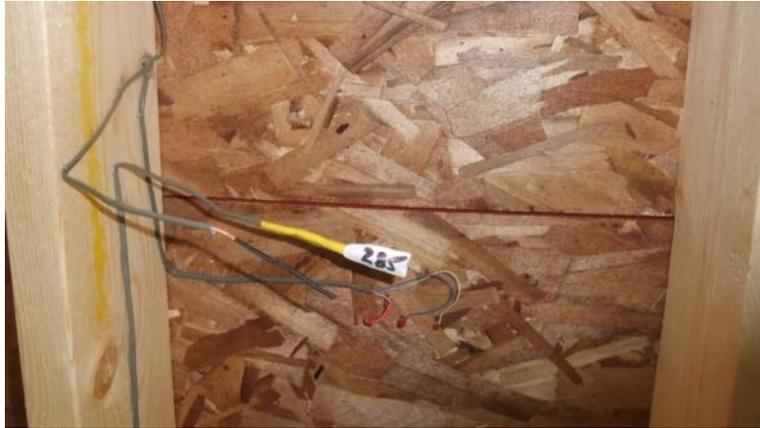
**Figure 8 - Interior Mid-Height T, T/RH and MC/T sensors**
