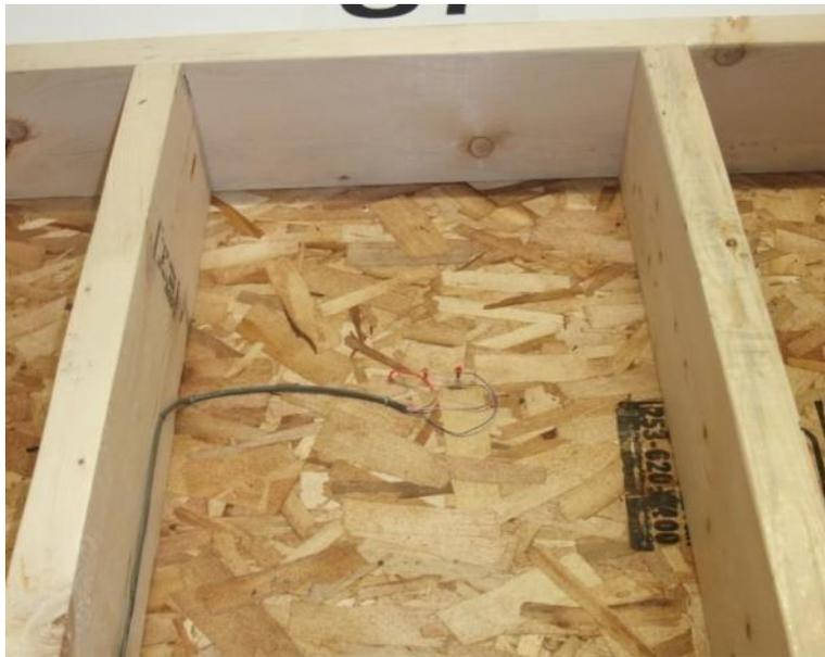
**Figure 7 - Upper Interior Sheathing MC/T Sensors**
