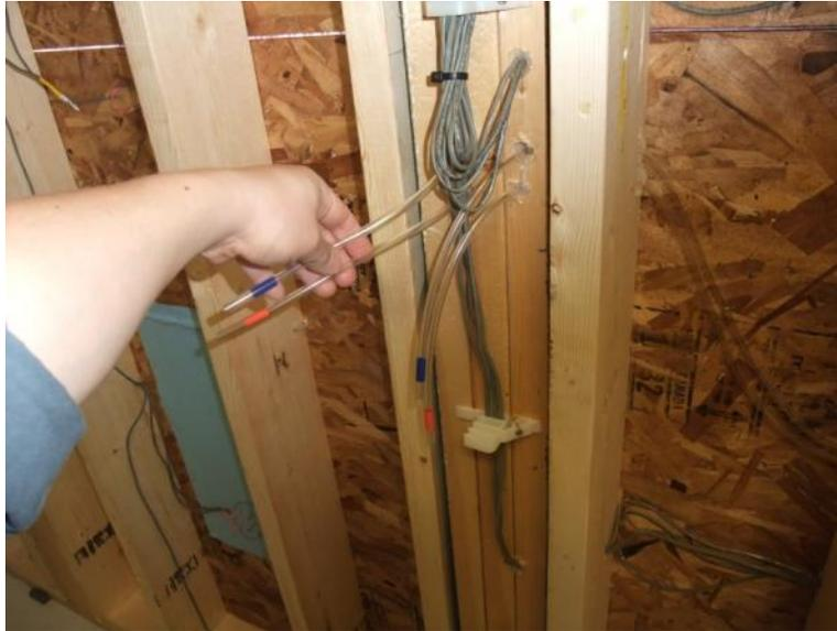
**Figure 16 - Wetting Apparatus Injection Tubes**
