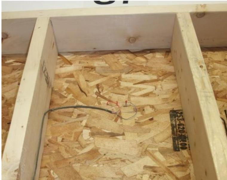
**Figure 15 - Upper Interior Sheathing MC/T Sensors**
