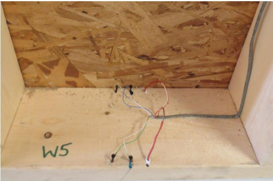
Figure 17 - Bottom Plate MC/T Sensors
