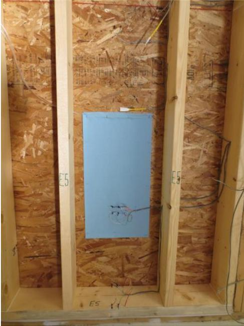
Figure 21 - Interior Wetting Apparatus
