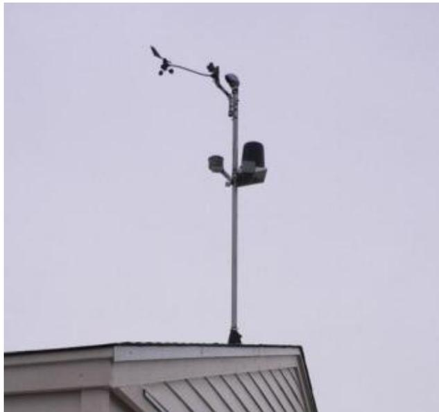
**Figure 5 : Weather station on the roof of the Coquitlam Test Hut**
