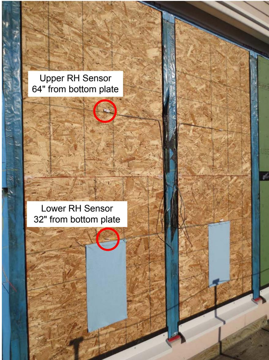
**Figure 18 - Exterior Upper and Lower T/RH Sensors**
