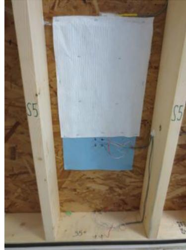
**Figure 9 : South Wall 5 – Interior Wetting system protected from spray foam**
