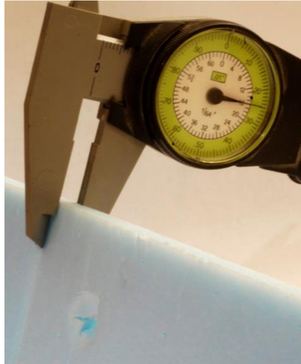
Figure 17 : Measured gap at permanently compressed portion of Dow HPU Layflat Insulation
