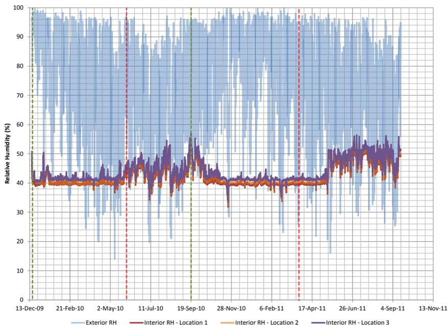
**Figure 31 : Measured interior and ambient relative humidity**
