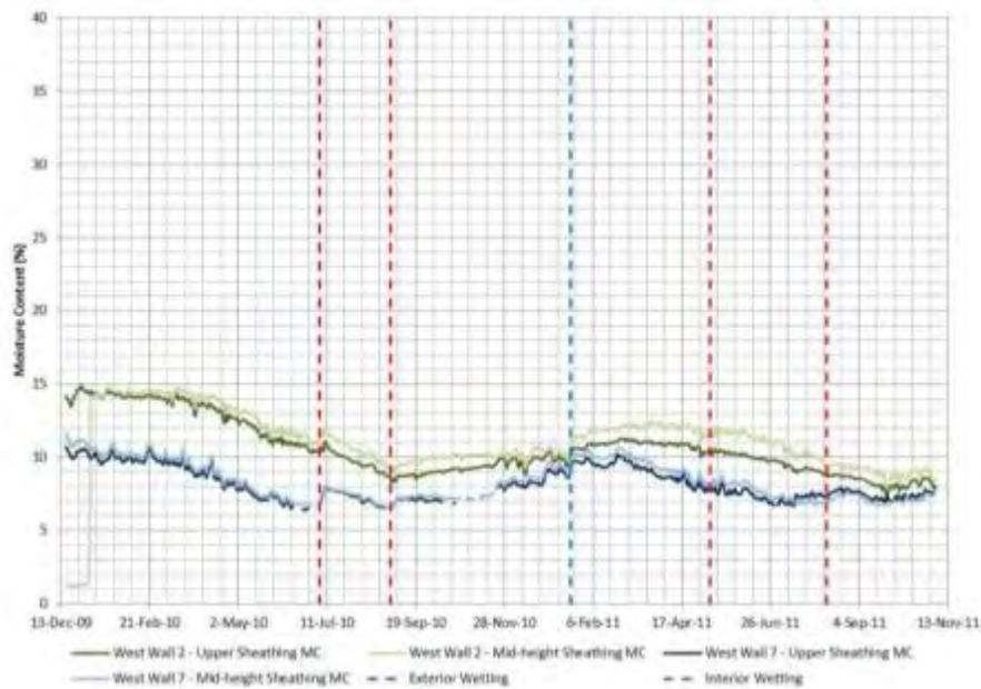
**Figure 28 : West Wall 2 and West Wall 7 Middle and upper OSB sheathing measured moisture content comparing exterior insulation**
