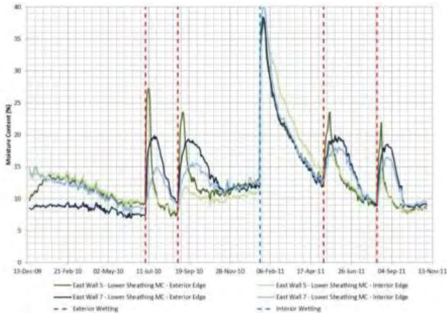
**Figure 19 : Lower OSB sheathing measured moisture content comparison between East Wall 5 (ventilated stucco) and East Wall 7 (exterior insulation)**
