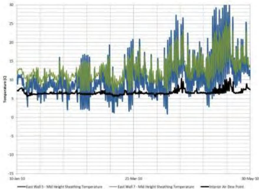
**Figure 34 : Comparison of condensation potential between East Walls 5 and 7, Jan to May 2010**
