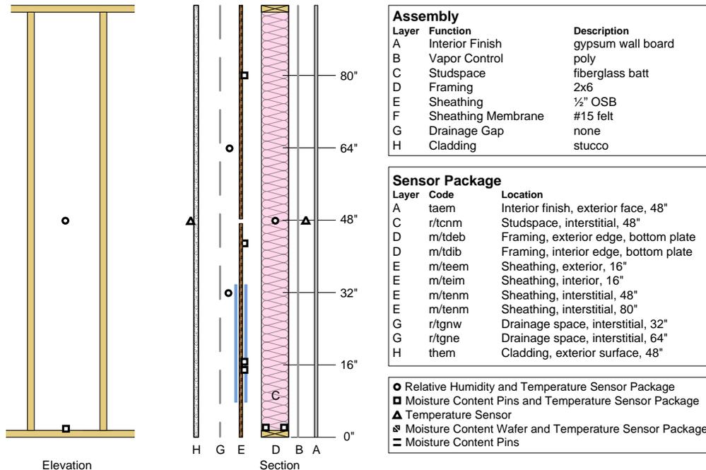
Figure 5 : Typical Wall Construction and Sensor Configuration
