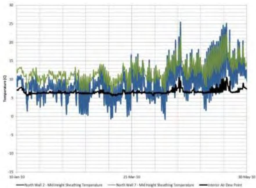
Figure 36 : Comparison of condensation potential between North Walls 2 and 7, Jan to May 2010
