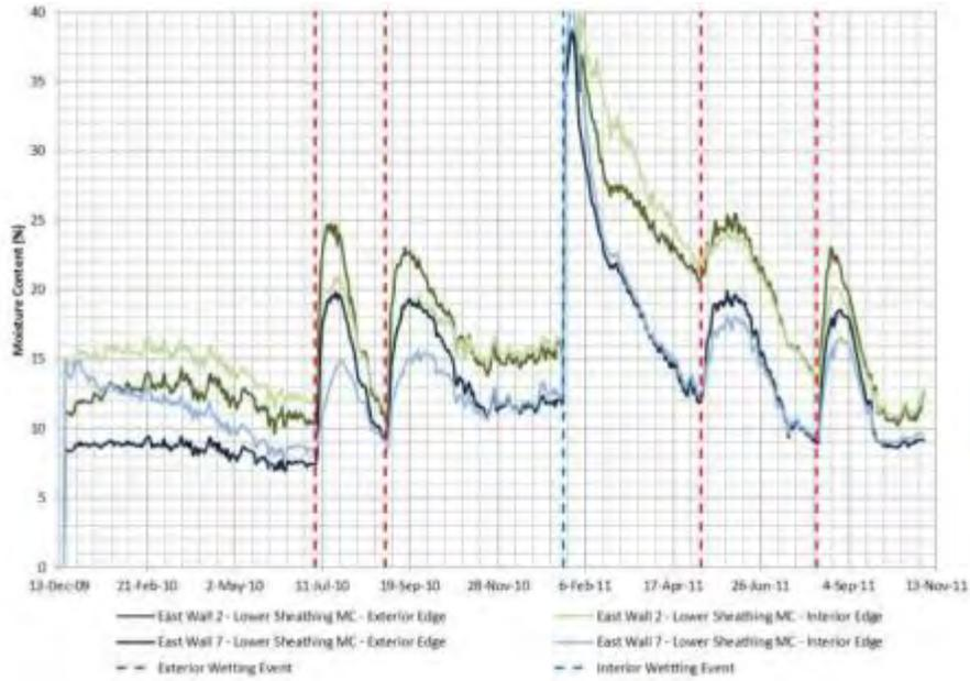
**Figure 23 : East Wall 2 (direct applied stucco) and East Wall 7 (insulating sheathing) lower OSB sheathing measured moisture content**
