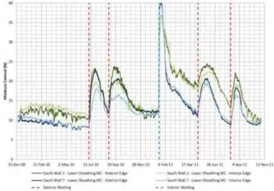
**Figure 25 : South Wall 2 (direct applied stucco) and South Wall 7 (exterior insulation) lower OSB sheathing measured moisture content**
