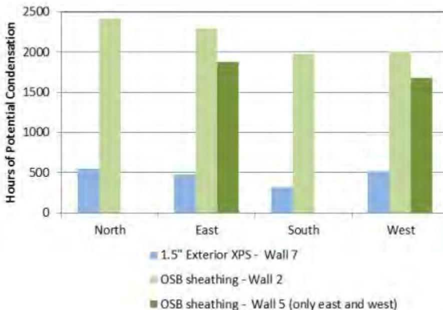
**Figure 33 : Comparison of the hours of potential condensation between Wall 2 and Wall 7 from September 19, 2010 to March 23, 2011 using measured interior dew point and sheathing temperature**
