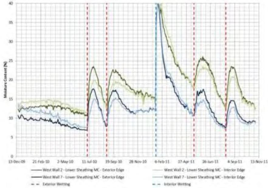
**Figure 27 : West Wall 2 and West Wall 7 Lower OSB sheathing measured moisture content comparing exterior insulation**
