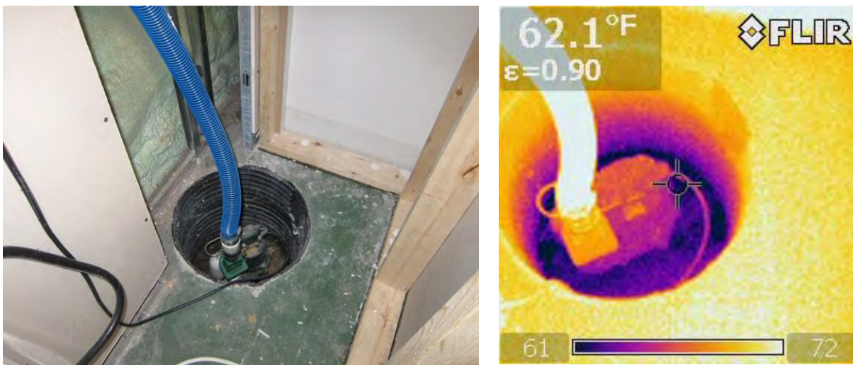
Figure 56. Sump pit temperatures, Concord House
