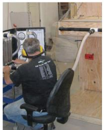
Photograph 3: Skunk Works Air Leakage Testing— Applying air pressure and measuring flow. There's nothing magical here. But, the results are impressive.
